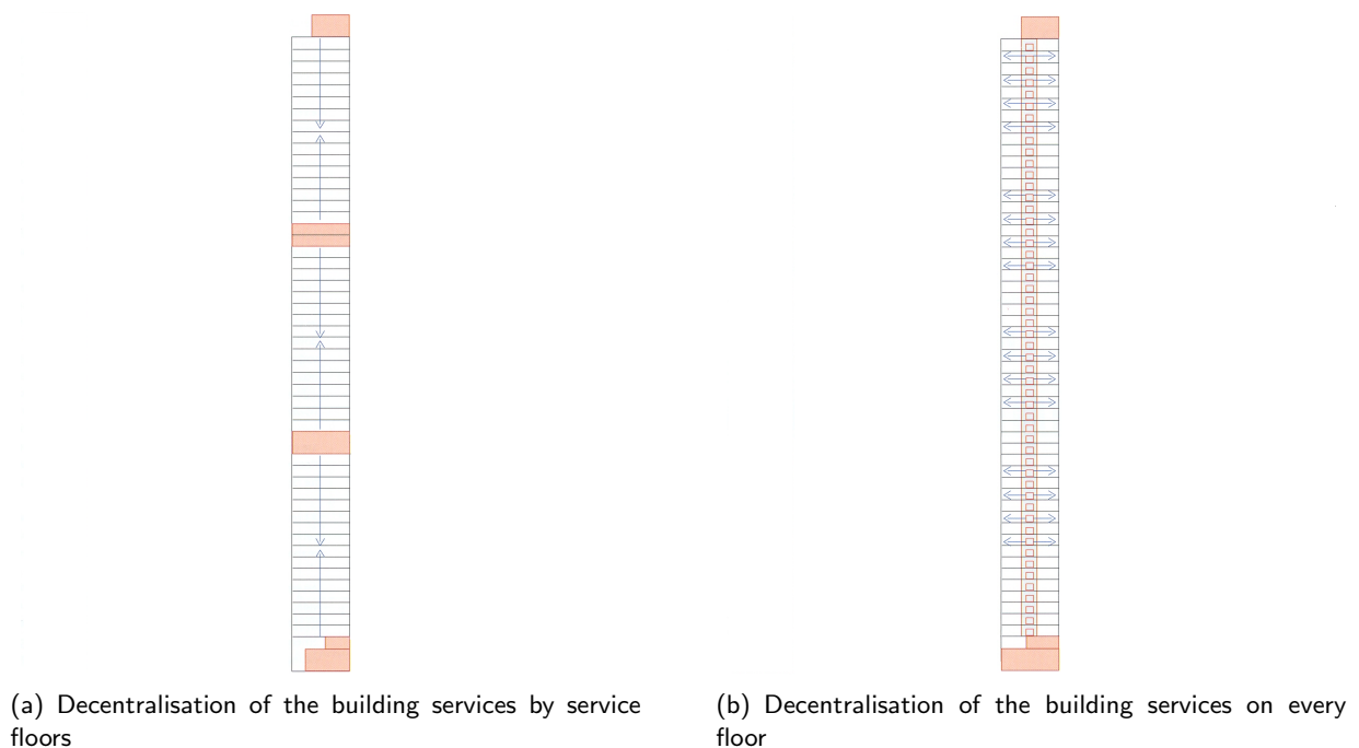
Figure 3.42: Decentralisation of building services
