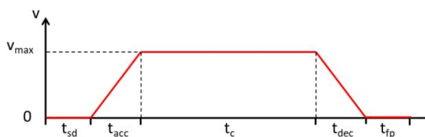
**Figure 3** The model to determine the process time of a yard crane component movement process where  $v_{max}$  is the maximum speed.
