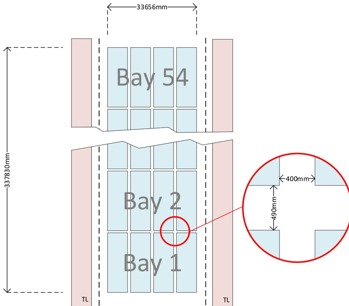
**Figure 15 Schematic top view of the reference case storage yard layout**
