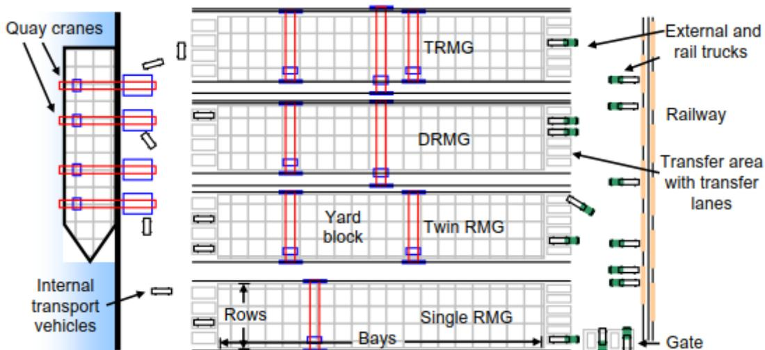
**Figure 13** The four yard crane configurations for automated container terminals shown in a schematic top view, each block represents a different yard crane configuration [11]
