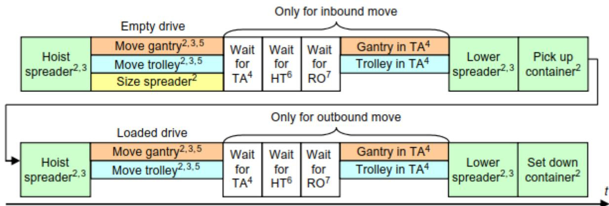
**Figure 8** Operational sequence of a yard crane container handling cycle where the transfer area (TA), the horizontal transport (HT) and the remote operation (RO) is taken into account. [11]
