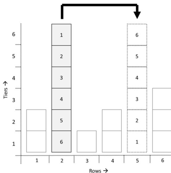
**Figure 4 Schematic representation of a job batch procedure executed by the automated yard crane from the reference case.**
