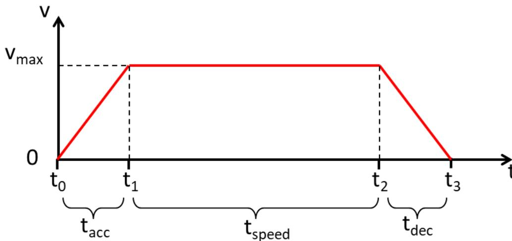
**Figure 21 A model of the theoretical exact movement time**
