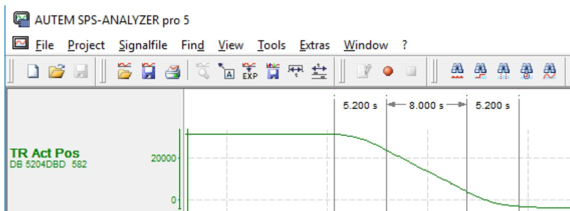
**Figure 20 An example of measurements of a trolley move process from a PLC-trace**
