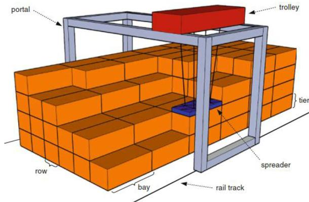
**Figure 1** Schematic overview of a yard crane system on a storage yard block, the portal moves on a rail track and supports a trolley, a spreader is suspended from the trolley which can connect to a container. [5]
