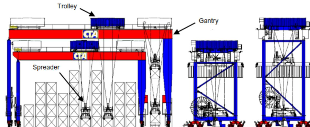
**Figure 14 Schematic side view of two yard cranes with a DRMG configuration, the yard cranes can pass each other when the trolley of the large yard crane is on a dedicated position [11]**
