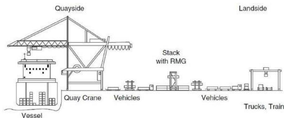
**Figure 1 Schematic sideview of a container terminal showing the quayside, storage yard and landside operational areas [2]**
