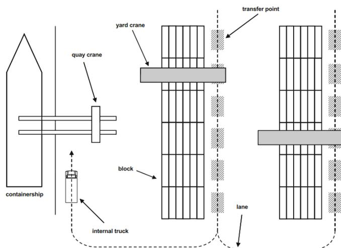
Figure 11 Side loading transfer point block configuration (Asian) [41]
