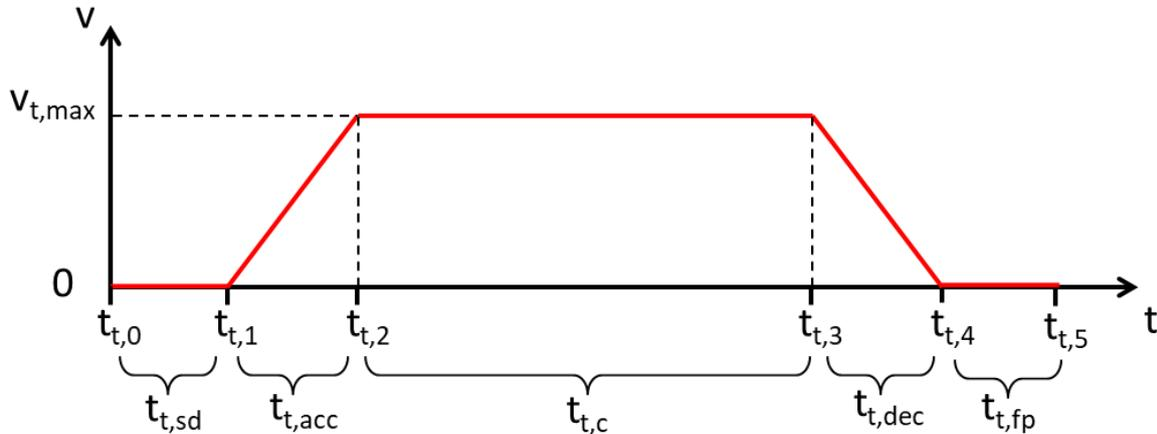
**Figure 18 Modeling the trolley movement process block**
