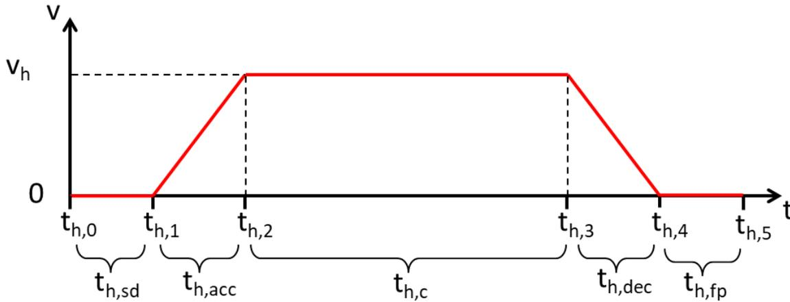
**Figure 19 Modeling the hoist movement process block**
