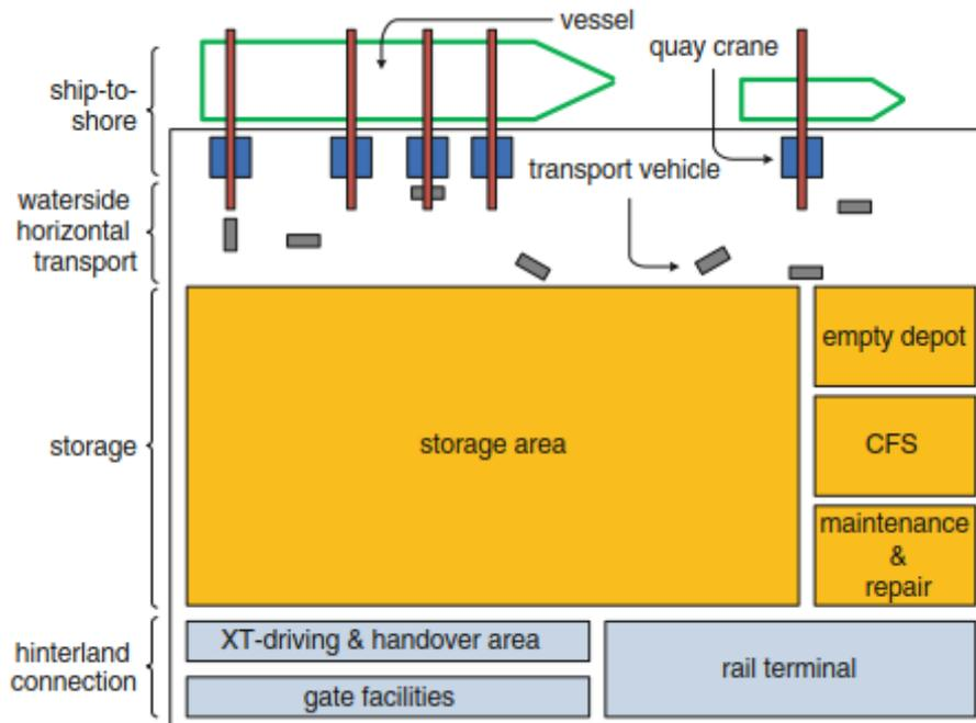
**Figure 5 Schematic top view of a container terminal [5]**
