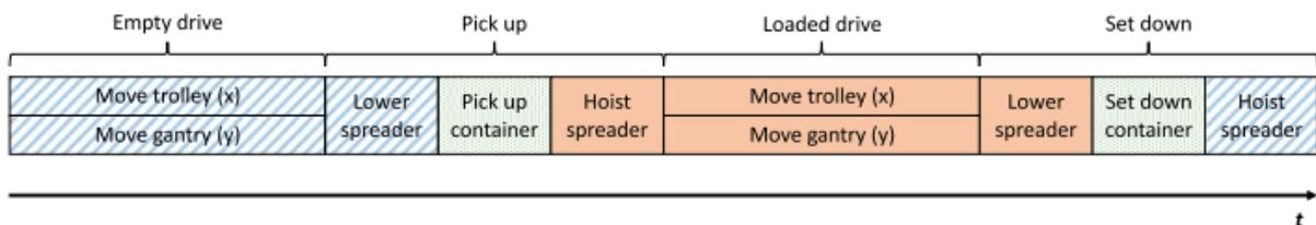
**Figure 7 Typical operational sequence of a yard crane container handling cycle [10]**
