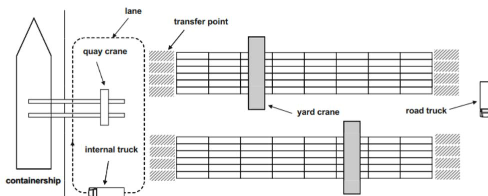
Figure 12 End loading transfer point block configuration (European) [41]
