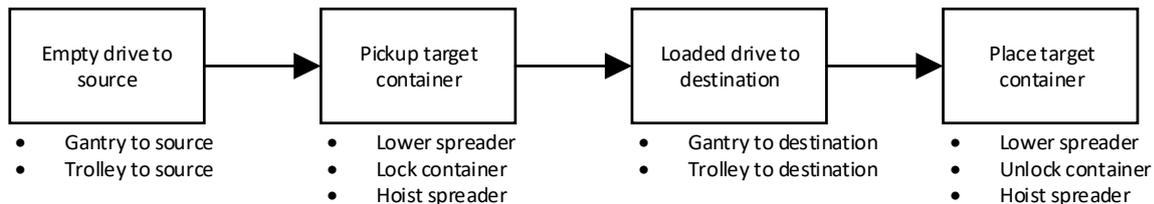
**Figure 9** The four basic yard crane processes and subprocesses to complete a container handling cycle
