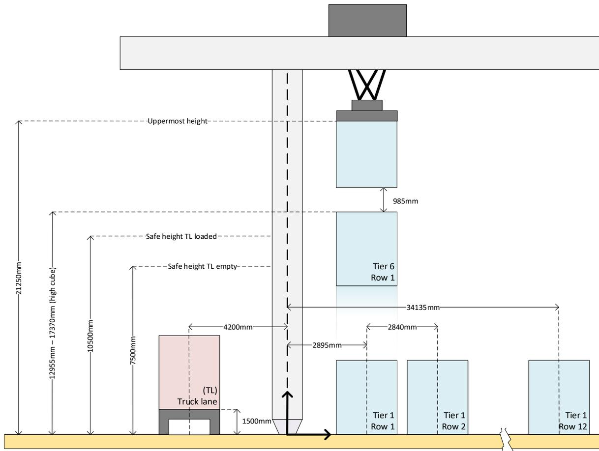
Figure 16 Schematic side view of the reference case storage yard configuration
