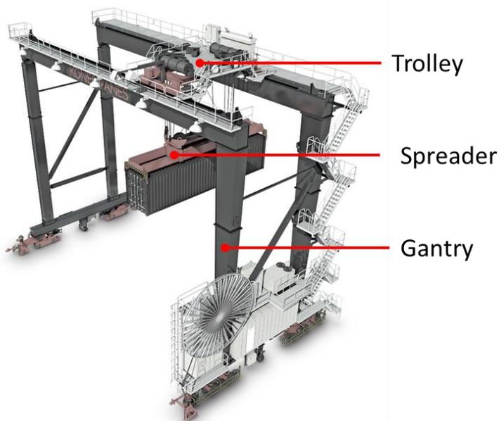
**Figure 3 An automated rail mounted gantry crane with the three main moving components highlighted [7]**
