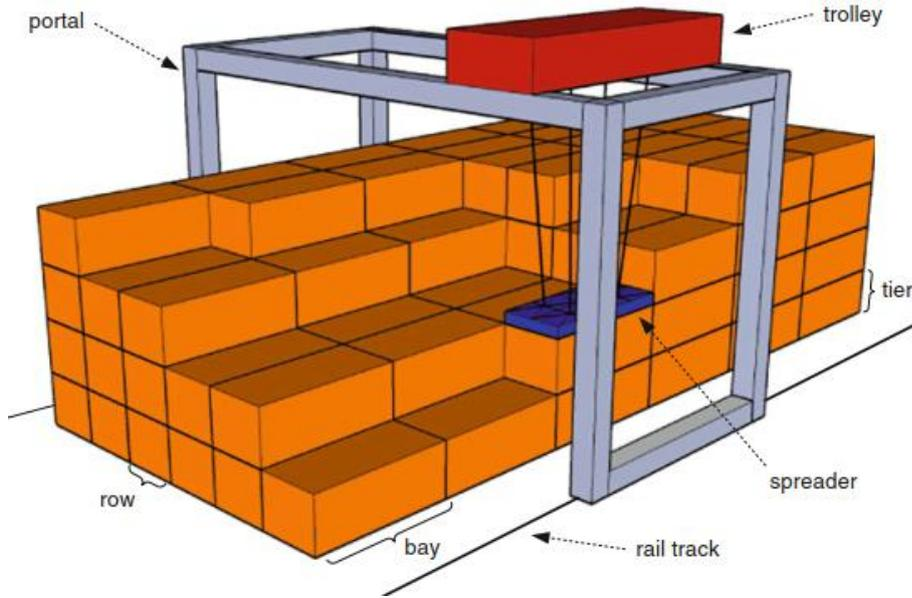
**Figure 6 Schematic overview of a yard crane system on a storage yard block, the portal moves on a rail track and supports a trolley, a spreader is suspended from the trolley which can connect to a container [5]**
