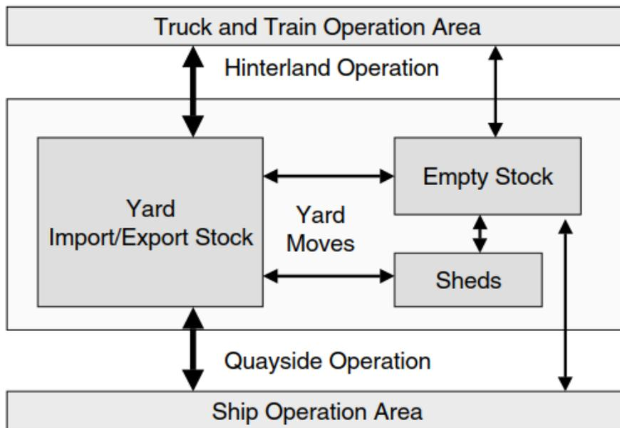
Figure 4 Diagram of operational areas and flow of transports on a container terminal [2]
