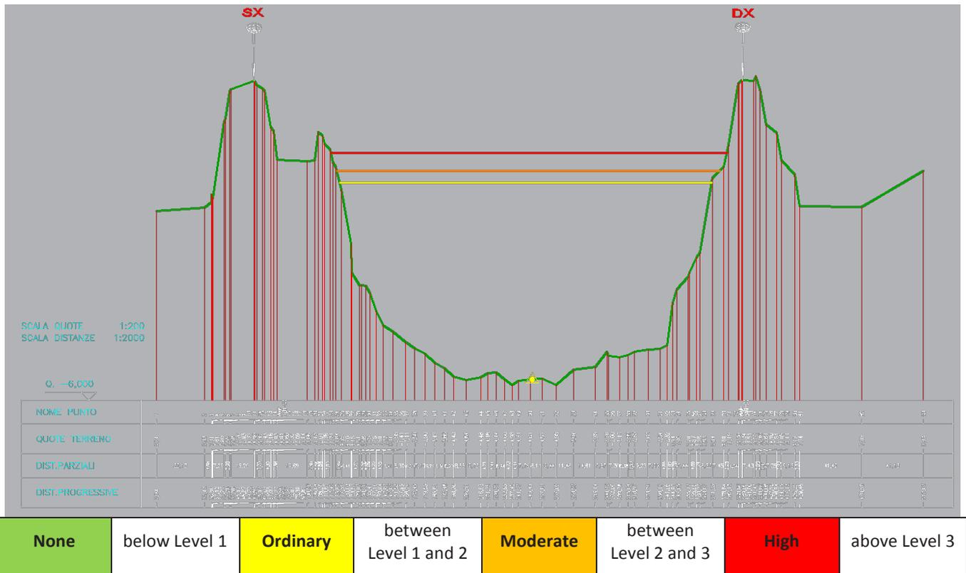
Figure 4.1. Example of flood alert threshold at Pontelagoscuro section: yellow line = level 1; orange line = level 2, red line = level 3.
