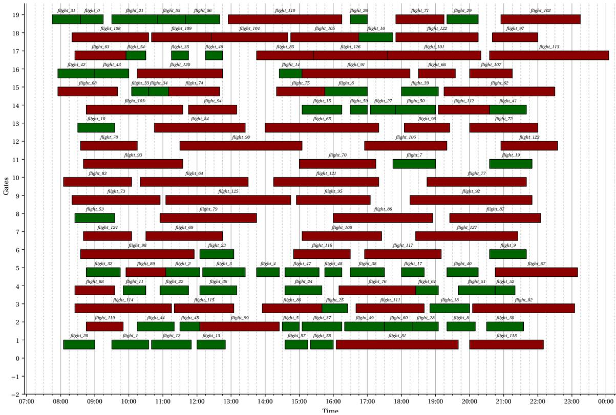
Figure 5.2: Initial gate assignment where the minimal number of gates is used for scenario two. Where green and red indicate respectively; narrow-body, wide-body flights. Blue represents narrow- or wide-body flights that have been split
