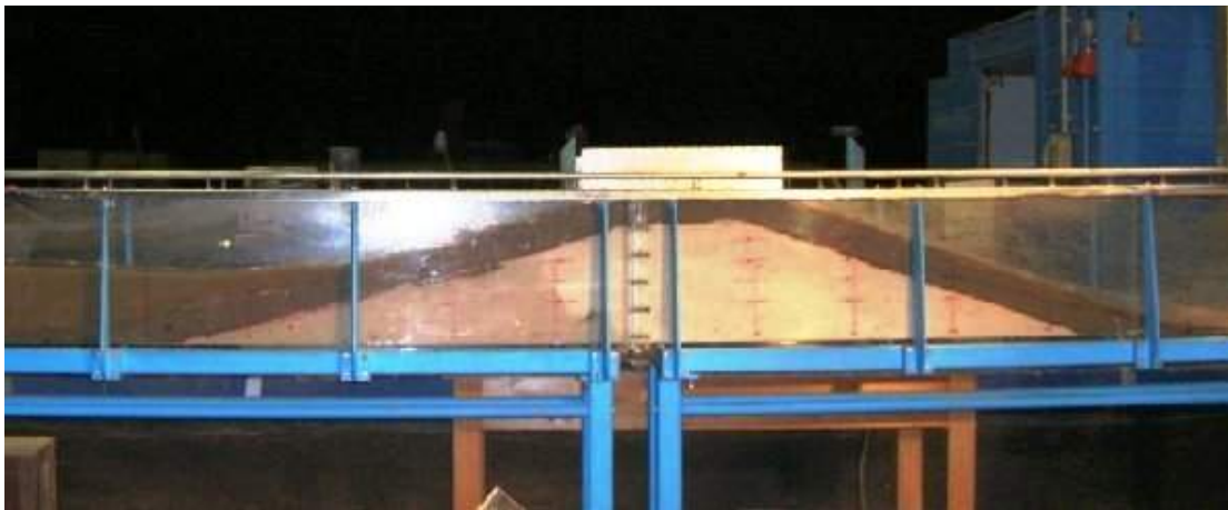
Figure 4-14 Seepage after clay cover failure
