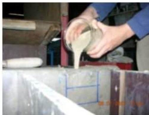
Sand replacement method for density measurement
