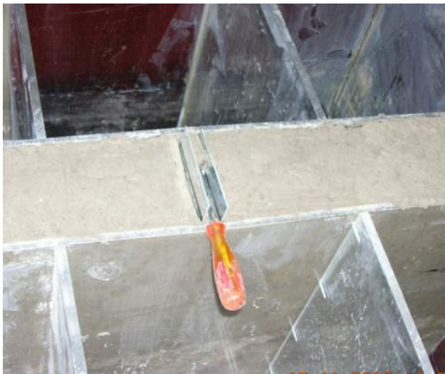
Figure 3-5 The making of artificial crack
