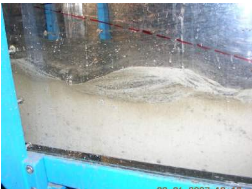
Figure 4-17 Sand bar formation along the new slope of damaged dike
