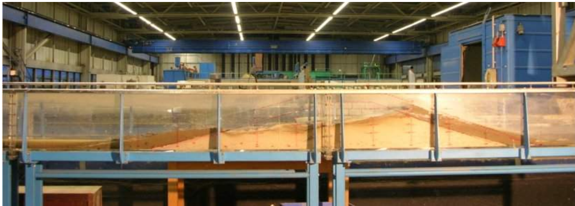
Final Profile of the failed dike. No breaching occurred due to single factor of breaking wave impacts
