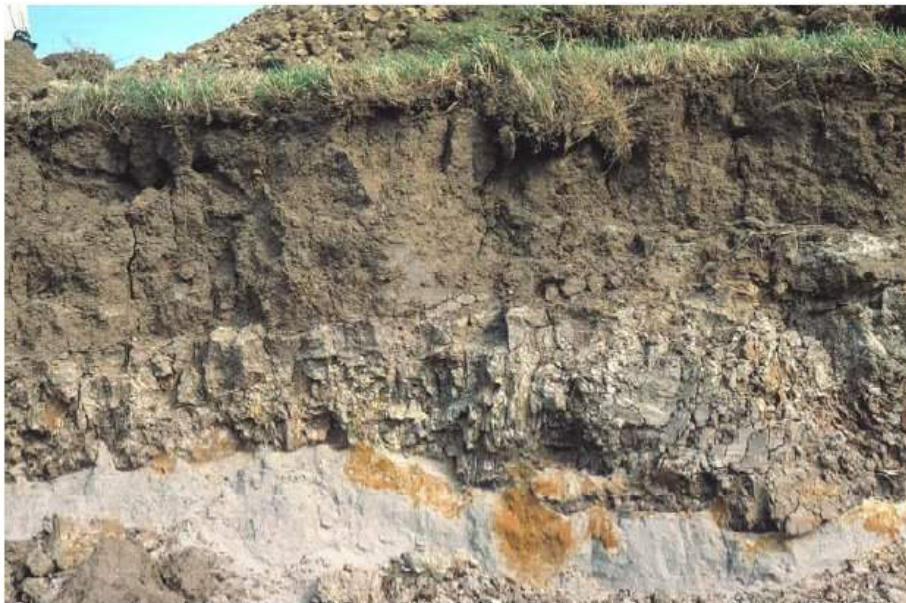
Figure 2-2 Cross section of a clay layer showing soil structures in the forms of cracks and pores as results of water content changes and biological activities (TAW, 1996)
