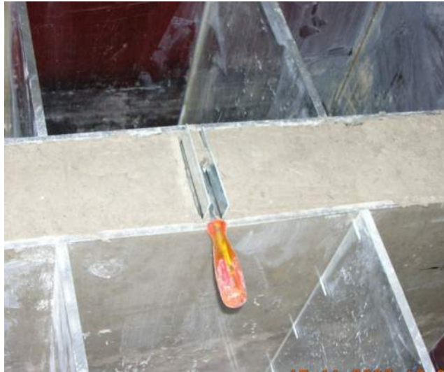
The making of artificial crack. The soil between 2 inserted thin plates is dig out
