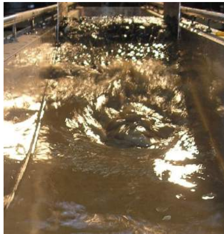
Figure 4-12 Location of breaking waves below the mean water level creating impacts on the dike slope.
