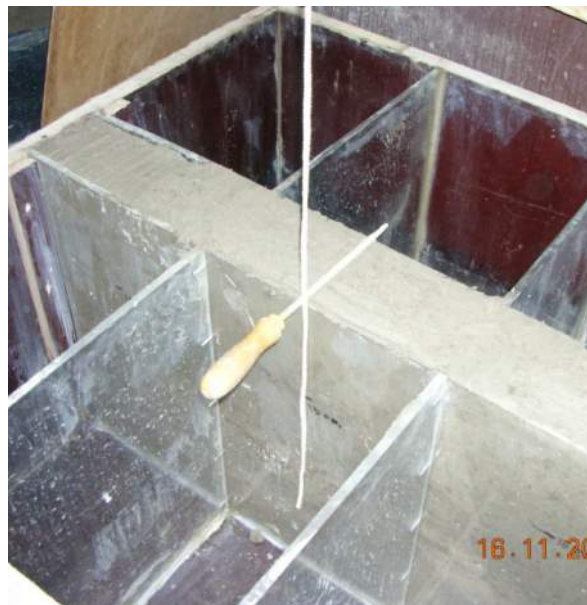
Crack location positioning by using weighted rope
