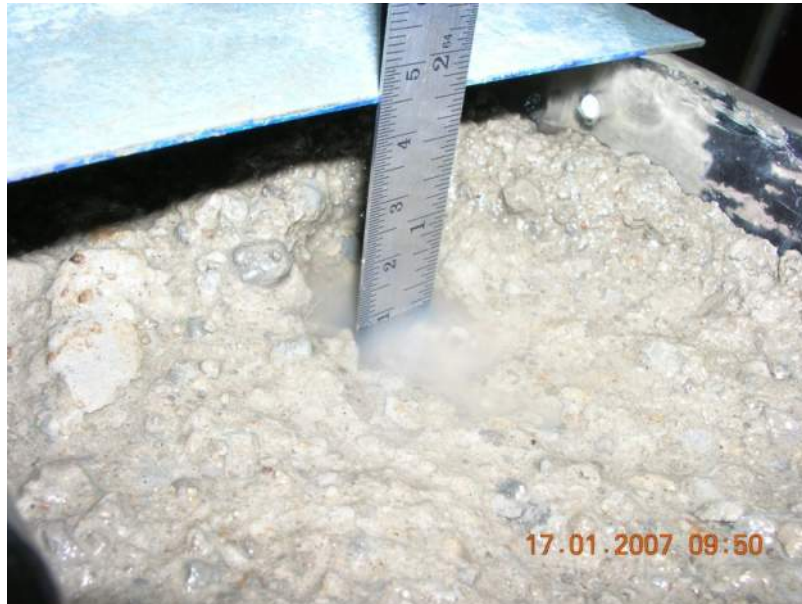
Eroded soil measurement by a ruler to measure the deepest part of scour hole
