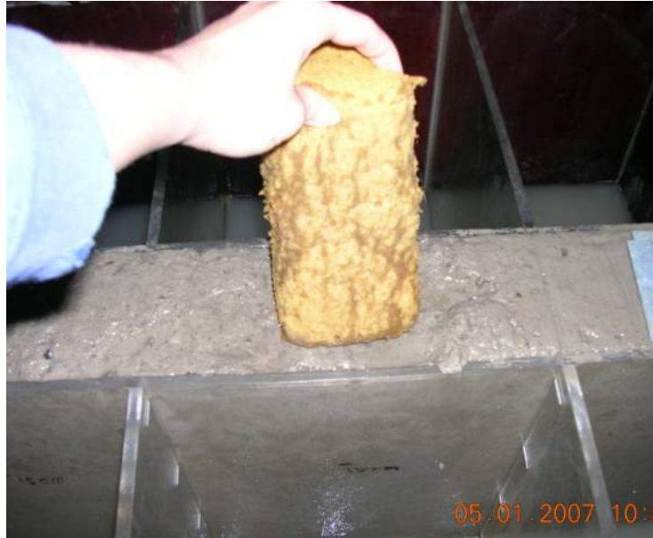
Removing water from the scour hole to avoid water layer
