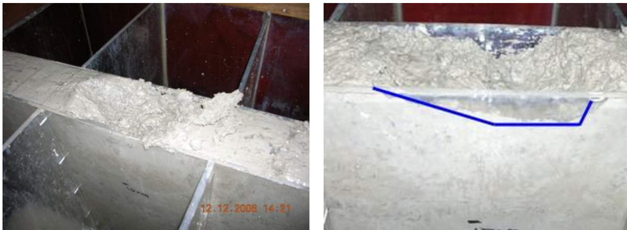
Figure 5-21 An imperfect falling-water mass and its asymmetrically crater-like scour hole
