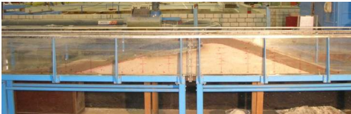
Figure 4-22 Final Profile of model 2 after being hit by breaking wave impacts for 45 hours.
