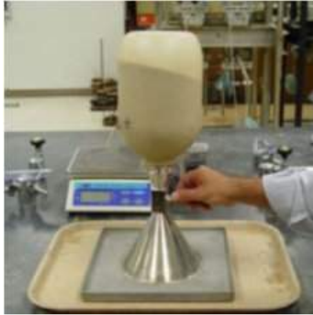
Figure E-3. Standard Sand Cone apparatus, not available at LWI (From geotechnical laboratory, University of Texas at Arlington)
