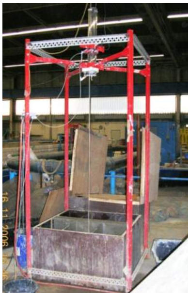
Crack location positioning by using weighted rope
