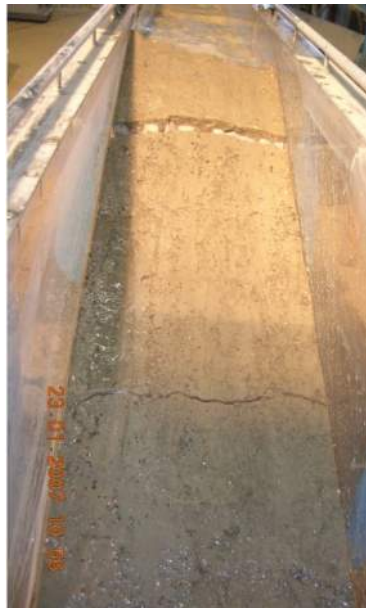
Figure 4-18 Flow slide cause the whole body of inner slope to move. Cracks appeared due to movement of the sand core.
