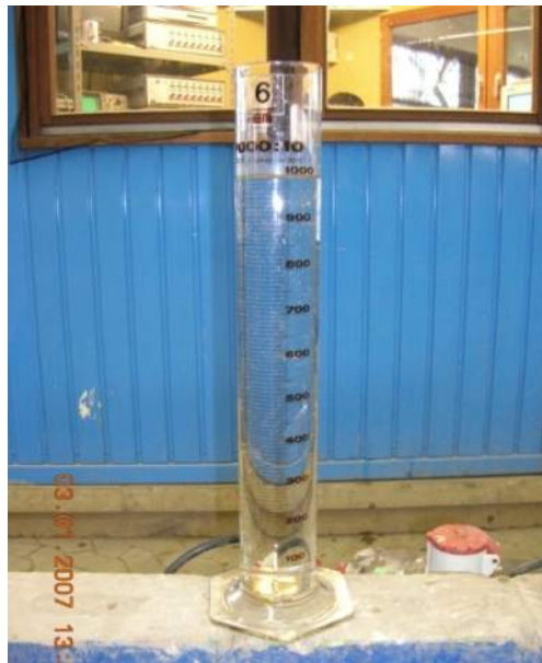
A glass beaker for eroded soil measurement. The difference reading between before and after pouring water into the scour hole is the eroded soil volume.
