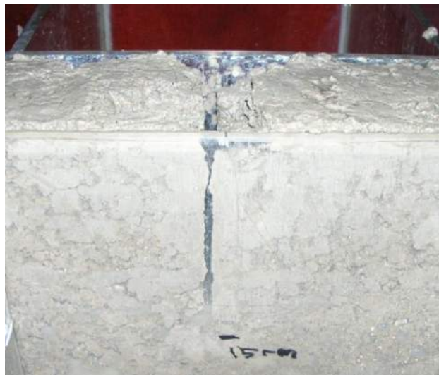
Figure 4-3 Damage around the surface of the water-filled crack
