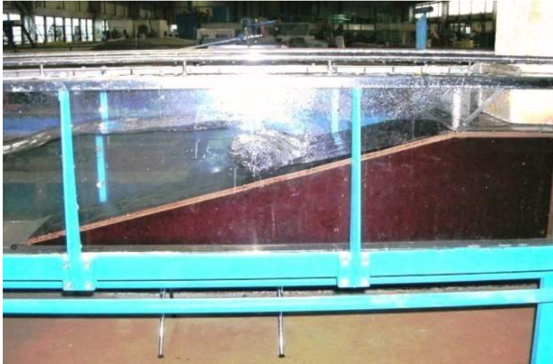
Figure 3-10 Dummy dike made from plywood for wave characteristics investigation before real experiments.
