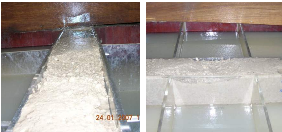
Figure 5-17 Less compacted samples cause side erosion and lead to early severe damage
