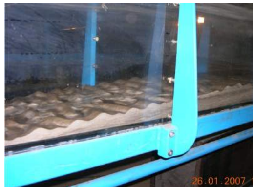
Figure 4-17 Sand bar formation along the new slope of damaged dike
