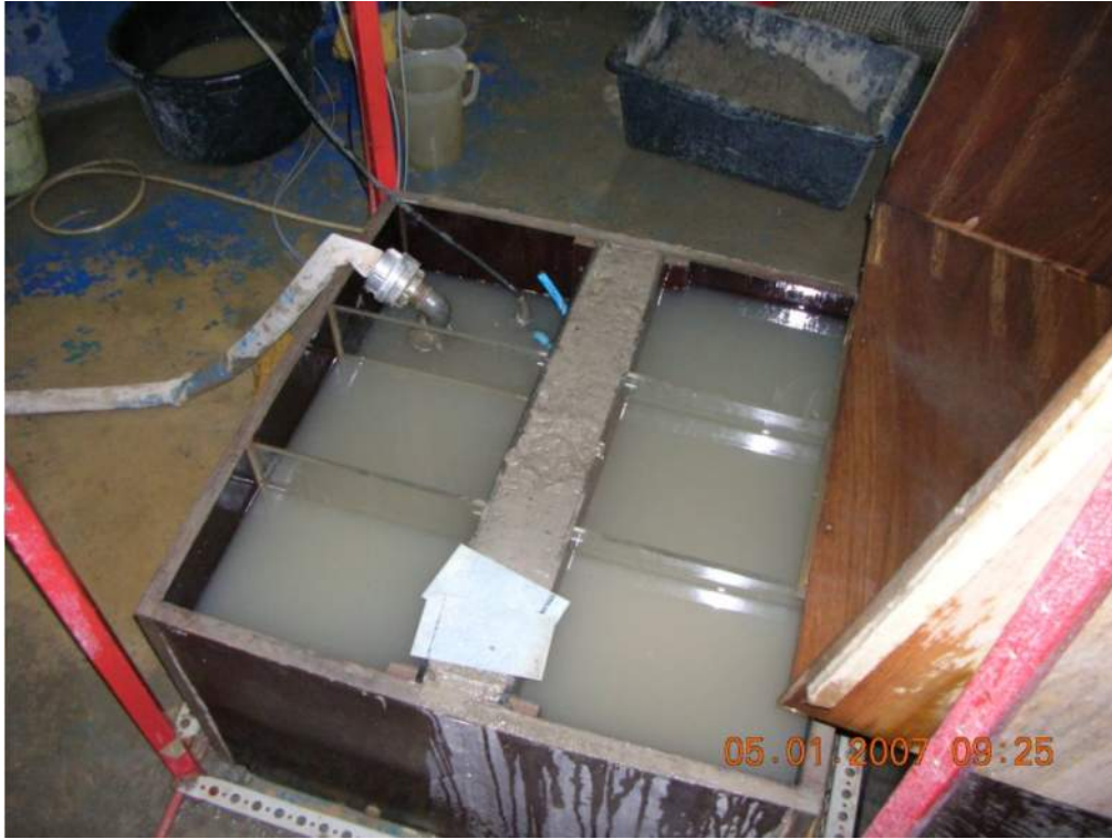
Pumping out the water from the wooden box compartment
