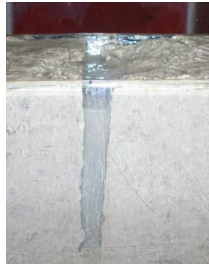
Figure 4-2 Small damage along the weak line after 12 th impact.
