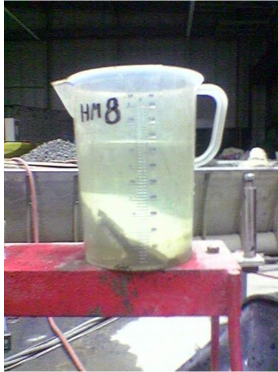
Volume measurement by applying Archimedes law
