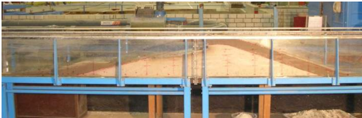
Final Profile of model 2 after being hit by breaking wave impacts for 3 days.
