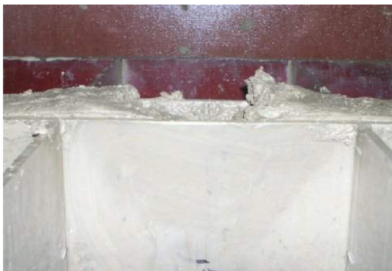
Figure 4-5 Crater-like shape of the eroded surface for the test with very high water content.
