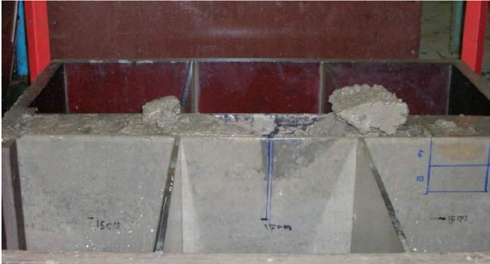
Figure 4-7 Blocks of soil are removed after releasing several impacts
