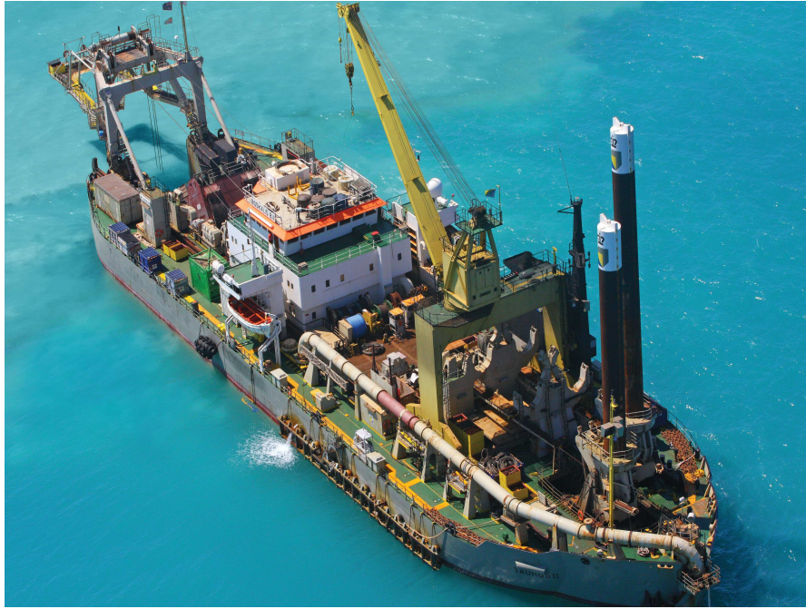
(a) The Taurus II cutter suction dredger
