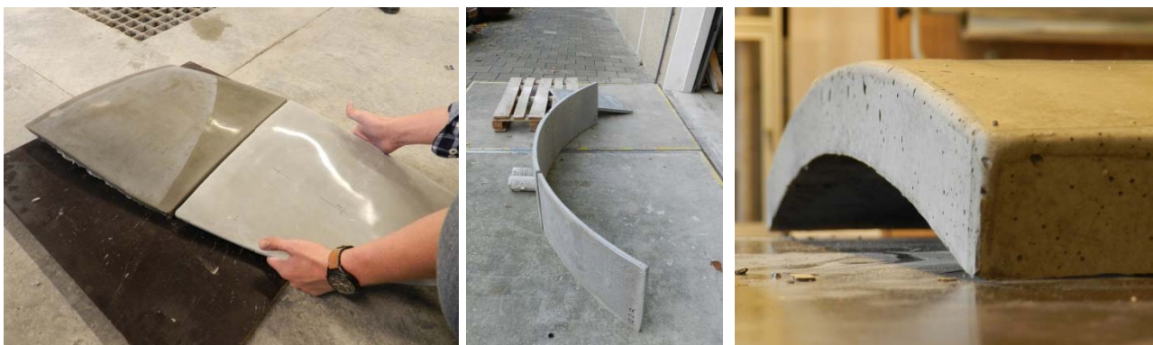
Figure 8 - Configurations of successfully deformed double-curved (left) and single-curved (middle) panels to be used as cladding elements (thickness 25 mm), and a single-curved element (right, h=50 mm)
