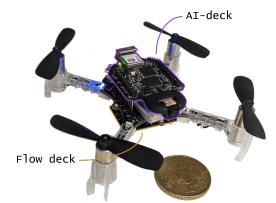
Fig. 6: We use the Crazyflie 2.x as the flight platform for our experiments. We use the AI-deck to capture images with the front-facing camera and to run optical flow inference and processing. The downward-facing optical flow deck is used for positioning only. The total flight platform weighs in at 34 grams.
