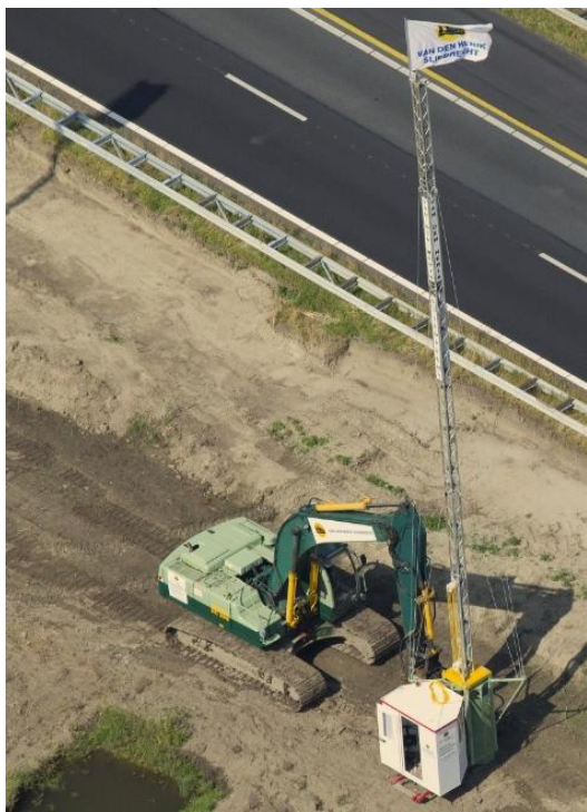
Figure 2. A probing crane with magnetocone instrumentation (Source: van den Herik, Slidrecht)
