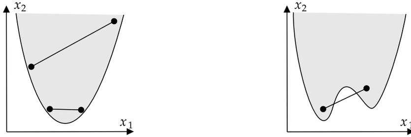
Figure B.1.: Convex function (left) and a non-convex function (right).
