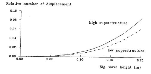
Fig. 4. Comparison of low superstructure with high superstructure
