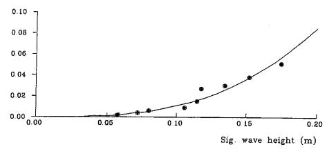
Fig. 3. D vs.  $H_{mo}^t$  of Dolosse breakwater with a high superstructure.
