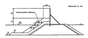
Fig. 1. Lay-out of the round head in wave basin
