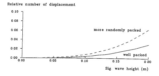
Fig. 5. Comparison of well packed slope with more randomly packed slope. Low superstructure
