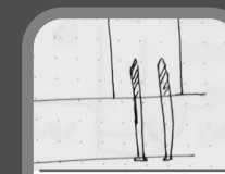
Screw in from the bottom
