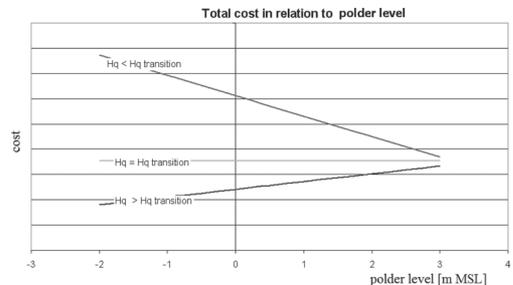
Figure 5. Total cost in relation to polder level for different quay wall heights.
