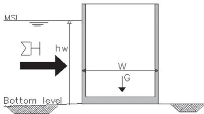
Figure 6. Resultant horizontal force in direction of terminal side of quay wall.
