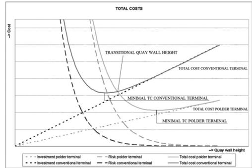
Figure 3. Risk framework optimization for a conventional and a polder terminal (conceptual graph).
