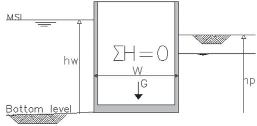
Figure 7. No resultant horizontal force on quay wall.
