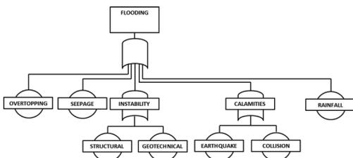
Figure 4. Fault tree for flooding of polder terminal.
