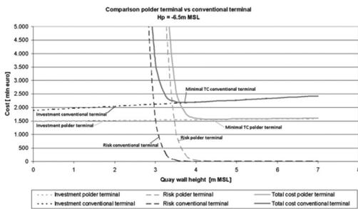
Figure 10. Comparison of total cost polder terminal vs conventional terminal (Reclamation = 20 €/m<sup>3</sup>).
