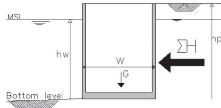
Figure 8. Resultant horizontal force in direction of polder side of quay wall.
