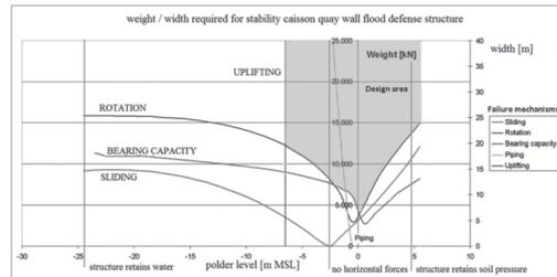
Figure 9. Required width of gravity structure related to the polder level (depth) for case study (4.1).
