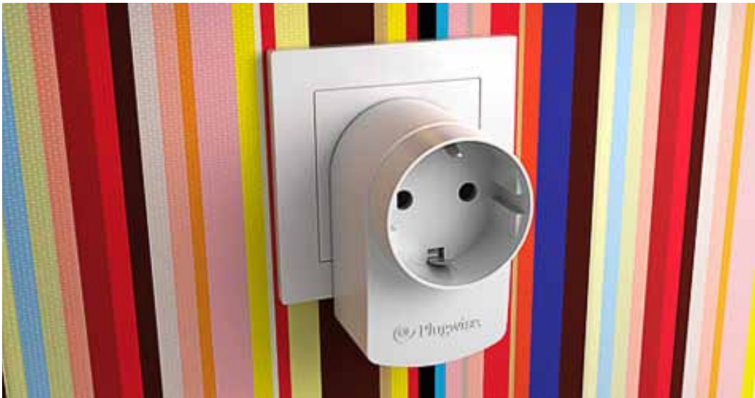
Figure 3 The 'Plugwise' energy management device used in case study 2.
