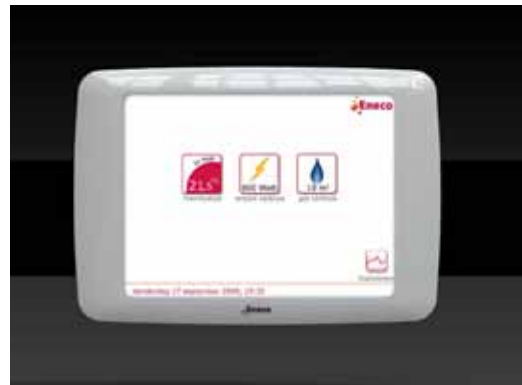
Figure 4 Multifunctional HEMS used in case study 3 (picture 1 displays the start screen for the 'smart' meter, picture 2 displays the start screen for the 'dumb' meter).
