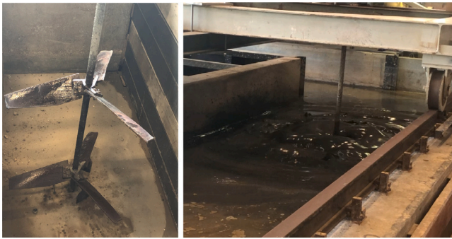
Fig. 2. The rotating mixer used to homogenise the mud. The right panel shows the mixer in action.
