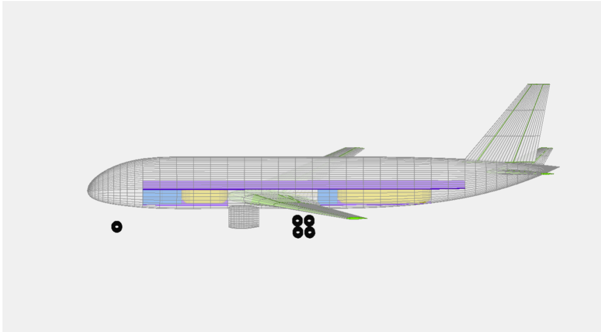
Figure 4.8: LNG tanks configuration. ULDs(blue) and cryogenic tanks(yellow) layout.
