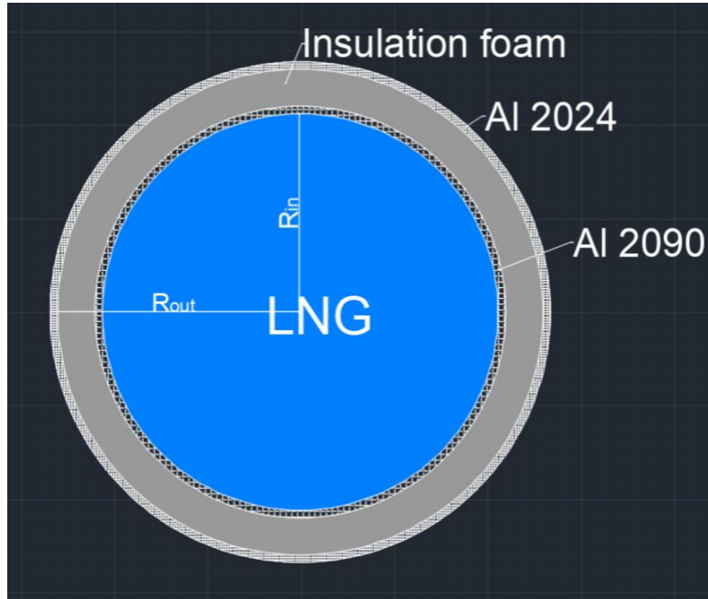
Figure 3.1. Cross section view of the cryogenic tank.
