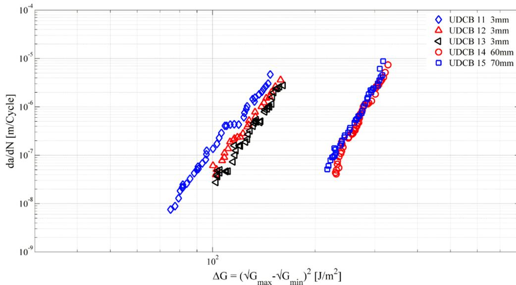
Figure 4.4. Fatigue resistance curve with fully developed fibre bridging
