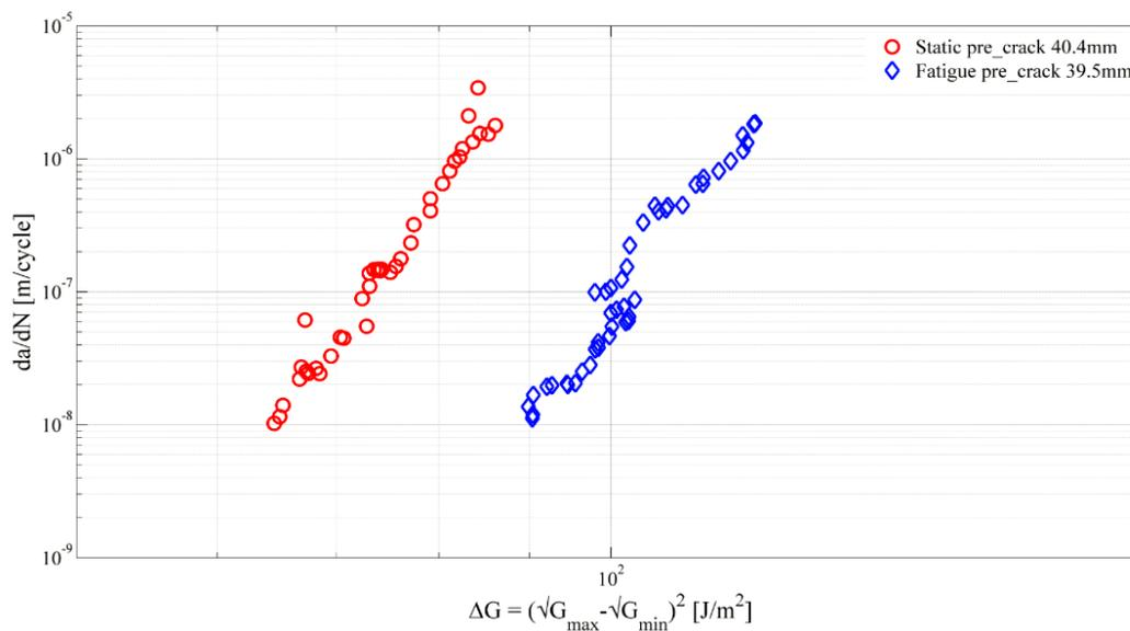
(a) Specimens UDCB 19 and UDCB 20 with 40mm pre-crack lengths
