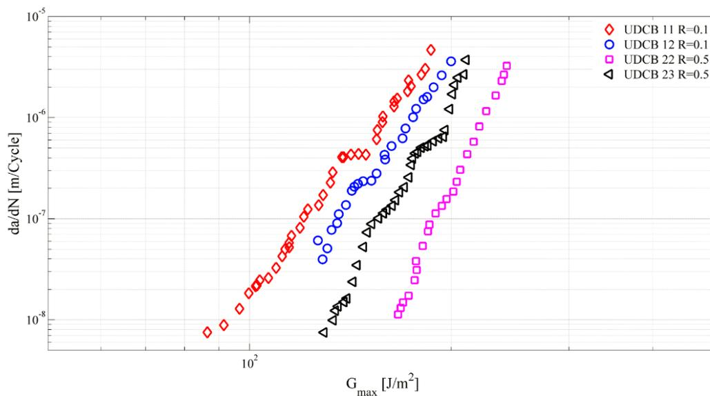
(a)  $da/dN$  vs.  $G_{max}$  for the 0//0 Interface
