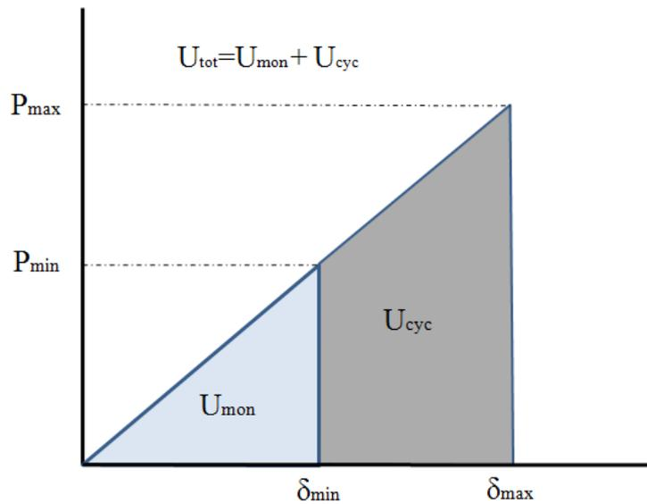
Figure 8.1 Schematic of the energy components in a fatigue load
