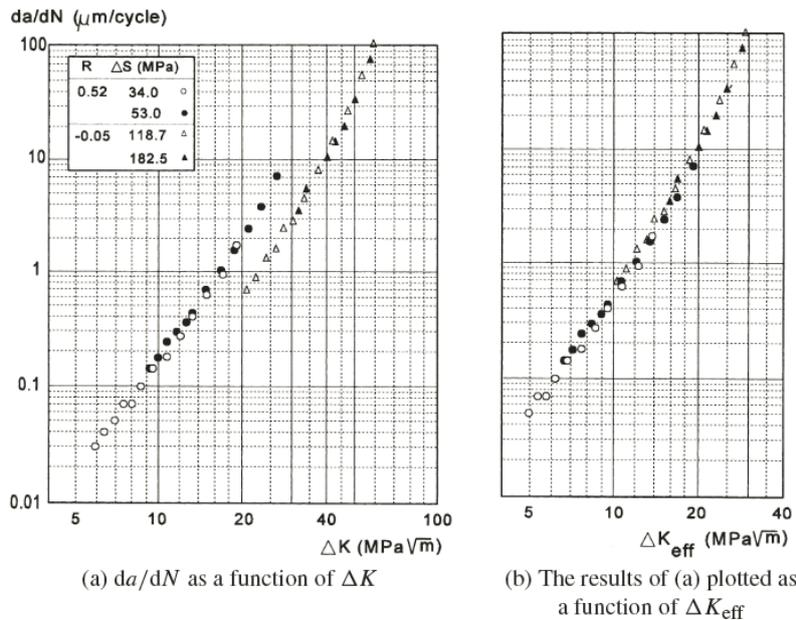
Figure 2.2 Fatigue crack growth correlated to  $\Delta K$  and  $\Delta K_{eff}$  in Al-alloy (2024-T3) at different stress ratios [35]
