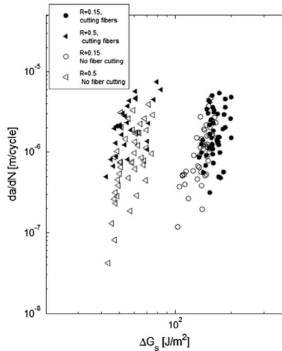
Figure 2.5 Fatigue tests with and without bridging fibre cutting [36]
