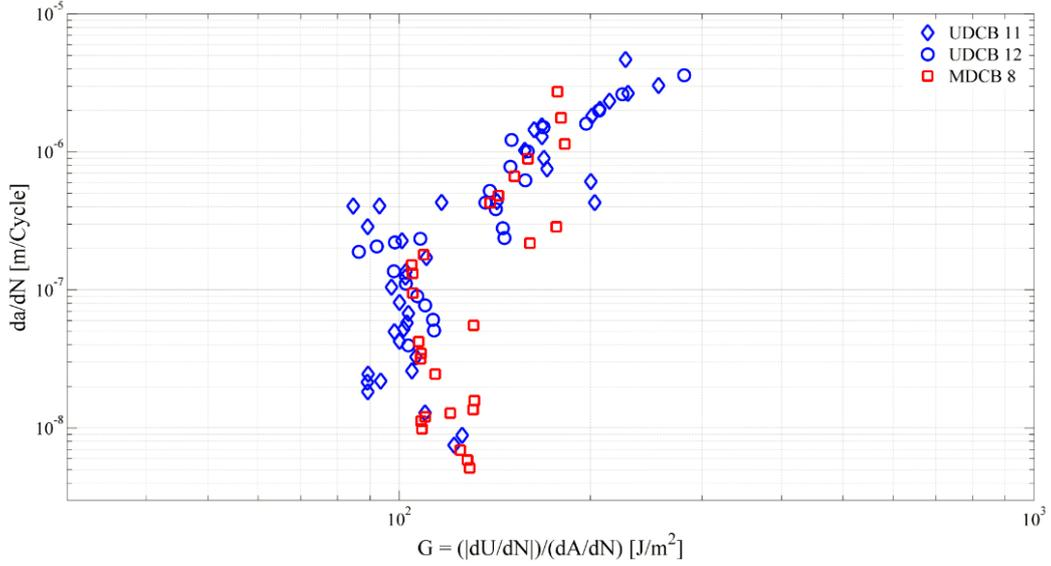
Figure 7.2  $da/dN$  vs.  $G$  at the stress ratio of  $R=0.1$
