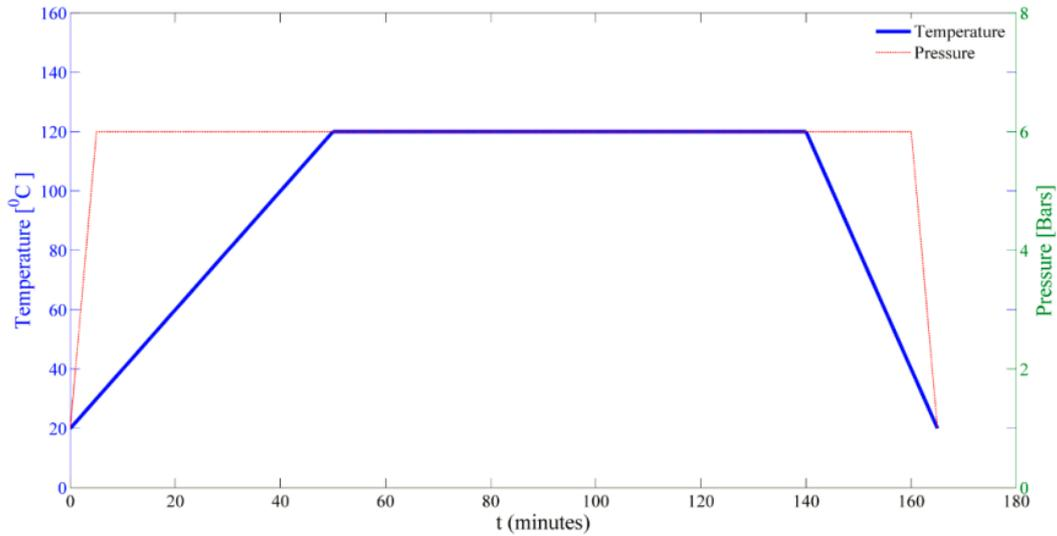
Figure 3.2 M30SC/DT120 curing procedure.
