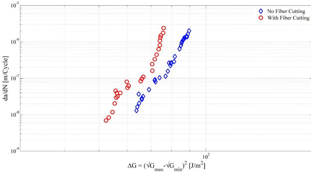
Figure 4.5. Fatigue resistance curve for fibre cutting
