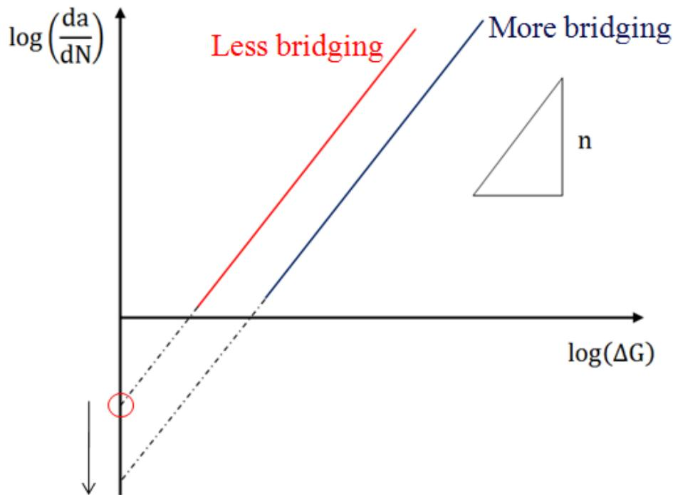
Figure 5.5 Schematic of  $\log(C)$  decrease with the increase of fibre bridging
