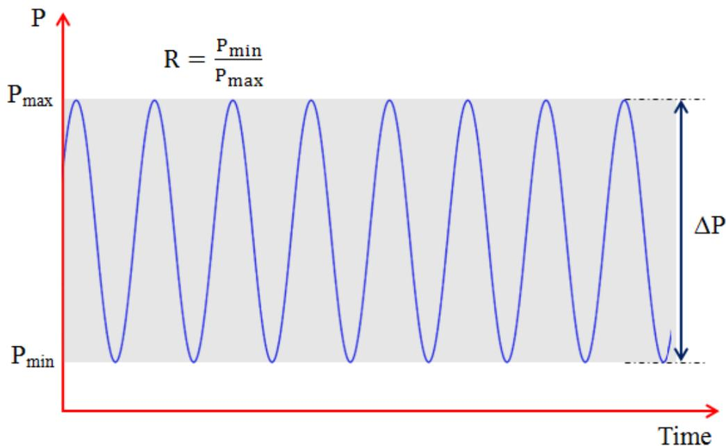
Figure 2.3 Constant amplitude fatigue load
