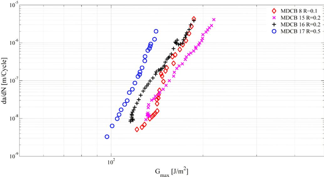
(b)  $da/dN$  vs.  $G_{max}$  for the 45//45 Interface
