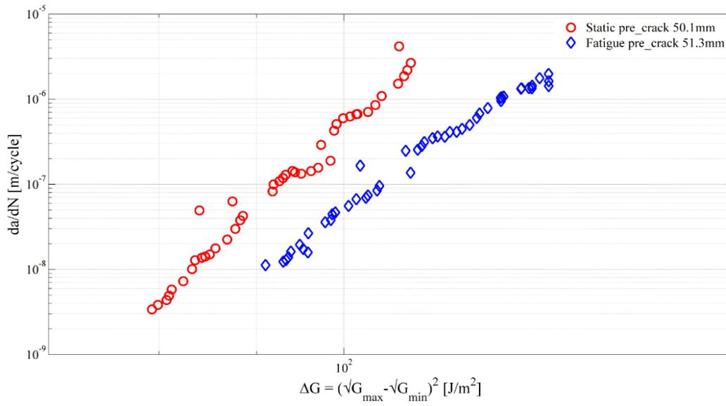
(b) Specimens UDCB 19 and UDCB 21 with 50mm pre-crack lengths
