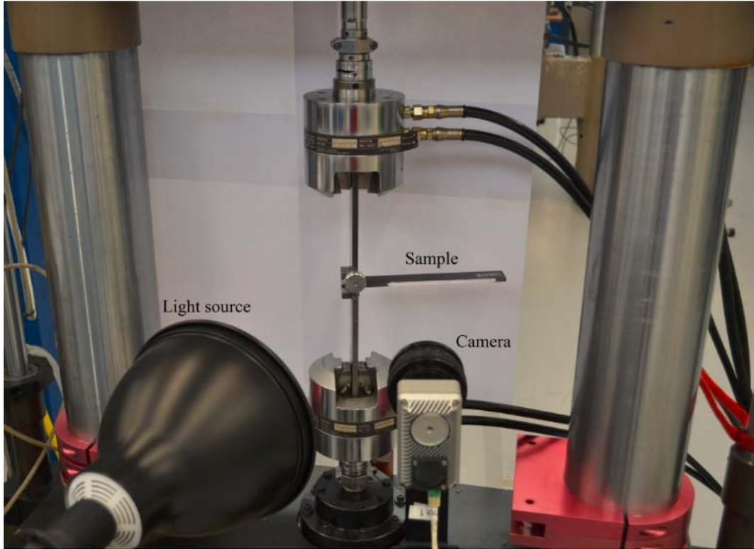
Figure 3.6 Fatigue experimental setup
