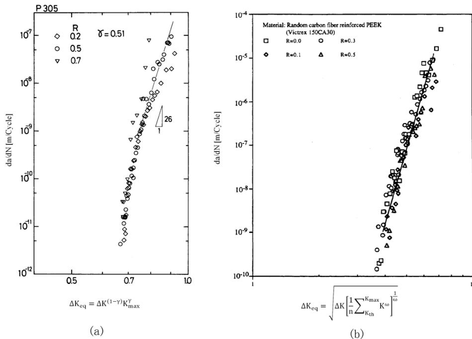
Figure 2.4 Two-parameter fatigue models
