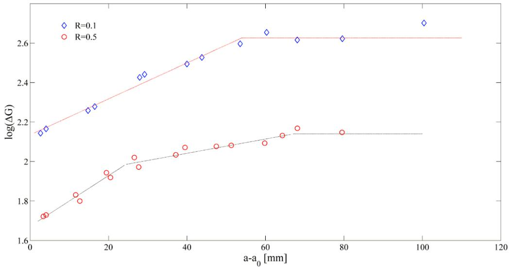
Figure 5.7  $\log(\Delta G)$  vs.  $a-a_0$  in the 0//0 interface ( $da/dN = 1\times 10^{-6}$  m/Cycle)
