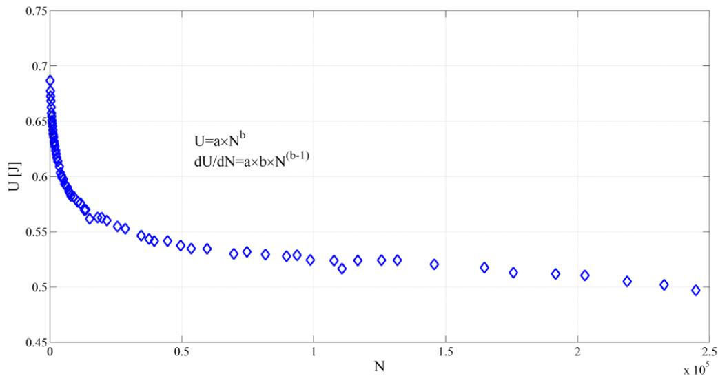
Figure 6.3 Applied work  $U$  versus number of cycles  $N$
