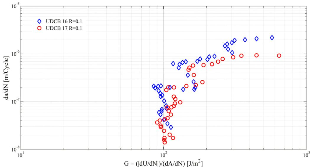
Figure 7.4 0//0 Interface with 15mm pre-crack length
