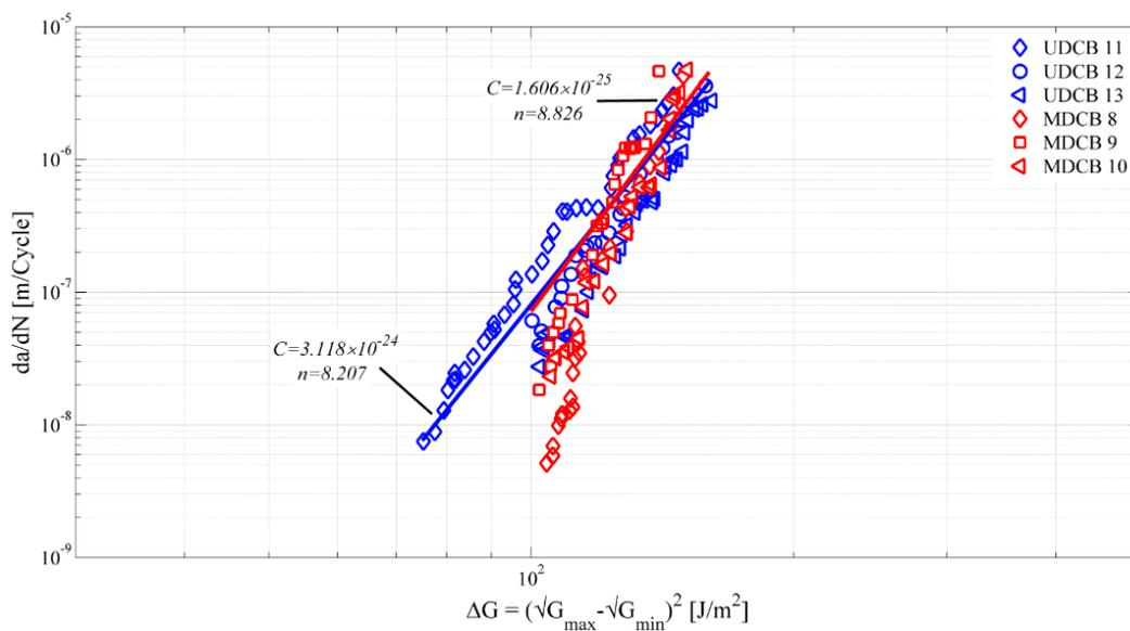
Figure 4.6. Bridging effect on the slope of fatigue resistance curve
