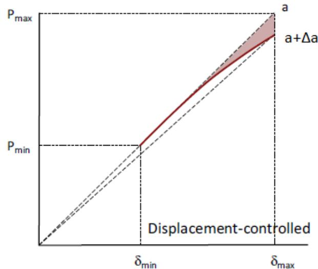
Figure 6.2 Non-linear response during fatigue loading [24]
