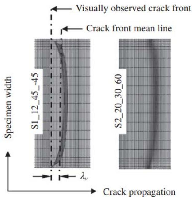
Figure 3.1 Curvature of the delamination front
