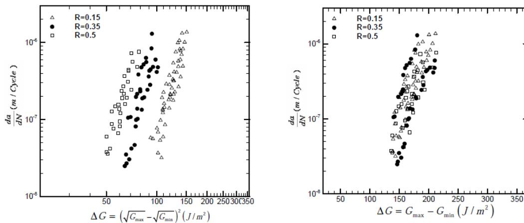
Figure 2.1 Fatigue crack growth rate against different definitions of *SERR* range [32]
