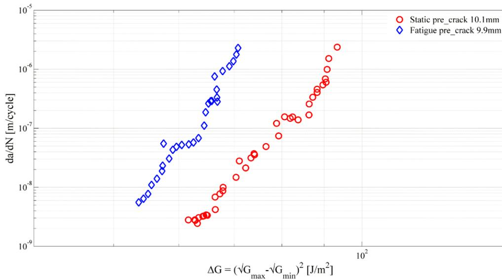
(c) Specimens MDCB 11 and MDCB 13 with 10mm pre-crack lengths
