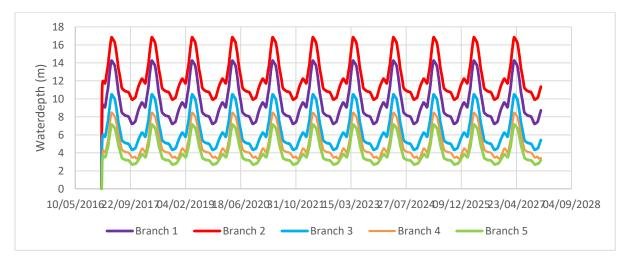
Figure B. 4.4 Water depth in Tigris branches when all nodes are open and Branch 1 is closed
