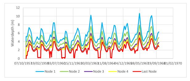
Figure B. 14.4 Water depth in Euphrates when the cross-section of branch 5 decreases 20%
