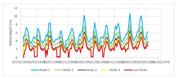
Figure B. 14.1 Water depth in Euphrates when the cross-section of branch 4 decreases 20%
