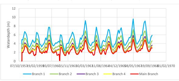
Figure B. 9.1 Water depth in Euphrates when the last 3 irrigation Nodes are open
