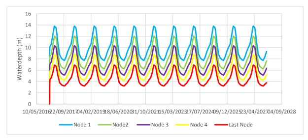
Figure B. 2.2 Water depth in Tigris when all nodes are open and with average flow
