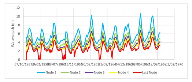
Figure B. 14.3 Water depth in Euphrates when the cross-section of branch 4 is closed
