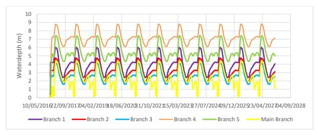
Figure B. 7.2 Water depth in Euphrates branches when all nodes are open and branch 5 and branch 6 are closed
