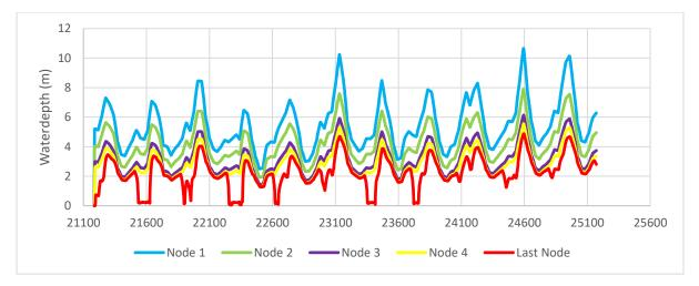
Figure B. 13.1 Water depth in Euphrates when the cross-section of branch 3 decreases 20%
