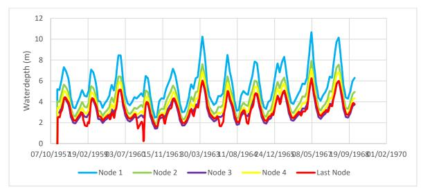
Figure B. 14.6 Water depth in Euphrates when the cross-section of branch 5 is closed
