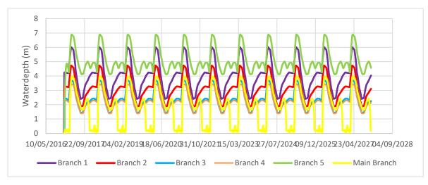
Figure B. 6.2 Water depth in Euphrates branches when all nodes are open and branch5 is closed
