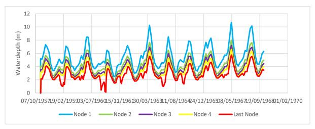
Figure B. 13.3 Water depth in Euphrates when the cross-section of branch 3 is closed
