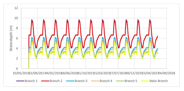
Figure B. 5.1 Water depth in Euphrates when all nodes are open and branch 1 and 2 are closed
