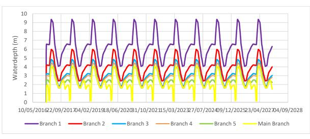
Figure B. 4.1 Water depth in Euphrates when all nodes are open and Branch 1 is closed
