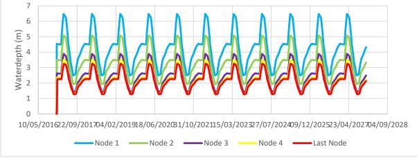
Figure B. 1.1 Water depth in Euphrates when there are no nodes and with minimum flow
