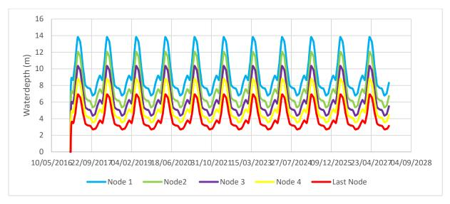
Figure B. 4.3 Water depth in Tigris when all nodes are open and Branch 1 is closed
