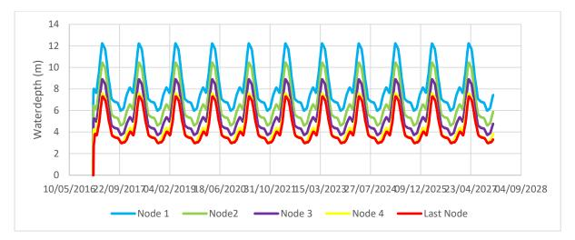
Figure B. 6.3 Water depth in Euphrates when all nodes are open and branch 5 closed
