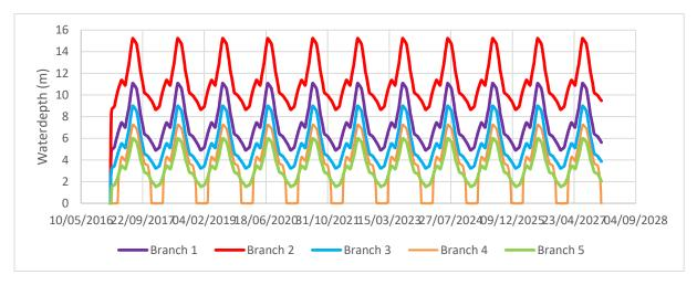
Figure B. 3.4 Water depth in Euphrates branches when all nodes are open and with minimum flow
