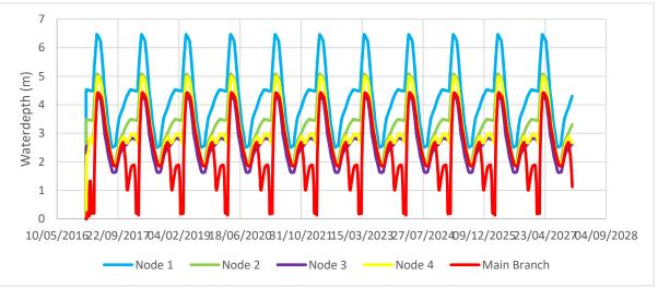
Figure B. 7.1 Water depth in Euphrates when all nodes are open and branch 5 and branch 6 are closed
