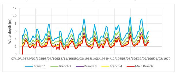
Figure B. 10.1 Water depth in Euphrates when the first 16 irrigation nodes are open
