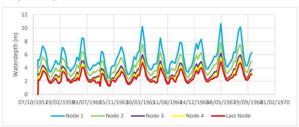
In Figures B.9.3.-B.9.4. the water depth in Euphrates when only the last 2 irrigation nodes of the system are open is shown:
