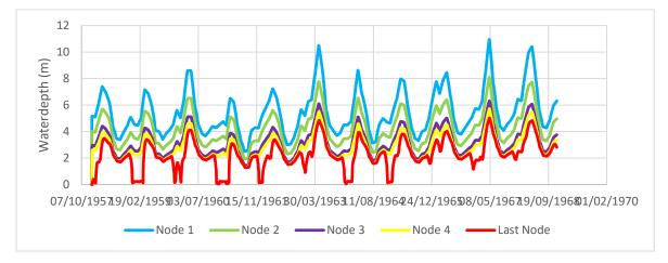
Figure B. 11.1 Water depth in Euphrates when the cross-section of branch 1 decreases 20%
