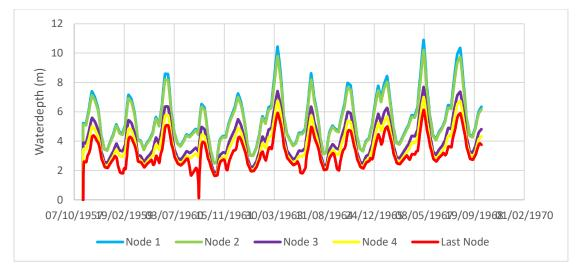
Figure B. 11.3 Water depth in Euphrates when the cross-section of branch 1 is closed
