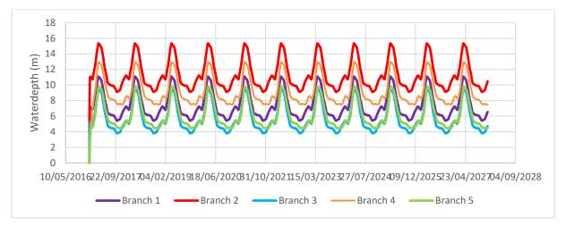
Figure B. 7.3 Water depth in Tigris when all nodes are open and branch 5 and branch 6 are closed
