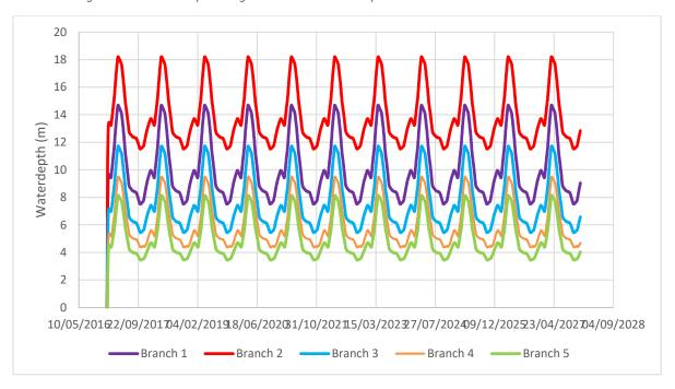
Figure B. 5.3 Water depth in Tigris when all nodes are open and branch 1 and 2 are closed
