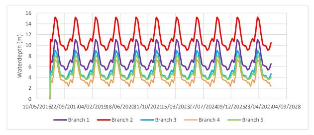
Figure B. 6.4 Water depth in Euphrates when all nodes are open and branch 5 closed
