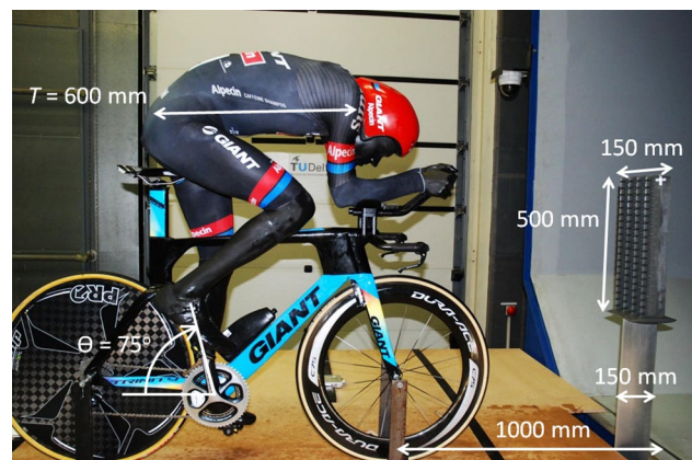
Fig. 2 Wind tunnel model and PIV seeding system
