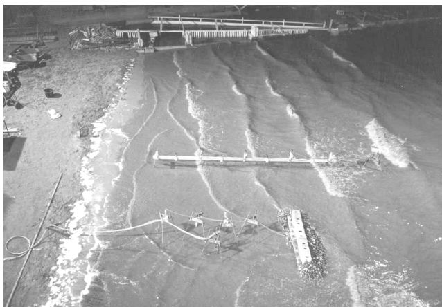
Figure 1 View of the detached offshore breakwater test with measurement tripods, beam with fixed instruments. Inflow is at the far end.
