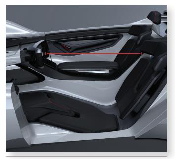
FIGURE 6.2 Steering wheel distance
