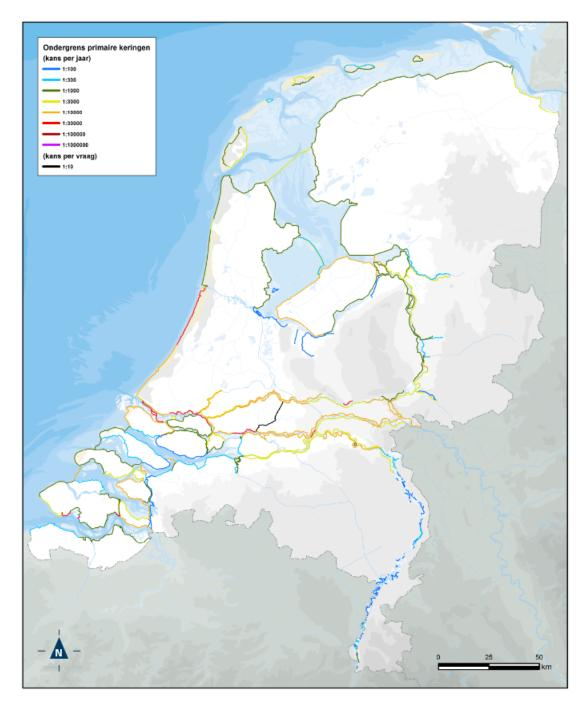
Figure 4.2: The maximum acceptable failure probability per dike trajectorie (source: [22])
