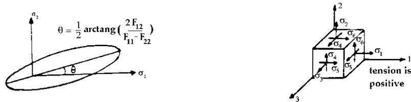
Figure 11.1. Failure ellipsoid and definition of positive stresses.
