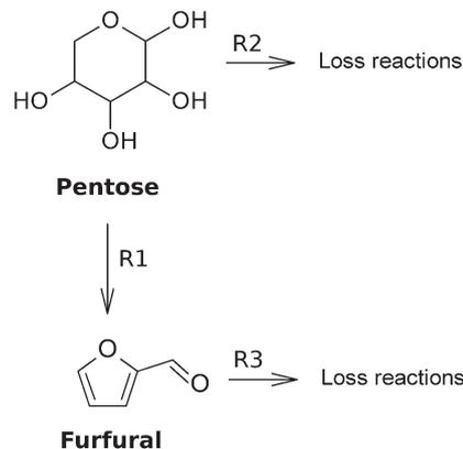
Fig. 9 Most employed reaction mechanism for the dehydration of a pentose towards furfural.
