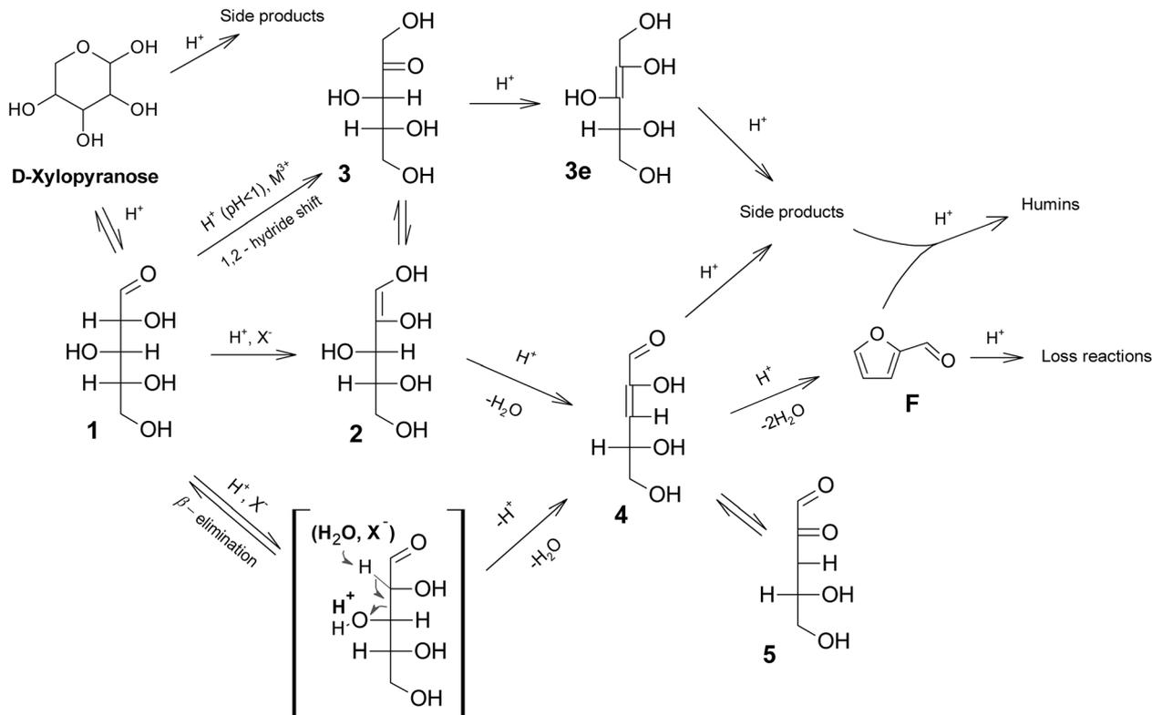
Fig. 6 Plausible mechanism of xylose reaction to furfural in acid media. X<sup>-</sup> indicates halides ions, and M<sup>3+</sup> indicates metal cations.
