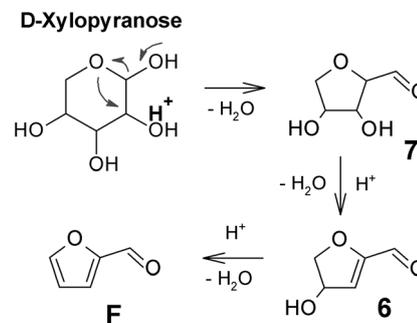
Fig. 4 Xylose dehydration mechanism *via* cyclic intermediates.<sup>27–30</sup>
