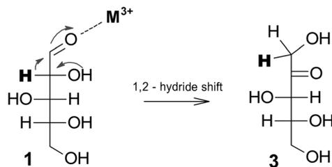
Fig. 7 Proposed isomerization of xylose via 1,2-hydride shift.<sup>32</sup>
