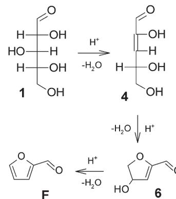
Fig. 3 Xylose dehydration mechanism *via*  $\beta$ -elimination.<sup>25,26</sup>
