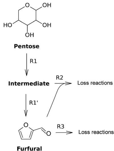
**Fig. 10** Reaction mechanism for the dehydration of a pentose towards furfural including a combined intermediate and furfural ('Kondensation') reaction.<sup>82</sup>
