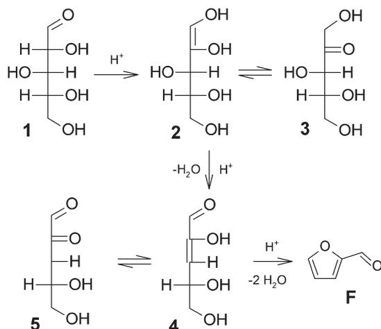
Fig. 2 Xylose dehydration mechanism *via* enolization.<sup>23,24</sup>
