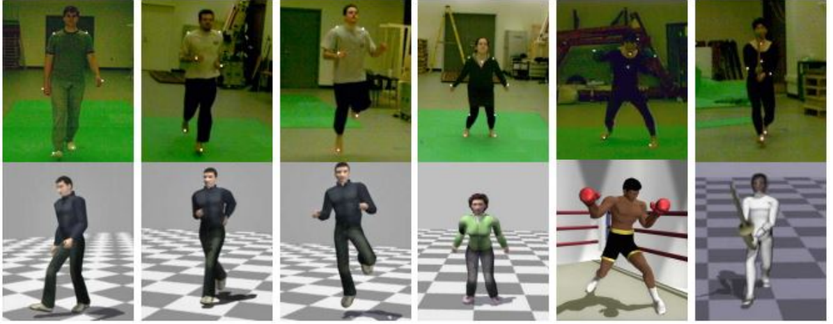
Figure 2.2: : Users wearing a few retro-reflective markers control the full-body motion of avatars by acting out the motion in front of two synchronized cameras. From left to right: walking, running, hopping, jumping, boxing, and Kendo (Japanese sword art).
