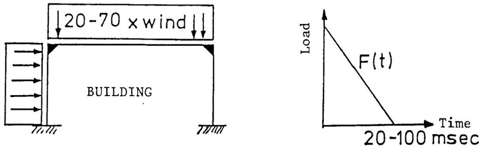
Fig. 4.1 Loading on explosion-resistant buildings for monitoring equipment.
