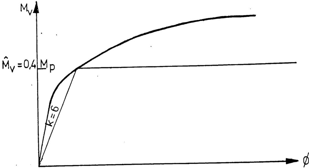
Fig. 1.11: Example of a moment-rotation characteristic and the calculated bilinear moment-rotation characteristic.
