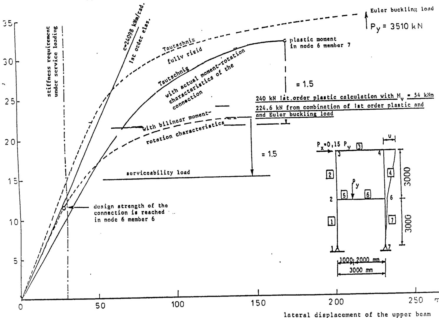
Fig. 1.6: Summary of force-displacement curves for an unbraced frame calculated by various methods (see Appendix A);
