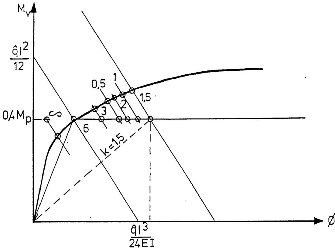
Fig. 1.13a: Intersections of the beam lines with the experimentally determined moment-rotation characteristic and the calculated moment-rotation characteristic.  $\hat{q}$  has been calculated on the basis of elastic theory with the aid of the diagram given below, for  $\hat{M}_v = 0.4 M_p$  and  $k=6$ .
