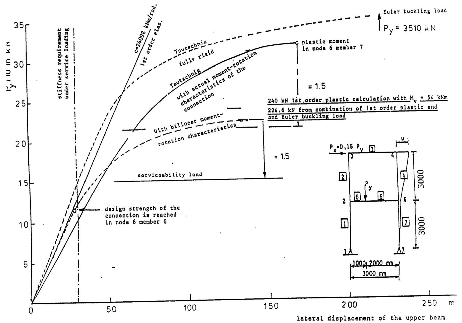
Fig. 1.3: Influence of the stiffness and strength of the connections on the force-displacement behaviour of an unbraced frame. (zie Fig. 1.6).
