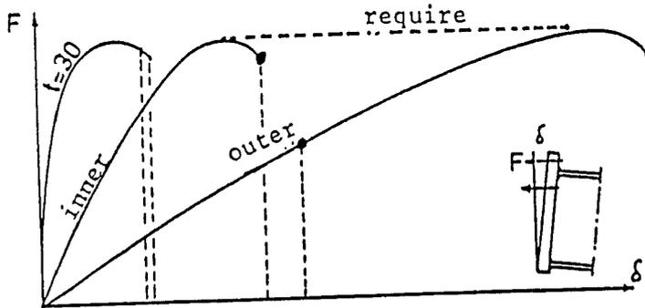
Fig. 3.9: Comparison of the force-displacement diagrams of "inner" and "outer" parts.
