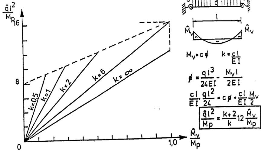
Fig. 1.8 : Design strength of a beam in a braced frame as a function of the joint strength and the ratio between joint stiffness and beam stiffness,  $k = \frac{cl}{EI}$ , in the case of comparatively stiff joints.
