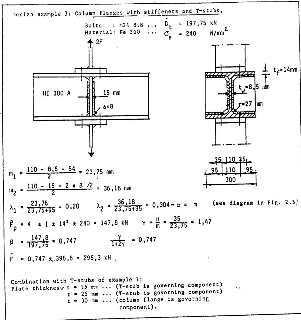
Fig. 2.4: Design example for column with stiffeners.
