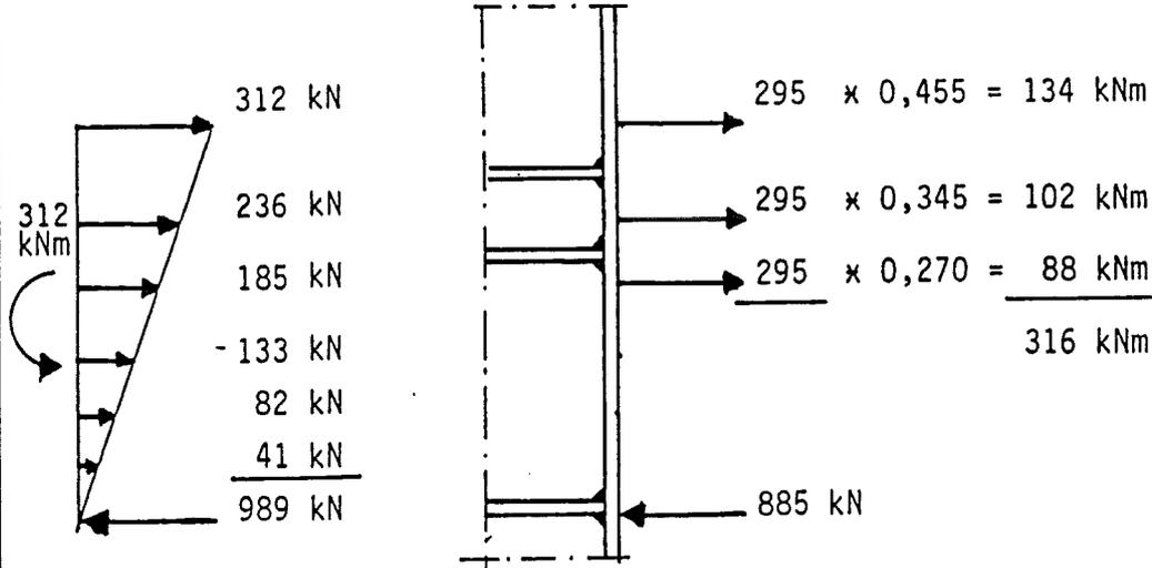
With end plate and column flange assumed to be infinitely stiff.
