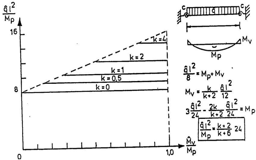
Fig. 1.9 : Design strength of a beam in a braced frame as a function of the joint strength and the ratio between joint stiffness and beam stiffness,  $k = \frac{cl}{EI}$  in the case of joints with comparatively low stiffness.
