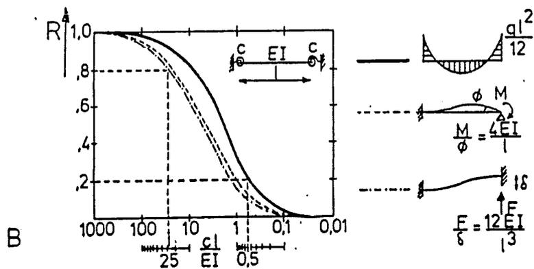
Fig. 1.7 : Relations between loads and deformations as a function of the ratio joint/stiffness/member stiffness and the belonging reduction factor
