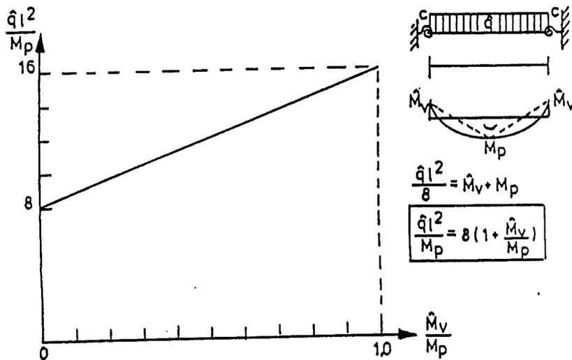
Fig. 1.10 : Design strength of a beam in a braced frame as a function of the joint strength, calculated according to the theory of plasticity.
