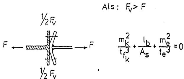
C. Prestressing the bolts with a force larger than the tensile force has the effect that the bending of the end plate and column flange can be neglected, provided that the contact pressure acts in alignment with the column web and beam web.
