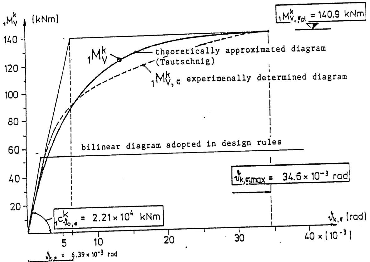
Fig. A.2: Moment-rotation diagrams of the connections to which the calculations relate.
