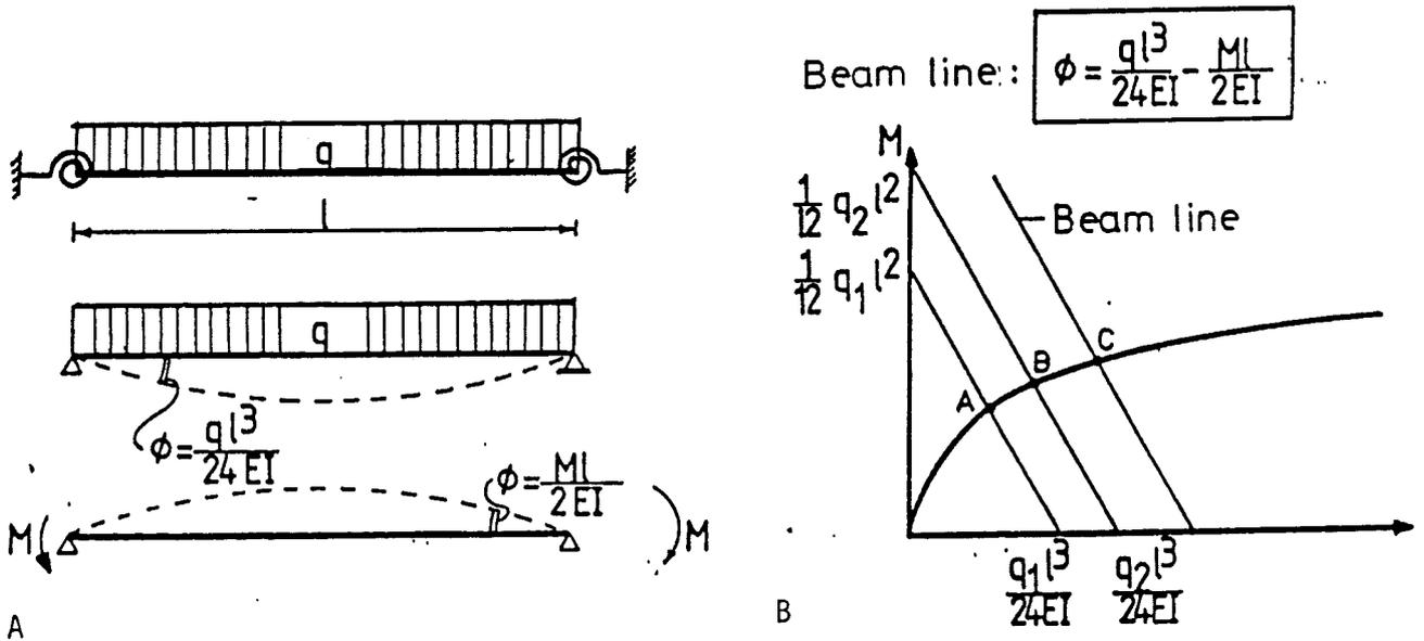
Fig. 1.12: The actual situation in the connection is determined by the intersection of the beam line with the experimentally determined moment-rotation characteristic of the connection
