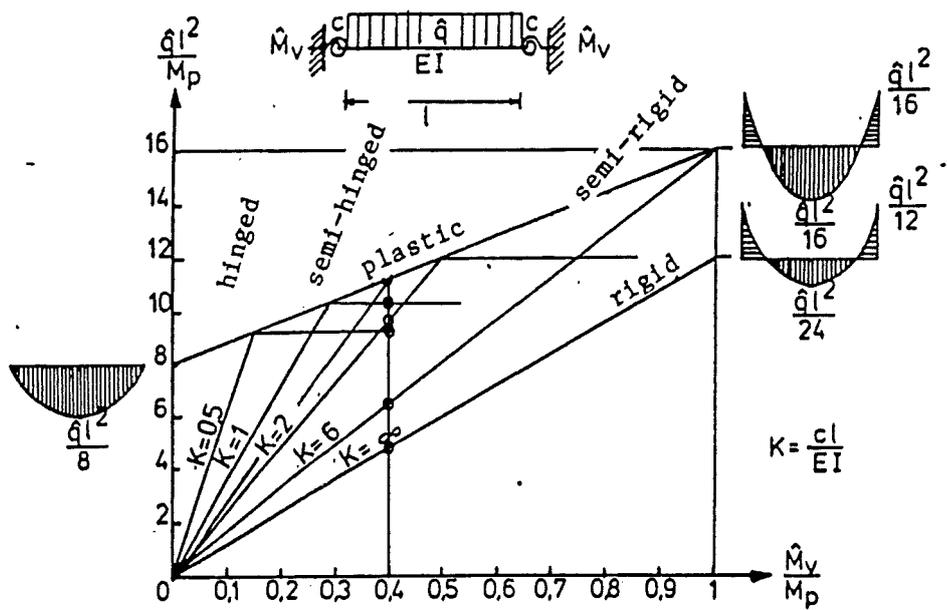
Fig. 1.13b: Relations between loading and the strength and stiffness of the connections and the beam in a braced frame;
