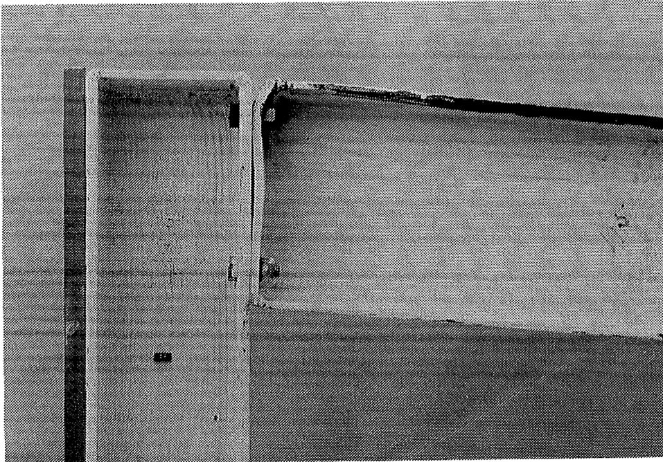
Rapidly loaded knee connection with end plate thickness  $t = 12$  mm. Failure governed by end plate.
