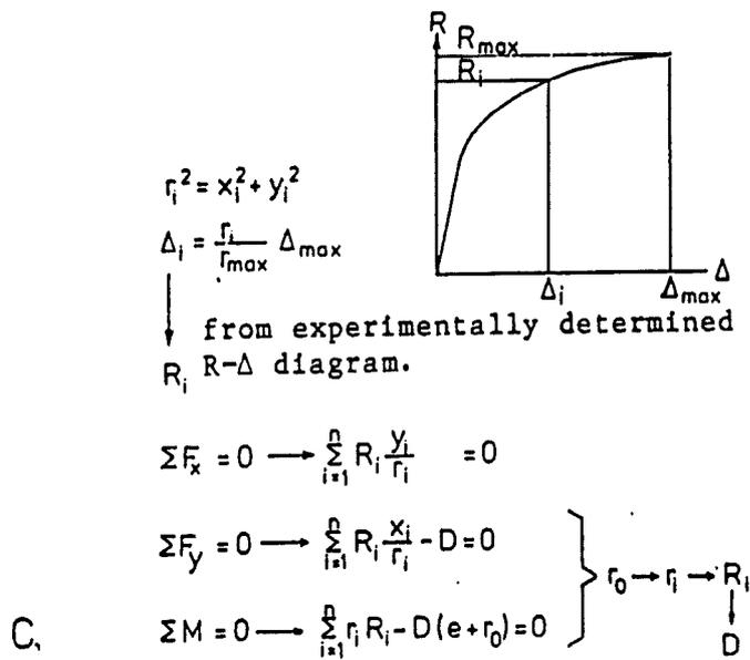
Fig. 3.2: Elasto-plastic method of analysis for angle cleats on web of beam.
