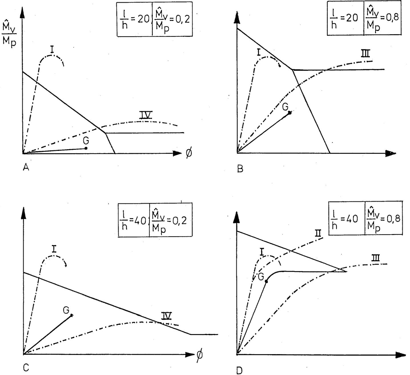
Fig. 1.16; Examples of minimum requirements and moment-rotation characteristics which are and are not satisfactory.
