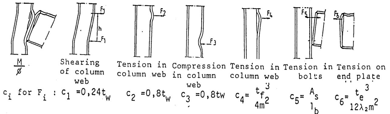
The deformation on the tension side is determined by one bolt row. The effect of the other bolt row is taken into account by multiplying by the quotient of the design strengths of the actual connection and the notational connection with one bolt row.
