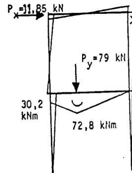
A linear moment-rotation diagram,  $c = 24098 \text{ kNm/rad}$ . no reduction due to design-strength of connection.
