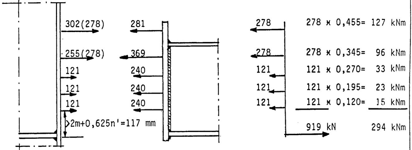
Column flanges without stiffeners on tension side (see ex. 3 and 9)
