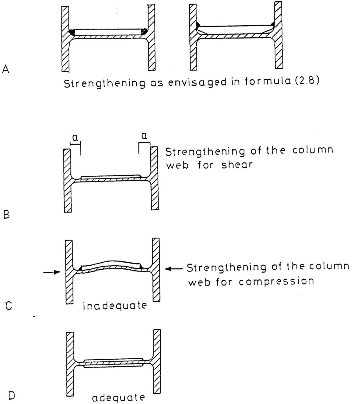
Fig. 2.27: Strengthening of column web with thickening plates.
