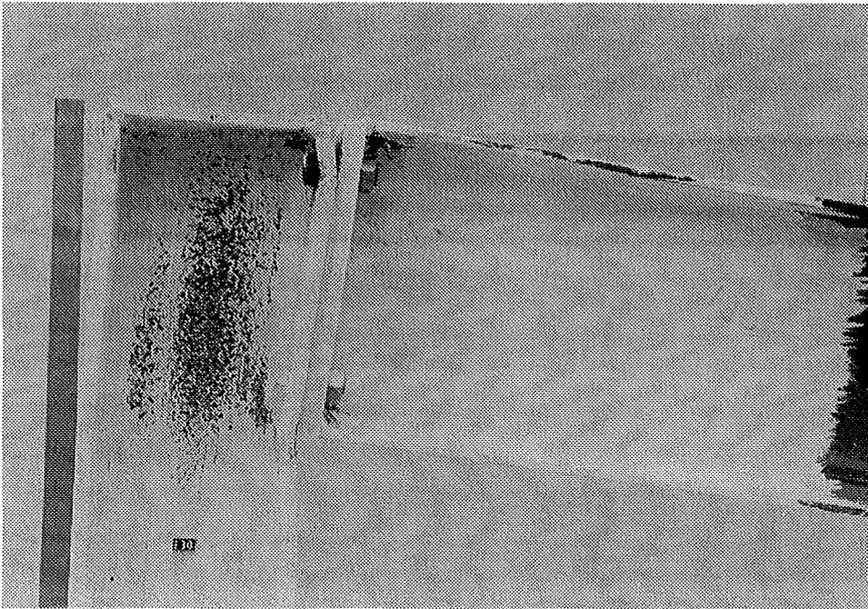
Rapidly loaded knee connection with end plate thickness  $t = 20$  mm. Failure governed by shearing of column web.
