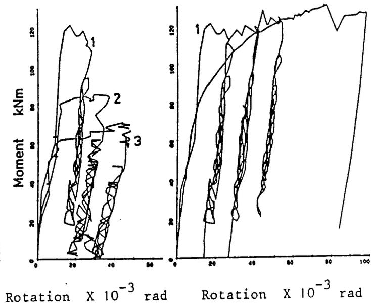
Fig 4.5. Moment-rotation characteristics of knee connections that were tested.
