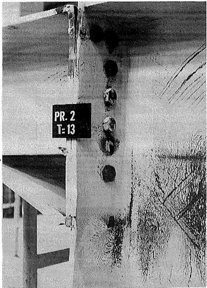
Fig. 2.9: A yield line pattern first develops around the bolt which is located nearest to the tension flange of the beam and the beam web.
