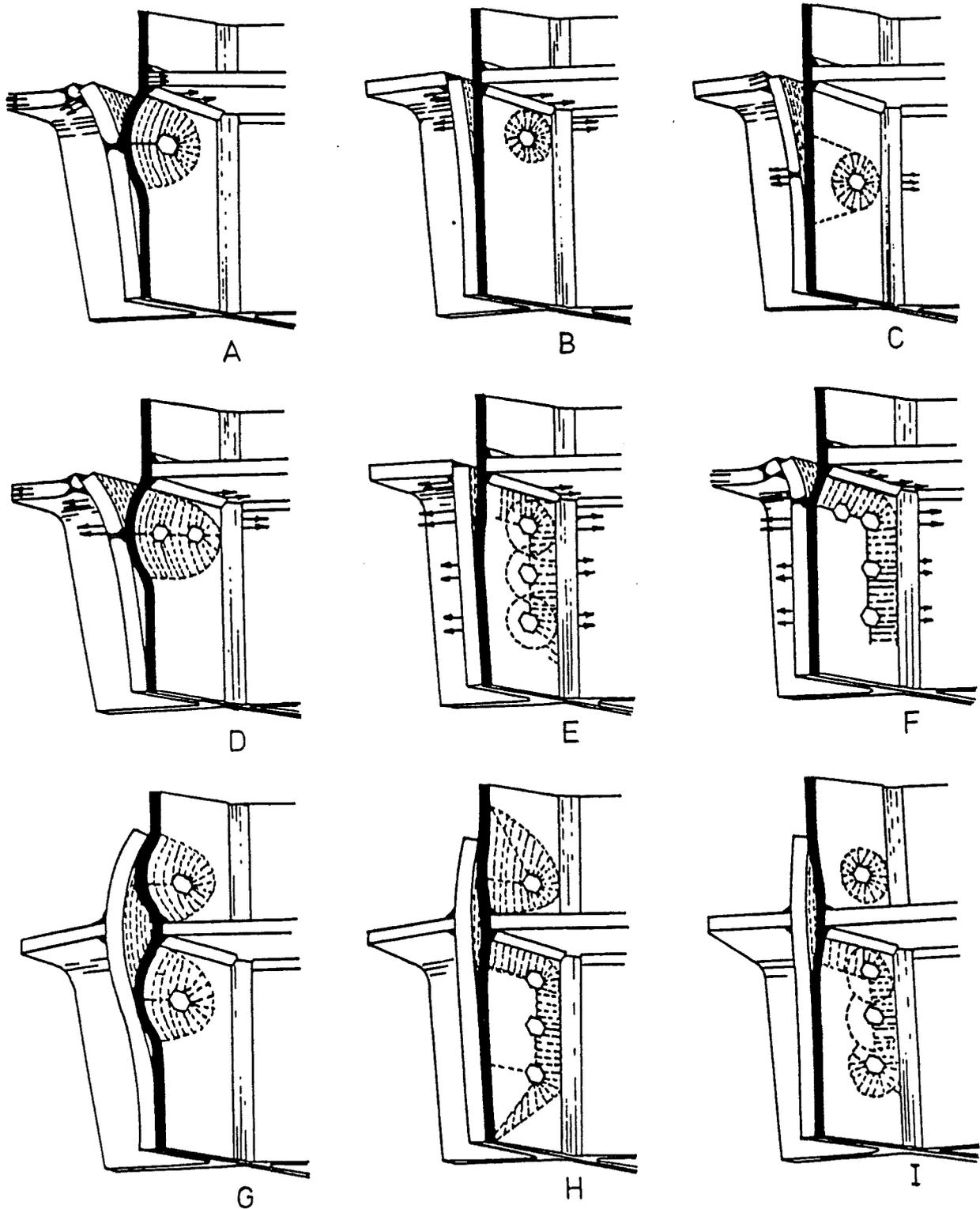
Fig. 2.10: The effectiveness of added bolts depends on the yield line pattern formed by the first bolt.
