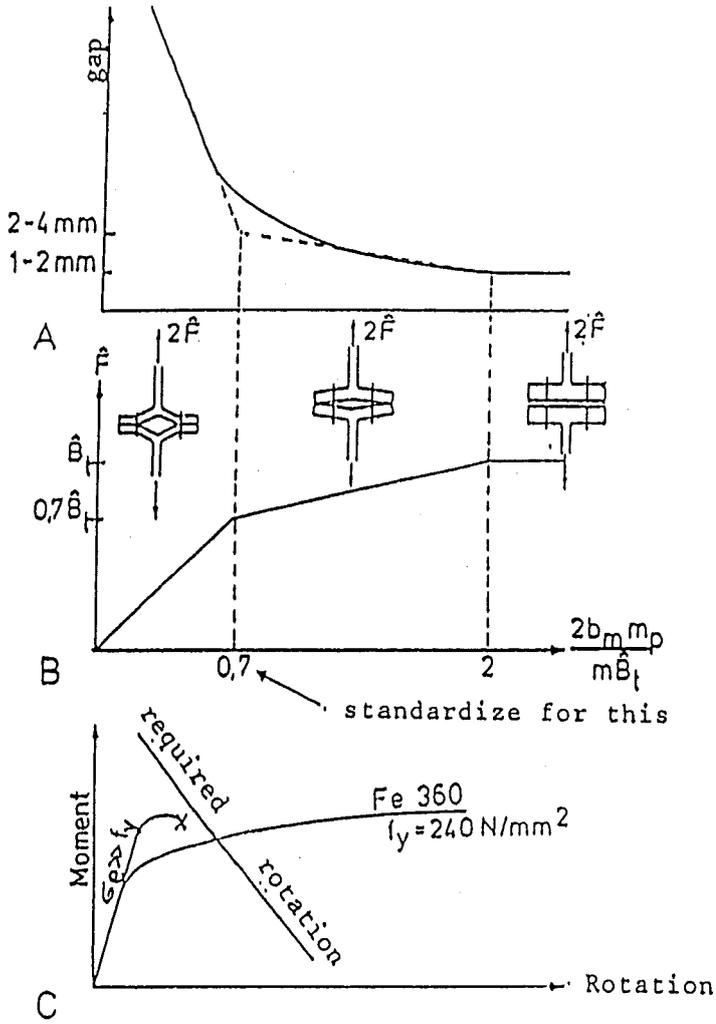
Fig. 3.5: Basis for standardization of end plates  $\beta = 0.7$
