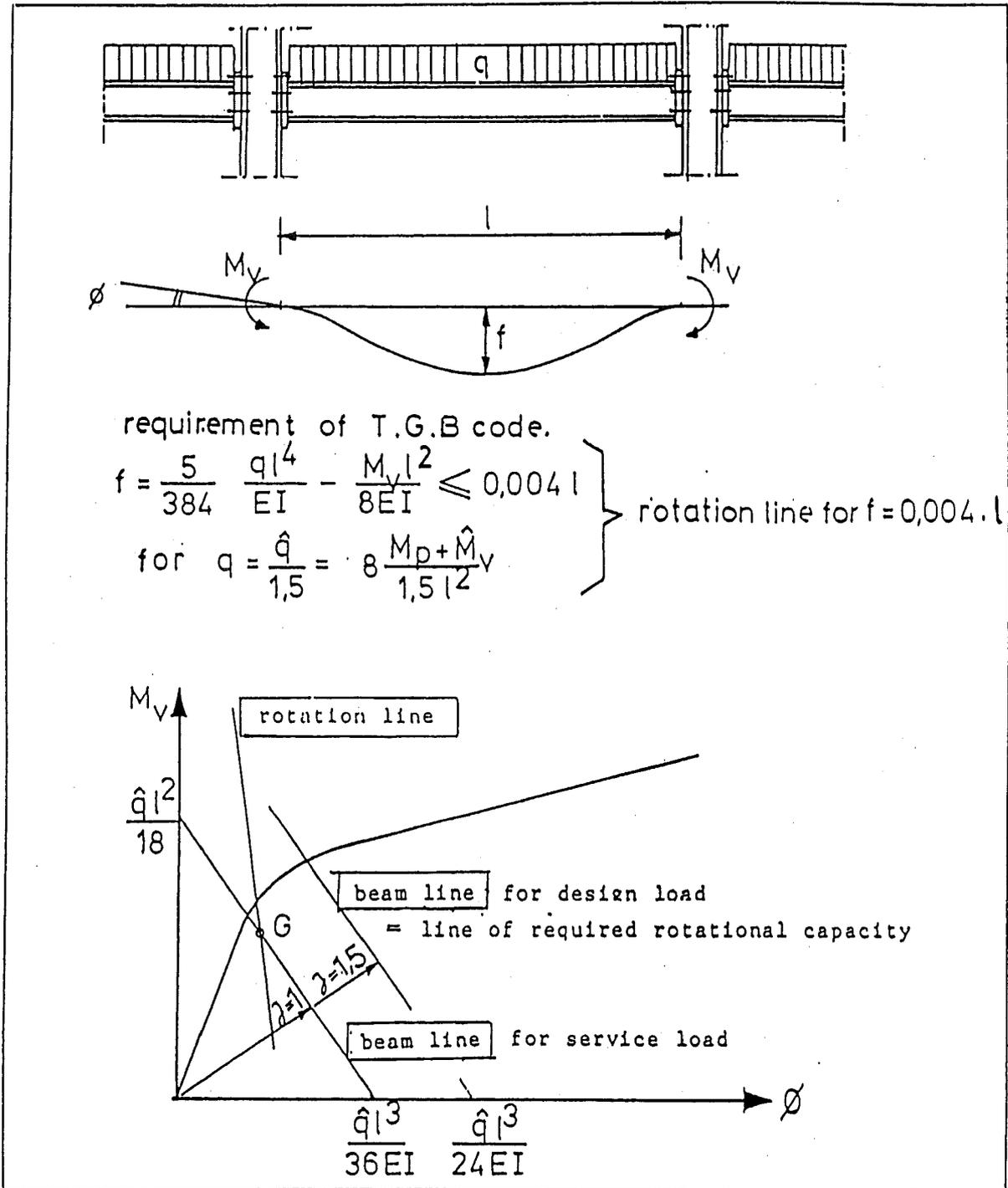
Fig. 1.14: The requirement of sufficient stiffness is represented by point G in the moment-rotation diagram;
