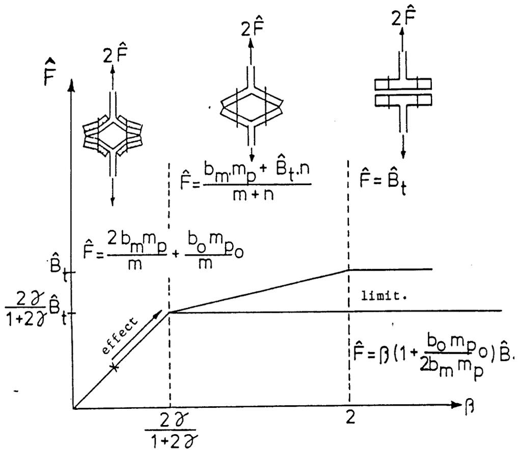
Fig. 2.26: Effect of packing plates.
