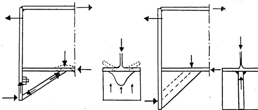
B. In the case of connections without stiffeners the haunch without flange is to be recommended because the forces must be transmitted into the webs of the column and beam.
