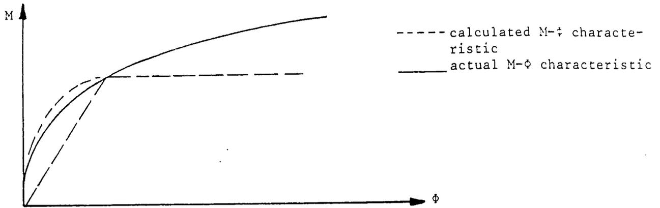
Fig. 1.4a: Moment-rotation characteristic of the structural connections.
