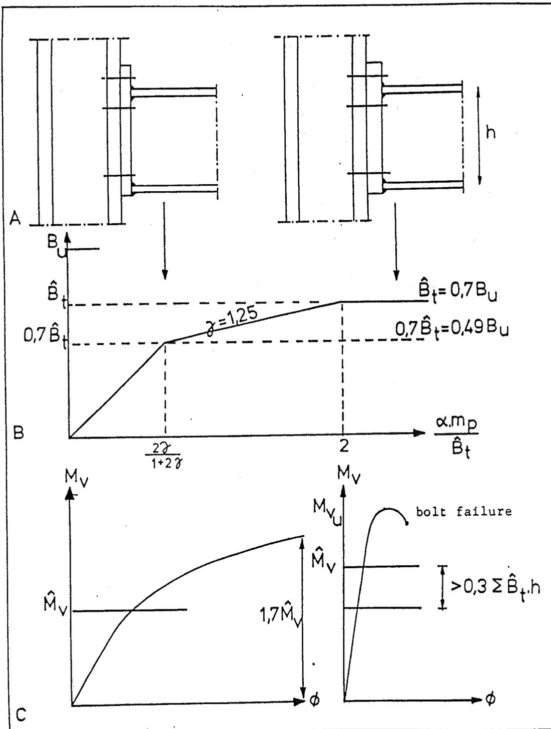
Fig. 2.20: Comparison of the behaviour of connections with and without deformation capacity, from which it appears that no extra bolt force capacity is necessary.
