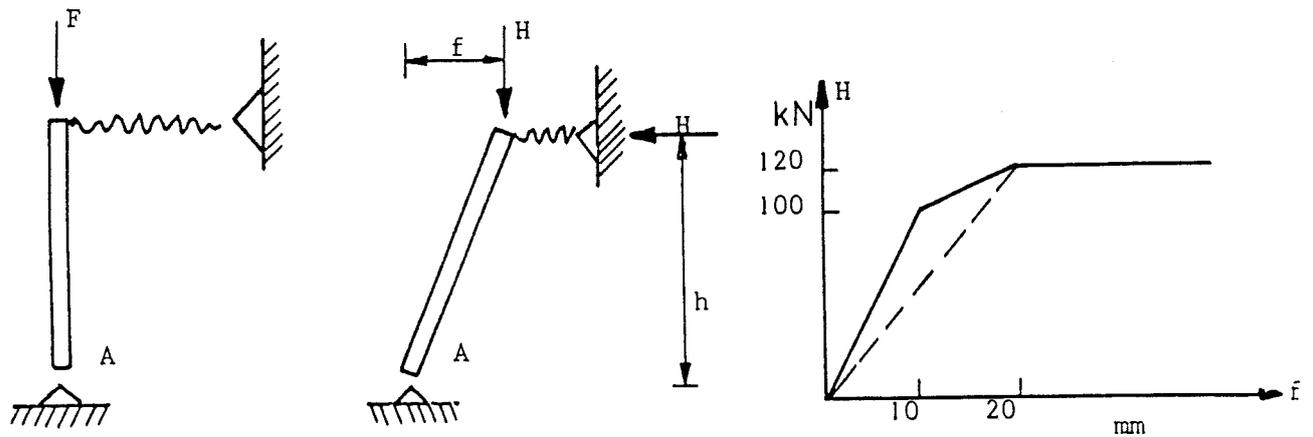
Fig. 1.4b: Schematization of the structure with spring characteristic for lateral displacement.
