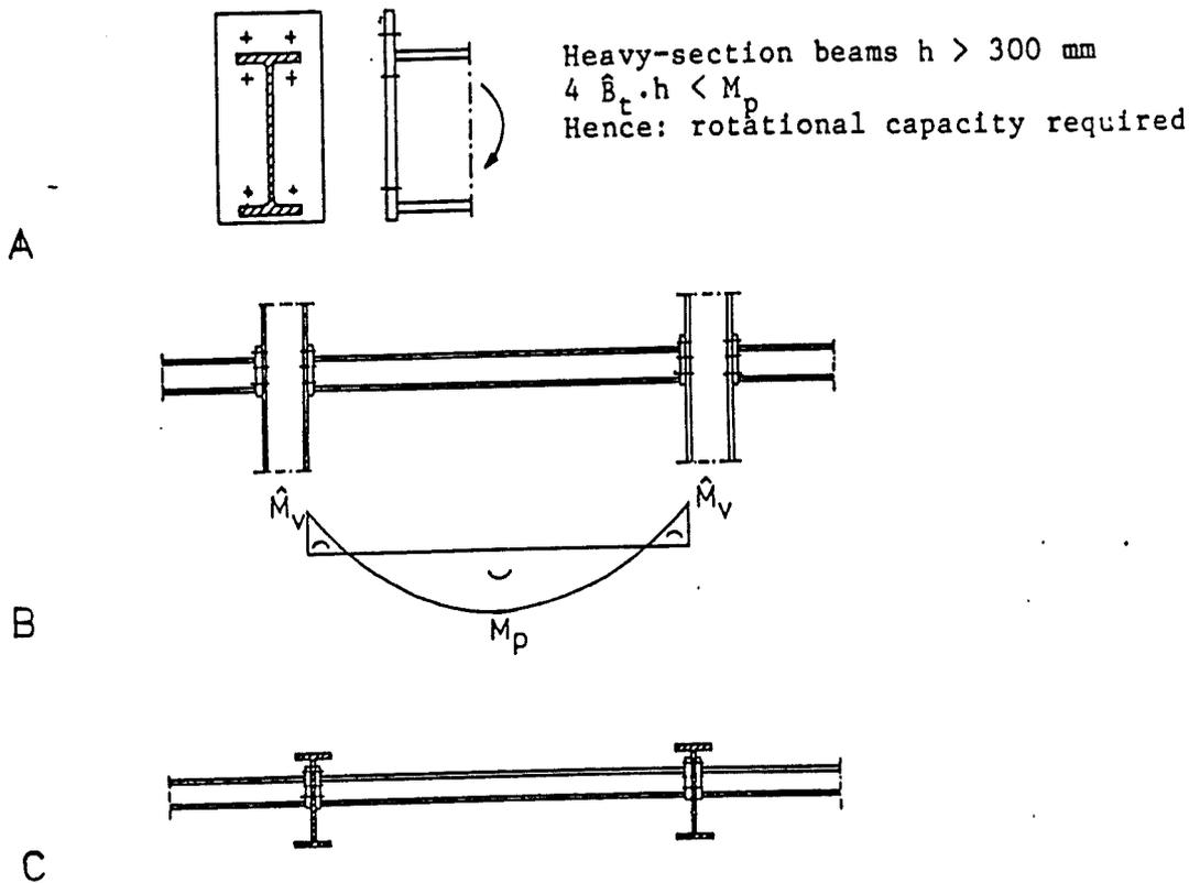
Fig. 3.4: Standardized end plates should provide deformation capacity if they are not designed for full-strength connection.
