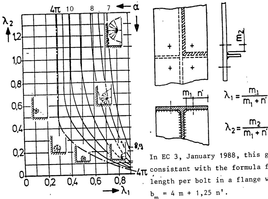
Fig. 2.5: Diagram for determining the design strength of an end plate or column flange with stiffener loaded by a bolt.
