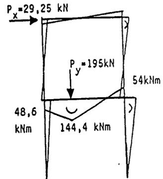
A with fully rigid connections according to Tautschnig.
