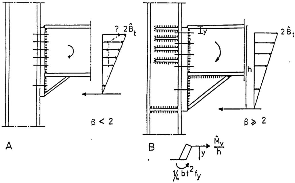
Fig. 2.17: Possible distributions of forces in the connections depend on the plate strength/bolt strength ratio  $\beta$ .
