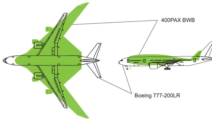
Figure 8. Comparison between BWB and Boeing 777-200LR.
