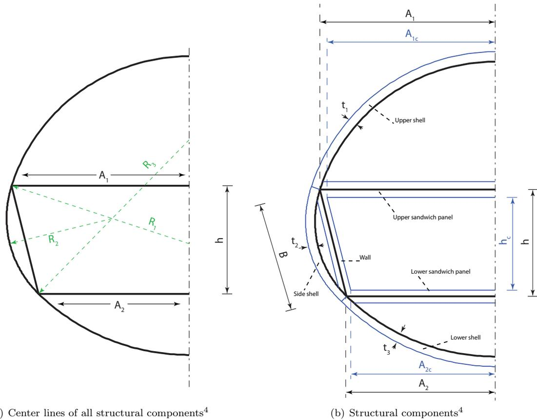
(a) Center lines of all structural components<sup>4</sup>
