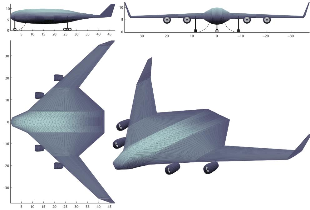
**Figure 6. Three-view of 400-passenger BWB (dimensions in meters).**
