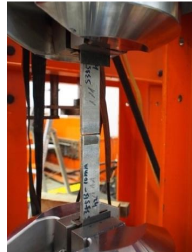
FIGURE 4: A FAILED FATIGUE TEST SPECIMEN IN THE HYDRAULIC TEST RIG
