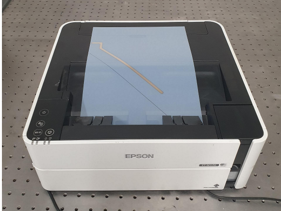
FIGURE 2.4: Printer EcoTank ET-M1170 and a PVC sheet with PA printed on.
