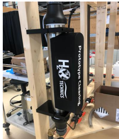
Figure 2. Ultrasound disinfection device provided by H2O TECHNICS
