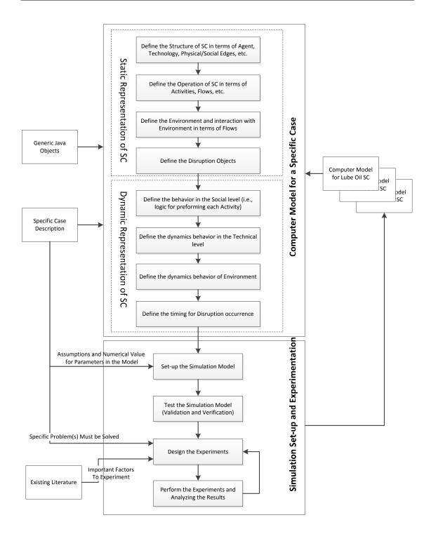
Figure 7.34. Process for developing models for other case studies
