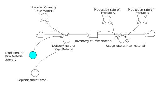
Figure 5.9. Stock-flow diagram for inventory management in a plant (Mussa, 2009)
