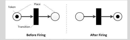
Figure 4.4. The main elements of PN model
