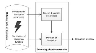
Figure 7.24. Procedure for scenario generation
