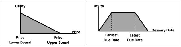
Figure 6.16. Examples of evaluation function for price and delivery time
