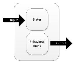
Figure 5.11. A simple structure for an Agent in ABM (after Nikolic, 2009)
