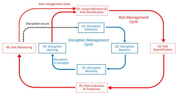
Figure 3.3. The overall structure of InForMDRiSC
