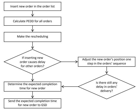
Figure 7.7. Flowchart to describe the logic behind sendOrderProcessingInfo Activity
