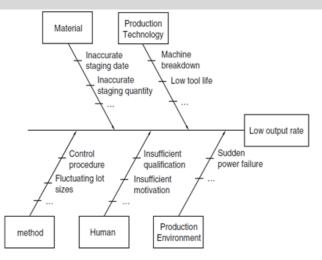
Figure 4.2. An example of Ishikawa diagram for supply chain risk identification, from Wiendahl et al. (2008)
