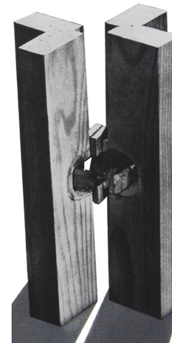
X-wedge connection (Lowry, 2008, pp. 80-87)
