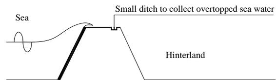
Figure 5: One dike system with small overtopping
