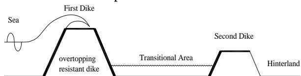
Figure 6: Using two dikes system with medium large overtopping
