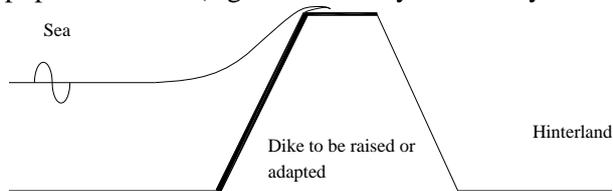
Figure 4: One dike system without overtopping
