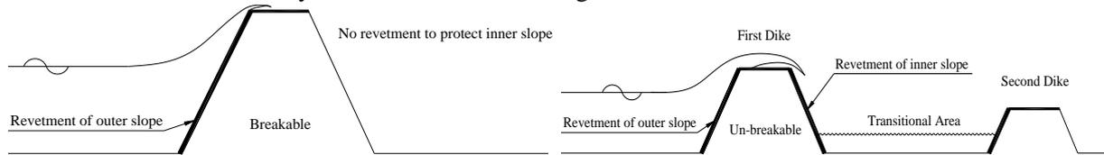
Figure 1: Cross-section of one defensive line
