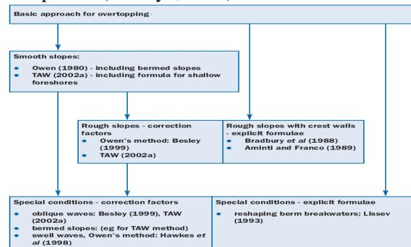
Figure 3: Calculation method for wave overtopping (CIRIA/C683, 2007)
