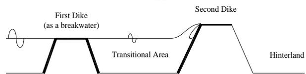
Figure 7: Using two dikes system with large overtopping
