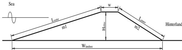
Figure 9: Specific parameters of one dike line system
