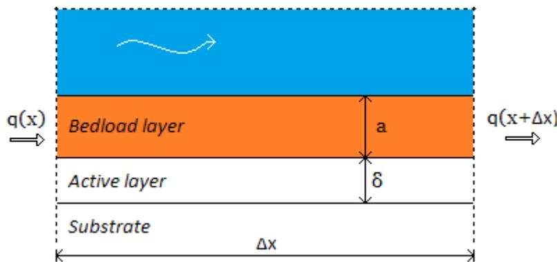
Figure 1 - Schematisation bedload transport
