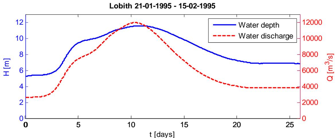
Figure 7 - Flow depth (measured hourly) and discharge (measured daily) in Lobith
