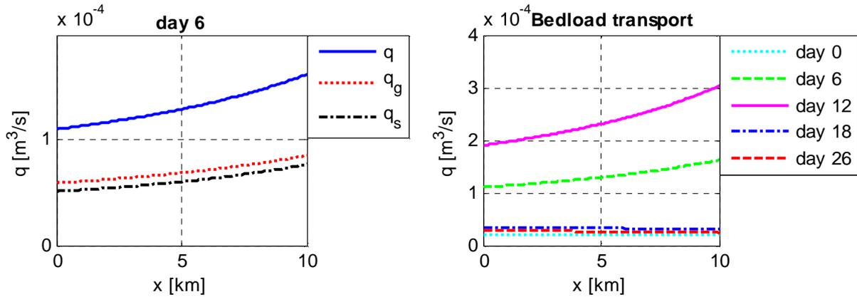
Figure 10 - Left: division corresponding to the separate fractions on day 6. Right: total bedload transport.
