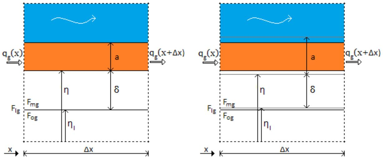
Figure 20 - Left: active plus bedload layer model, right: same model at another moment in time
