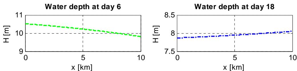
Figure 9 - Detailed flow depth variation for day 6 (M2 curve) and day 18 (M1 curve)
