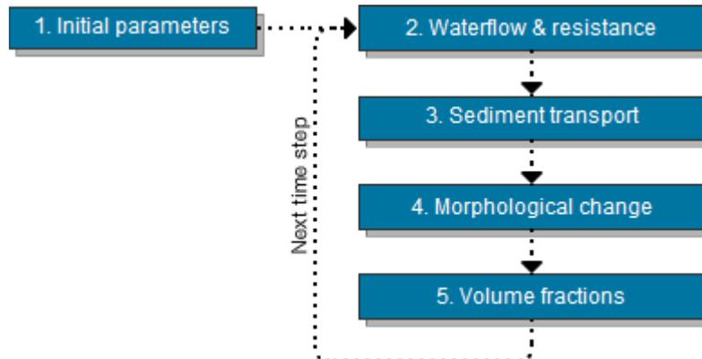
Figure 5 - Approach sand-gravel sediment model
