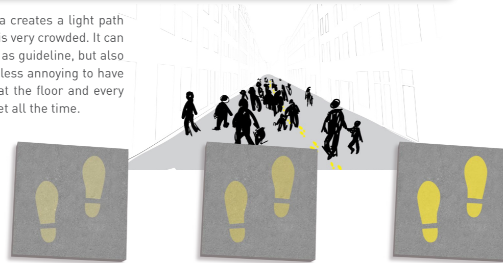
No people walk on tile Some people walk on tile Many people walk on tile
