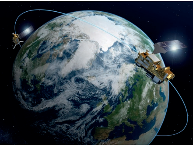
▲ Figure 2, After completion Sentinel-2A and 2B will operate in the same sun-synchronous orbit 180° apart (Courtesy: ESA).
