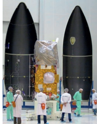
▼ After encapsulation in the Vega rocket fairing (left) Sentinel-2A is transported to the launch zone (Courtesy: ESA).
