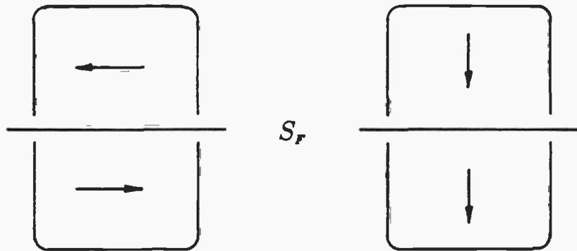
Figure 3-1. When  $t \rightarrow 0$ ,  $G(\vec{x}; \vec{\xi}, t) \rightarrow \frac{1}{R} - \frac{1}{R'}$ . In this limit,  $\phi^{(1)}(\vec{x}, t) = 0$  on the free surface, as in the frequency-domain limit of  $\omega \rightarrow \infty$ . The potential is anti-symmetric with respect to the free surface. This limit defines the 'pressure-release' problem. For heave, pitch, and roll this is also the infinite-fluid problem.
