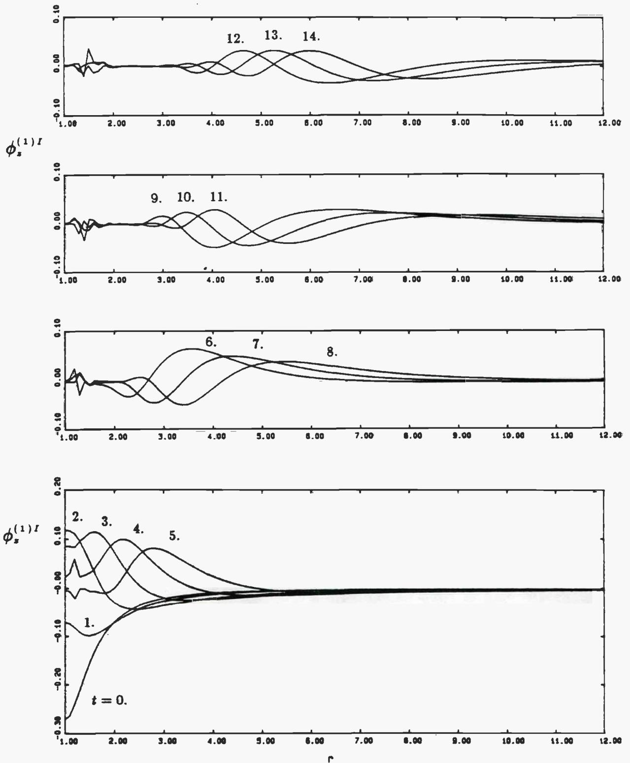
Figure 9-5. The heaving cylinder.  $\phi_z^{(1)I}(\vec{r}, t)$  on the free surface.  $\Delta t = 0.1$ , panelling: 24x36 (bottom & side x azimuthal). The region close to the body (Figure 9-3) has been interpolated through.
