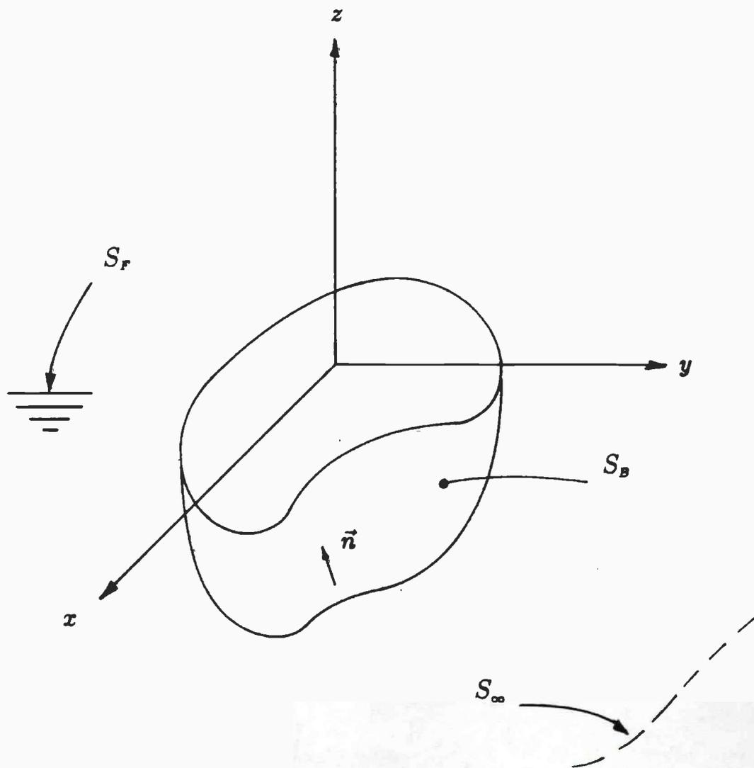
**Figure 2-1.** The coordinate system for the transient radiation problem. Surface identifications apply to the initial positions of the surfaces as understood in the first- and second-order problems.
