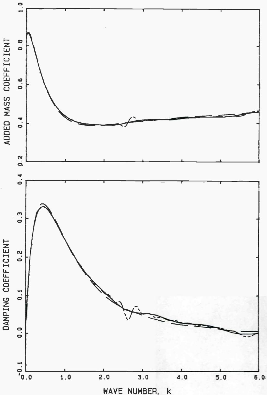
Figure 6-6. Heaving hemisphere; 64 panels,  $\Delta t = 0.2$ , truncated at  $t = 20$ . — ; 64 panels,  $\Delta t = 0.2$ , truncated at  $t = 50$ . - - - ; 256 panels,  $\Delta t = 0.1$ , truncated at  $t = 20$ . — — . Coefficients are non-dimensionalized by the displaced fluid mass.
