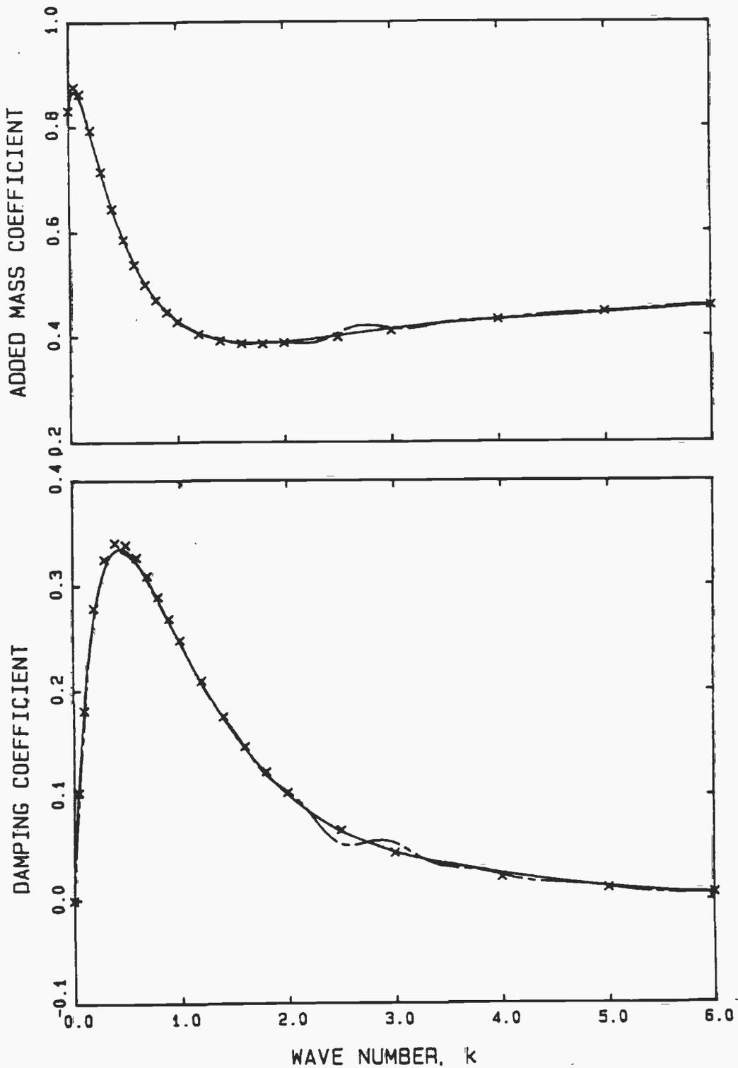
Figure 6-9. Heaving hemisphere. Transform of the patched functions of Figure 7 (numerical portion for 100 cosine distributed panels,  $\Delta t = 0.2$ ) truncated at  $t = 30$ , ———; the same model without patching truncated at  $t = 30$ , - - -. Results from Hulme (1982)  $\times$ . Coefficients are non-dimensionalized by the displaced fluid mass.
