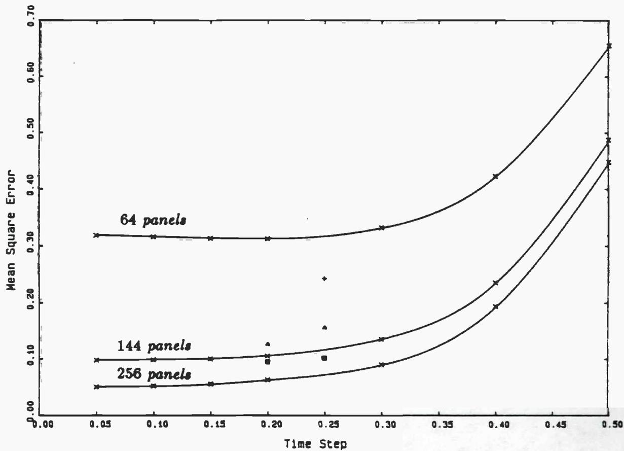
Figure 4-4. Heaving hemisphere. Mean square error in the impulse response function (compared to a 4608-panel model with  $\Delta t = 0.05$ ). Solid lines are splines through the marked data-points for regularly distributed panel models. Cosine distributed panel models are marked: 64 panels + , 100 panels ▲ , 144 panels □ .
