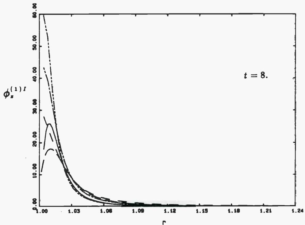
Figure 9-3 cont. The heaving cylinder.  $\phi_z^{(1)H}(\vec{r}, t)$  and  $\phi_z^{(1)I}(\vec{r}, t)$  on the free surface close to the body ( $r=1.0$ ). All results are for  $\Delta t = 0.1$ . Panelling: 16x16 — — ; 16x24 — — — ; 24x24 — - - - ; 24x36 — — — — ; and 36x36 — - - - - ; (bottom & side x azimuthal).
