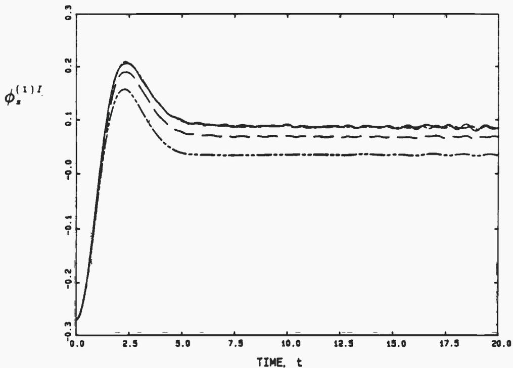
Figure 9-2 cont. The heaving cylinder.  $\phi_s^{(1)I}(\vec{r}, t)$  at the body and free-surface intersection. All results are for  $\Delta t = 0.1$ . Panelling: 24x36 ——— ; 24x72 — — — ; 24x144 — - - - ; and 36x54 — · · · ; (bottom & side x azimuthal).
