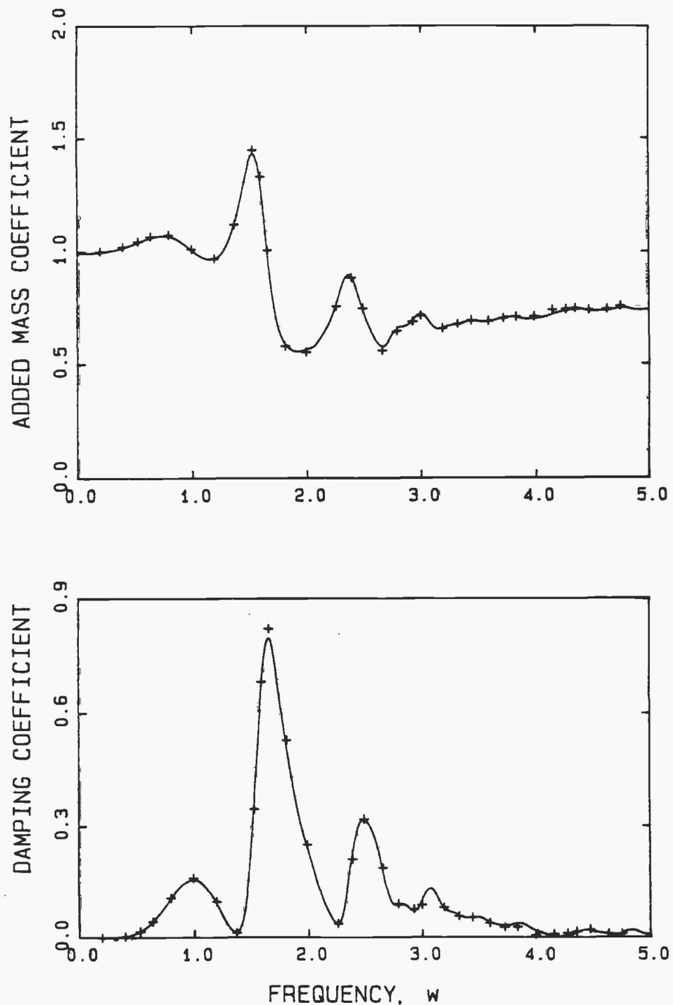
**Figure 6-13.** The Tension Leg Platform in surge. The Fourier transform of impulse response function of Figure 6-12. 820 panels,  $\Delta t = 0.1$ , truncated at  $t = 35$ . — ; Frequency domain results from WAMIT, 1696 panels, + . Coefficients are non-dimensionalized by acceleration due to gravity, fluid density and body half-breadth set equal to one.
