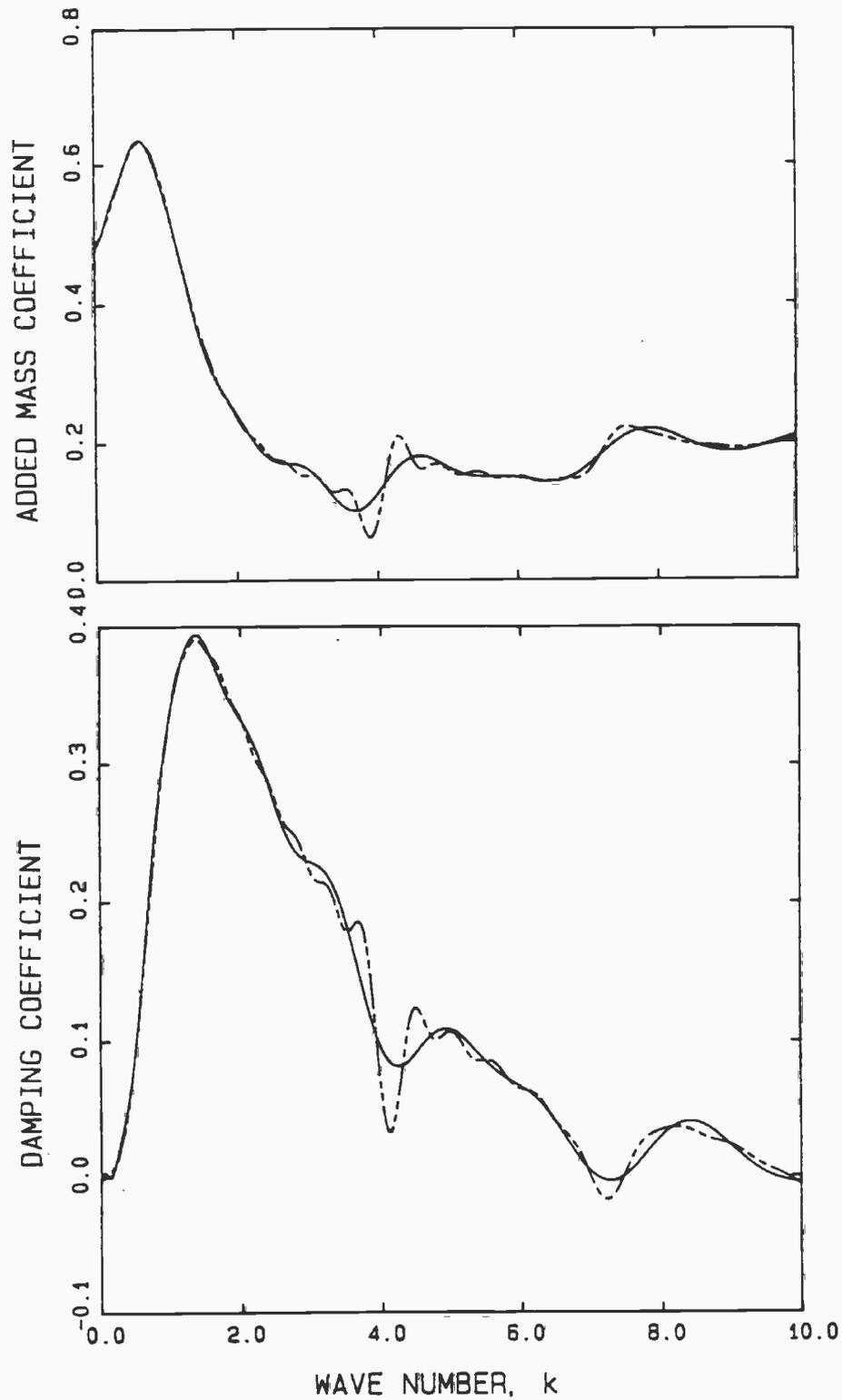
**Figure 6-2.** Swaying hemisphere; 64 panels,  $\Delta t = 0.2$ , truncated at  $t = 20$ . — ; 64 panels,  $\Delta t = 0.2$ , truncated at  $t = 50$ . - - -. Coefficients are non-dimensionalized by the displaced fluid mass.
