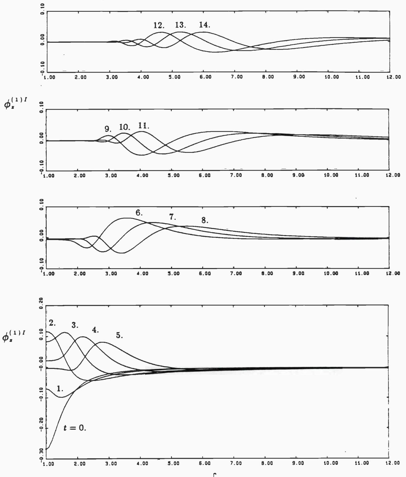
Figure 10-3. The heaving cylinder.  $\phi_z^{(1)I}(\bar{r}, t)$  on the free surface.  $\Delta t = 0.1$ ; panelling on the body: 24x36 (bottom & side x azimuthal); the infinite cylinder truncated at  $z = -6.0$ , discretized by 48 points. Compare with Figure 9-5.
