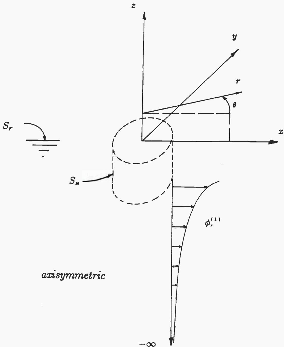
Figure 10-1. The coordinate system for the alternate method. Note that the semi-infinite cylinder, on which  $\phi_r^{(1)}(1, \theta, z)$  is specified, is an extension of the body itself.
