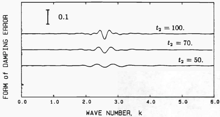
Figure 6-4 Form of the irregular frequency effect in the damping coefficient for the heaving hemisphere predicted by equation (6.2). In all cases,  $t_1 = 30$ .
