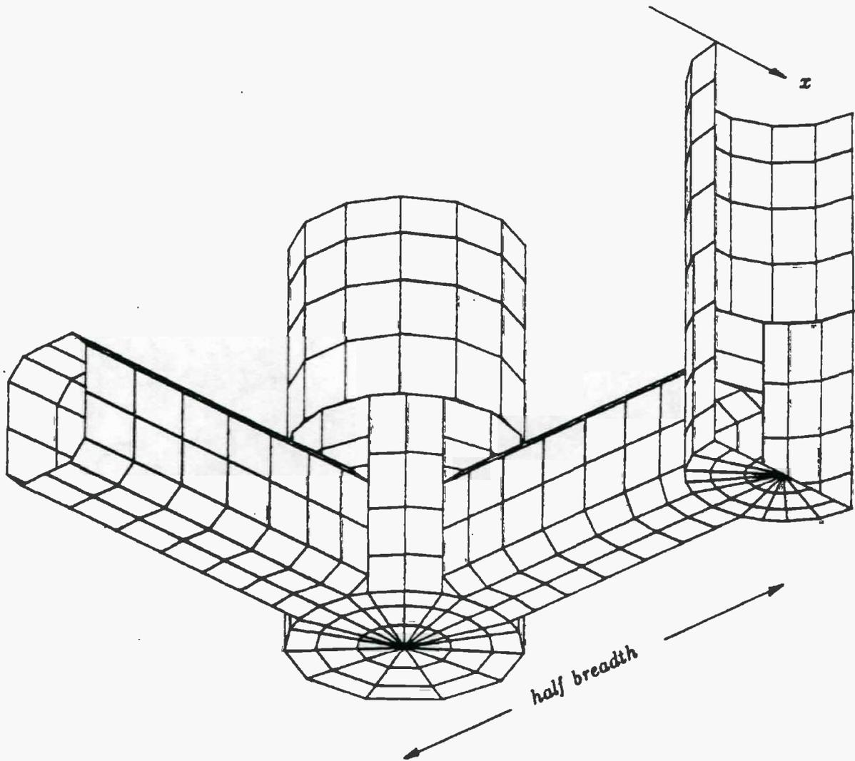
**Figure 6-11.** One quadrant of the Tension Leg Platform. The number of panels on the entire body is 1652.
