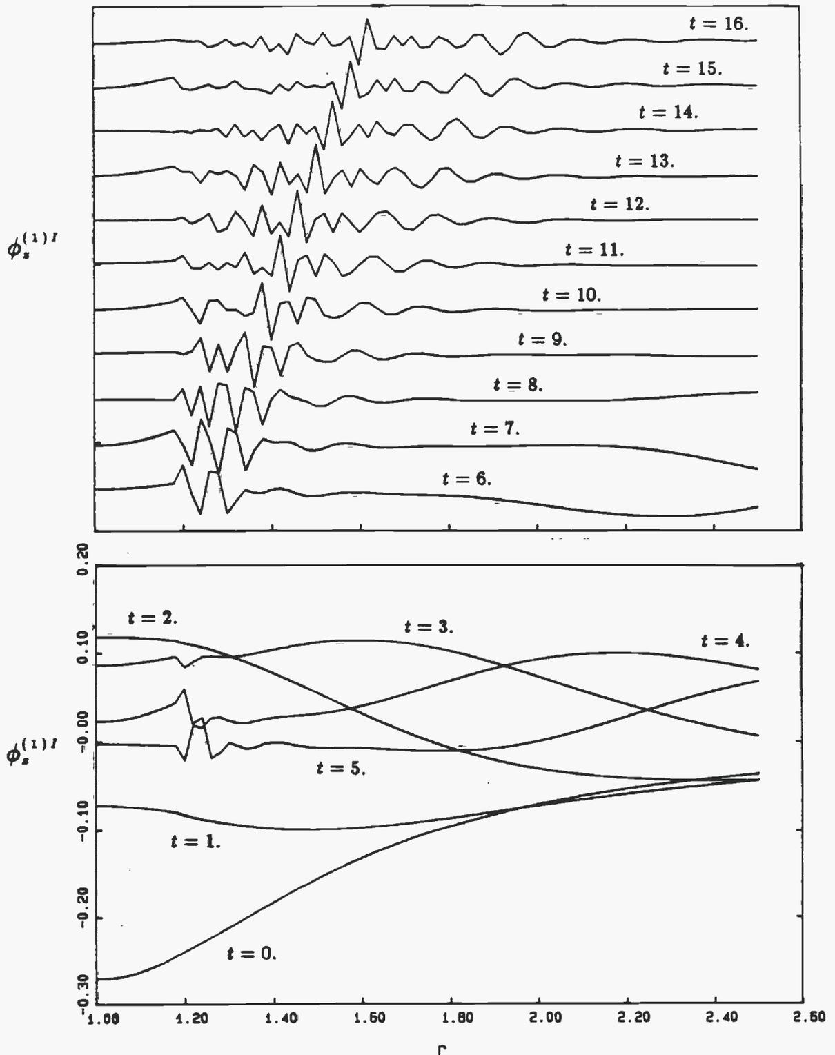
Figure 9-4. The heaving cylinder.  $\phi_s^{(1)l}(\bar{r}, t)$  on the free surface in the region of short waves.  $\Delta t = 0.1$  panelling: 24x36. The region close to the body (Figure 9-3) has been interpolated through.
