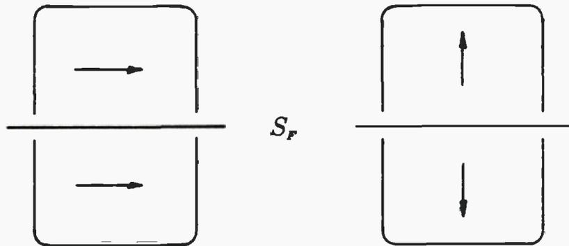
Figure 3-2. When  $t \rightarrow \infty$ ,  $G(\vec{x}; \vec{\xi}, t) \rightarrow \frac{1}{R} + \frac{1}{R'}$ . In this limit,  $\phi_s^{(1)}(\vec{x}, t) = 0$  on the free surface, as in the frequency-domain limit of  $\omega \rightarrow 0$ . The potential is symmetric with respect to the free surface. This limit defines the 'rigid-lid' problem. For surge, sway, and yaw this is also the infinite-fluid problem.
