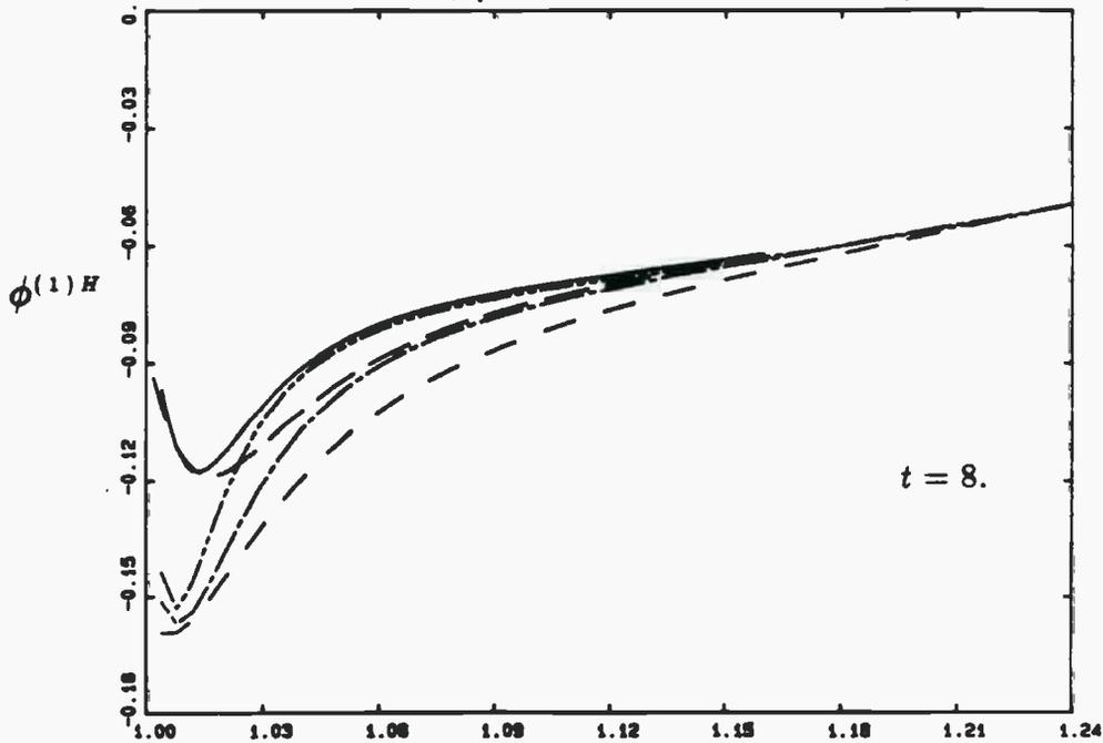
Figure 9-3. The heaving cylinder.  $\phi^{(1)H}(\vec{r}, t)$  on the free surface close to the body ( $r=1.0$ ). All results are for  $\Delta t = 0.1$ . Panelling: 16x16 — — — ; 16x24 — - - ; 24x24 — · · · ; 24x36 ——— ; and 36x36 — · · · ; (bottom & side x azimuthal).
