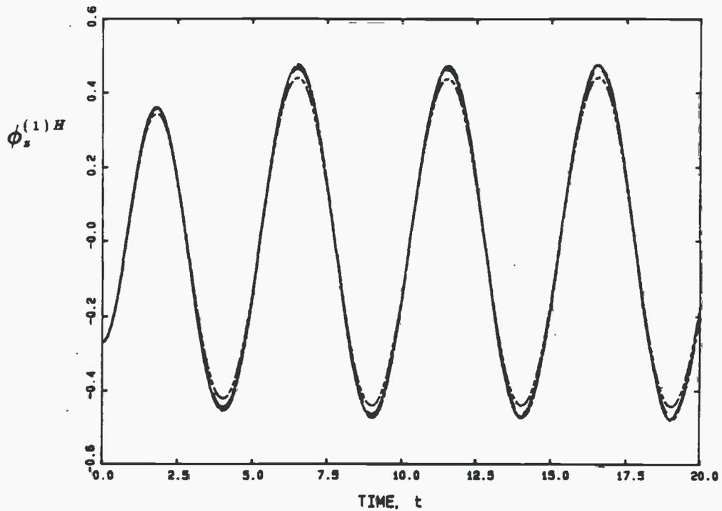
Figure 9-2. The heaving cylinder.  $\phi^{(1)H}(\vec{r}, t)$  and  $\phi_s^{(1)H}(\vec{r}, t)$  at the body and free-surface intersection, for  $\omega = 1.2533$ . All results are for  $\Delta t = 0.1$ . Panelling: 24x36 ———; 24x72 — — —; 24x144 — — — —; and 36x54 — — — —; (bottom & side x azimuthal). Continued on next page.
