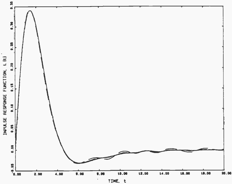
Figure 4-2. Heaving hemisphere;  $\Delta t = 0.1$ ; 64 panels — — , 144 panels - - - , 256 panels . . . .
