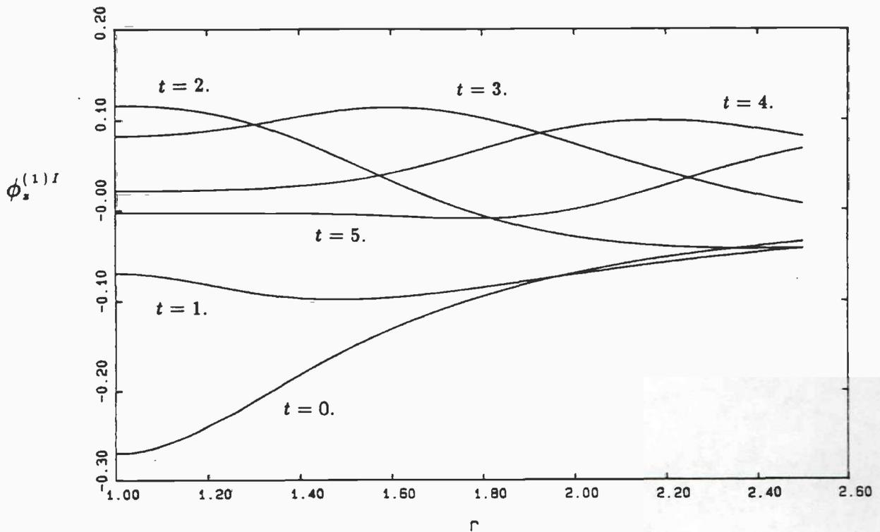
Figure 10-2. The heaving cylinder.  $\phi_z^{(1)I}(\vec{r}, t)$  on the free surface in the region close to the body.  $\Delta t = 0.1$ ; panelling on the body:  $24 \times 36$  (bottom & side  $\times$  azimuthal); the infinite cylinder truncated at  $z = -6.0$ , discretized by 48 points. Compare with Figure 9-4.
