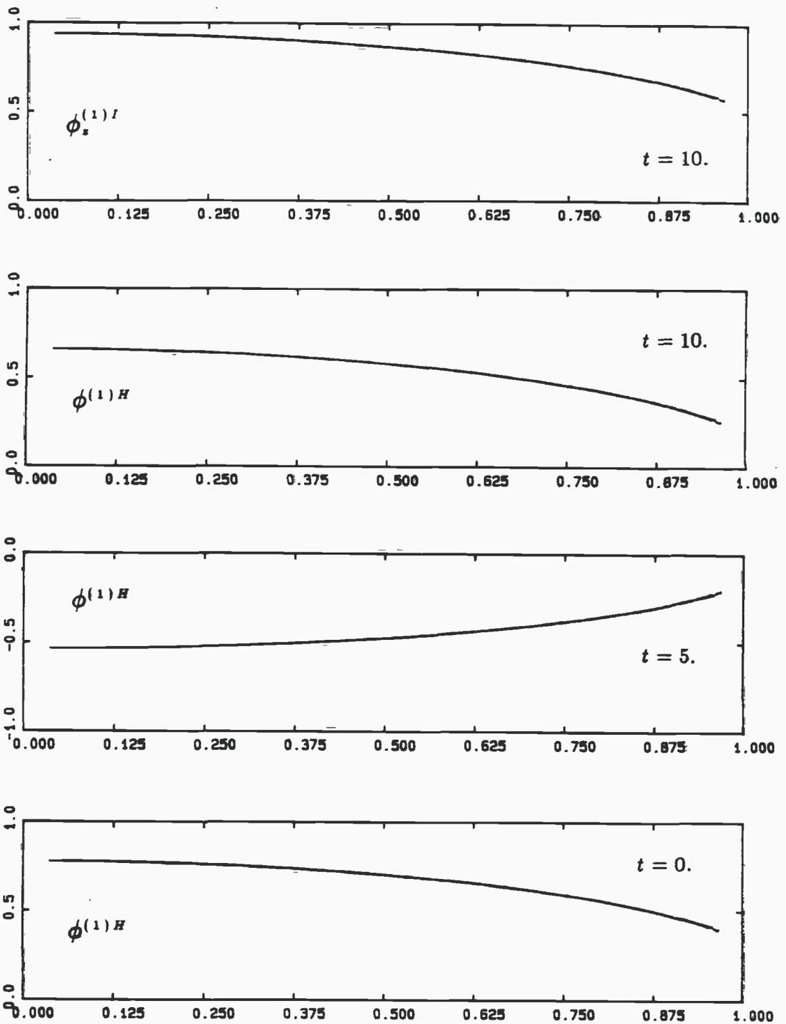
Figure 9-1. The heaving cylinder.  $\phi^{(1)H}(\vec{r}, t)$  for  $\omega = 1.2533$  and  $\phi^{(1)I}(\vec{r}, t)$  on the cylinder bottom. All results are for  $\Delta t = 0.1$ . Panelling: 24x36 ——— ; 24x72 — — — ; and 36x54 - - - ; (bottom & side x azimuthal).
