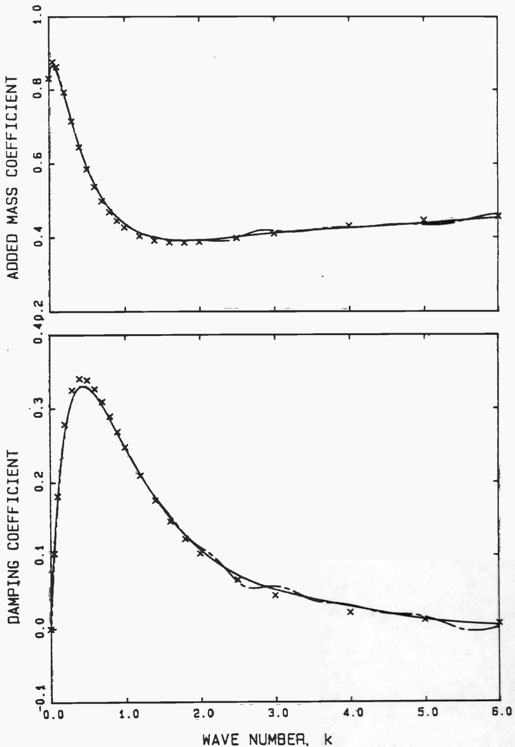
Figure 6-10. Heaving hemisphere. Transform of the patched functions: numerical portion for 64 panels,  $\Delta t = 0.2$  truncated at  $t = 30$ , — ; the same model without patching truncated at  $t = 30$ , - - -. Results from Hulme (1982)  $\times$  . Coefficients are non-dimensionalized by the displaced fluid mass.
