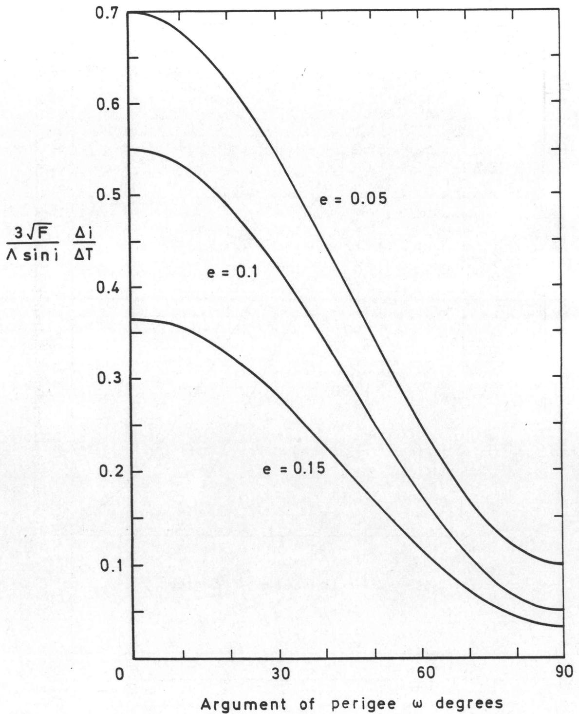
Fig 6 Variation of  $\Delta i/\Delta T$  with  $\omega$  for eccentric orbits, as given by equation (3)
