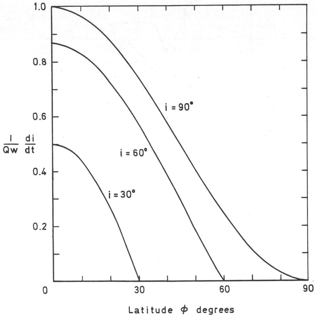
Fig 5 Rate of change of inclination for satellite in circular orbit: effect of inclination  $i$  and latitude  $\phi$
