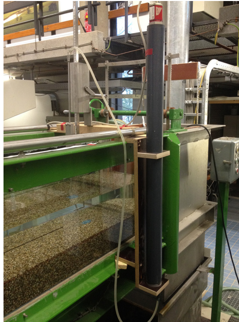
Figure 3.9: Water level meter at the downstream end of the flume. The meter is a Temposonics® magnetostrictive linear position sensor (G-series) and is fitted inside the grey tube, connected to a pitot tube in the water that measures the static water pressure.
