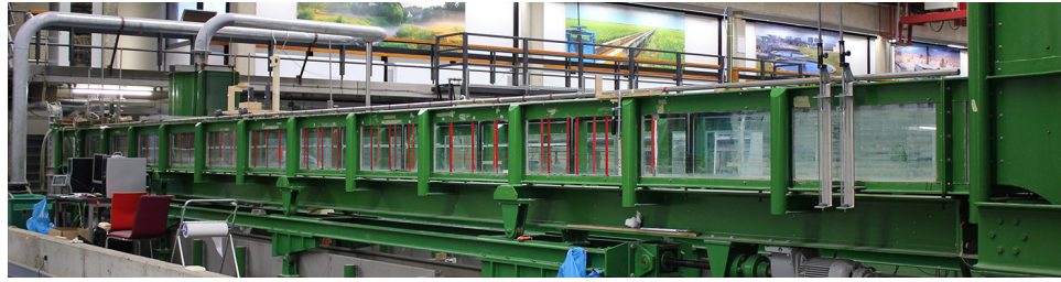
Figure 3.1: Picture of the tilting flume of the Water Lab of the Faculty of Civil Engineering and Geosciences of Delft University of Technology. The upstream side is at the right hand side.
