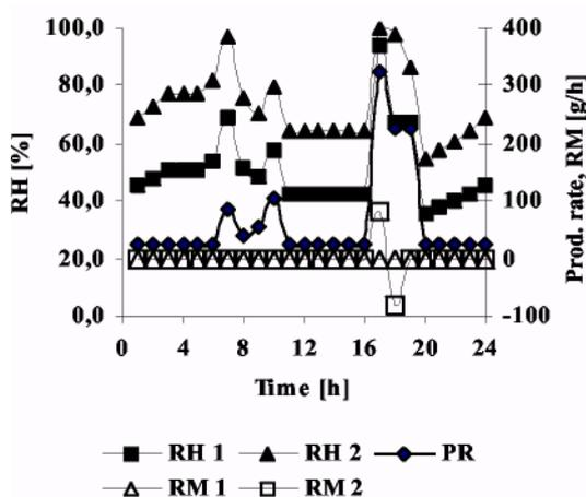
Figure 2. Course of RH, moisture production PR and RM (= PR minus removal) in the kitchen; outdoor (1) and indoor air ventilation (2).
