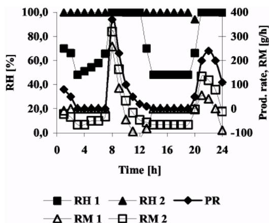
Figure 4. Course of RH, moisture production PR and RM (= PR minus removal) in the bathroom; outdoor (1) and indoor air ventilation (2).
