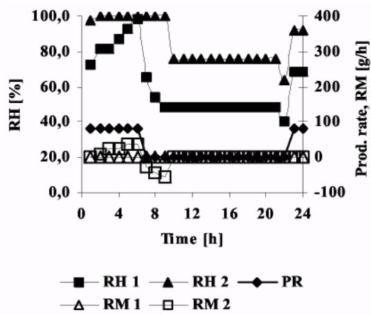
Figure 3. Course of RH, moisture production PR and RM (= PR minus removal) in the bedroom; outdoor (1) and indoor air ventilation (2).
