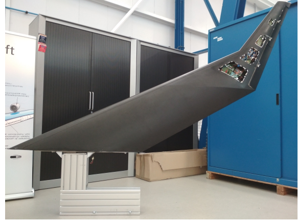
(b) Wind tunnel model with balance connection
