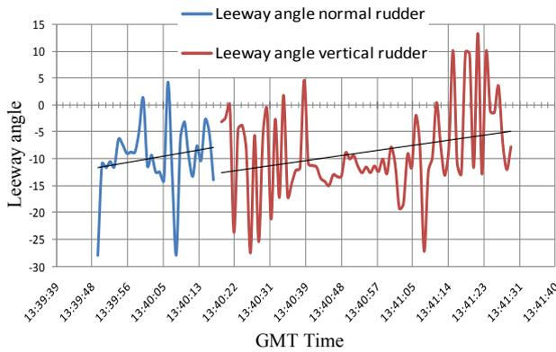
Fig. 5. Leeway angle measured for both rudder positions
