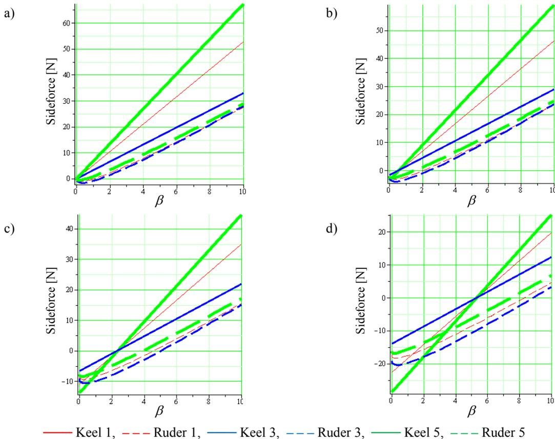
Fig. 3. Side force for hull model 366; a)  $F_n = 0.3$ ,  $\alpha = 4^\circ$ ,  $f = 0^\circ$ ,  $\delta_{ru} = 0$ ; b)  $F_n = 0.3$ ,  $\alpha = 4^\circ$ ,  $f = 10^\circ$ ,  $\delta_{ru} = 0$ ; c)  $F_n = 0.3$ ,  $\alpha = 4^\circ$ ,  $f = 20^\circ$ ,  $\delta_{ru} = 0$ ; d)  $F_n = 0.3$ ,  $\alpha = 4^\circ$ ,  $f = 30^\circ$ ,  $\delta_{ru} = 0$
