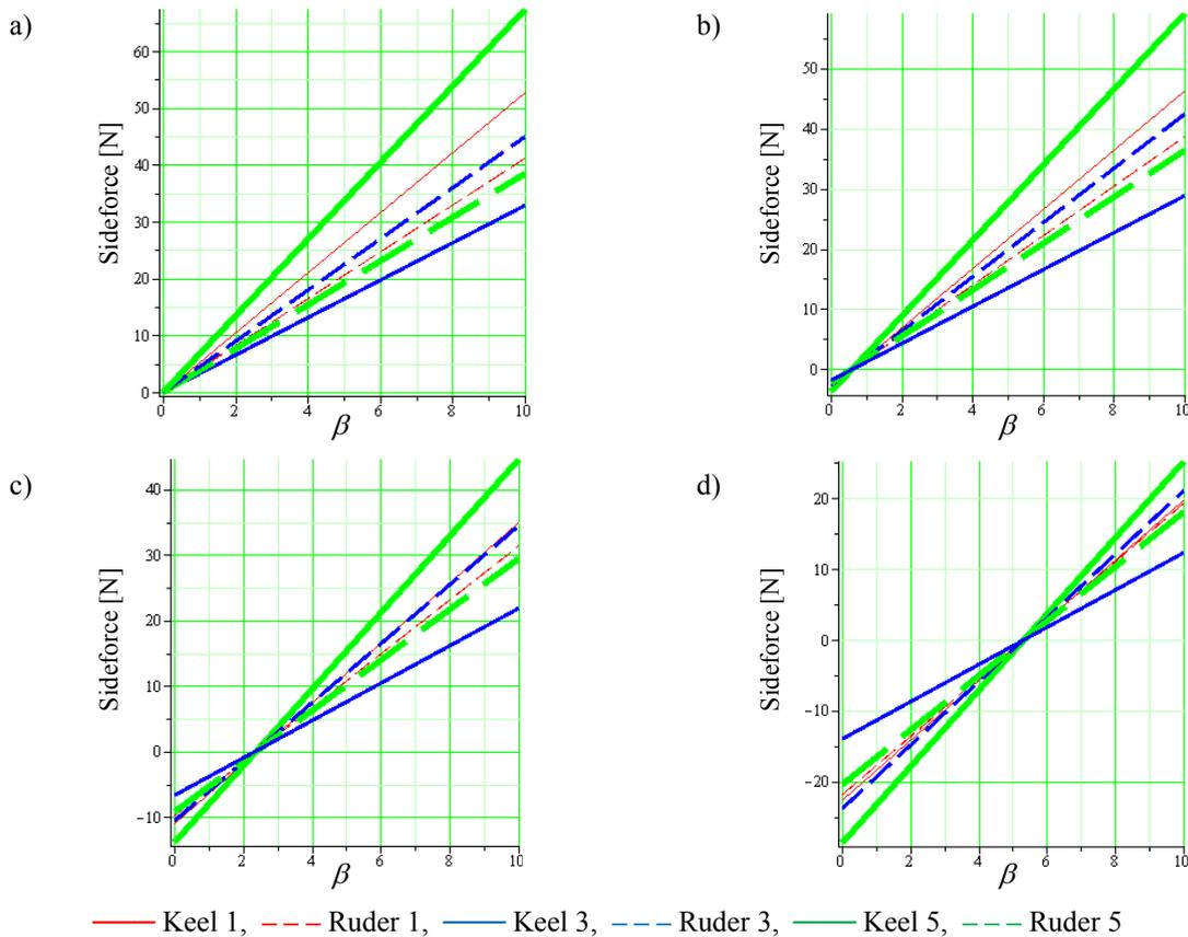
Fig. 4. Side forces assuming a vertical position of the rudder or hull model 366; a)  $F_n = 0.3, \alpha = 4^\circ, f = 0^\circ, \delta_{ru} = 0$ ; b)  $F_n = 0.3, \alpha = 4^\circ, f = 10^\circ, \delta_{ru} = 0$ ; c)  $F_n = 0.3, \alpha = 4^\circ, f = 20^\circ, \delta_{ru} = 0$ ; d)  $F_n = 0.3, \alpha = 4^\circ, f = 30^\circ, \delta_{ru} = 0$
