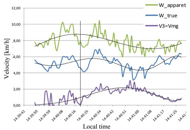
Fig. 10. Apparent and true wind speed compared with velocity made good for windward sailing
