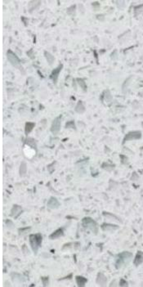
WHITE CONCRETE WITH STONE, METAL AND GLASS FRAGMENTS
