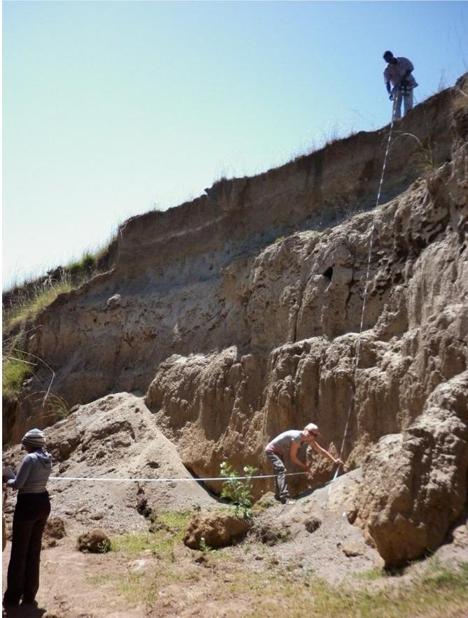
Fig. 3.4.2. Using measuring tape to measure gully dimensions in the field.
