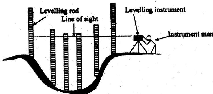
Fig. 3.4.1. Measuring the profile of a gully (Tulu 2011).
