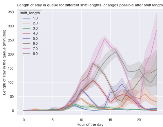
Figure 6.40: Length of stay in the queue over the day with different shift lengths - Optimization variant 1
