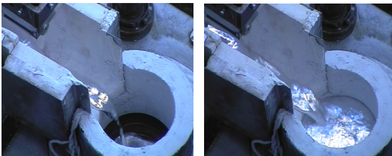
Fig. 5.11. Inflow of liquid aluminium into the mould during the start-up of Exp3.
