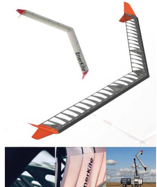
Dbox and rib skeleton, with membrane cover of early generation prototype wing.
