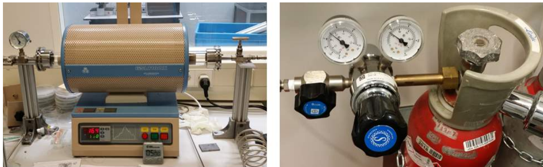
Figure 5.14: At the left a photograph of the CVD oven is shown. The photograph on the right shows one of the gas bottles (hydrogen) that was used.
