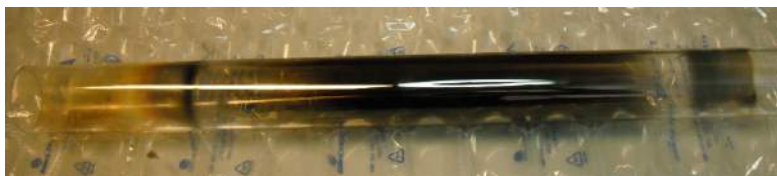
Figure 5.13: The quartz tube after four growth experiments. Carbon deposits have turned the tube black and opaque.
