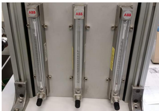
Figure 5.15: A photograph of the variable area flow meters used in this study.
