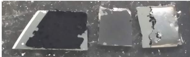
Figure 6.4: Photograph of three forests. The left forest is pure black and contains low amounts of a-c. The central forest is grayish and contains medium amounts of a-c, while the forest on the right shows a shiny top most likely due to a thin graphite layer.
