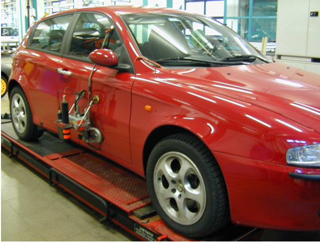
Figure 19 Photo of a gyrometric box that measures lateral acceleration and speed attached to a vehicle
