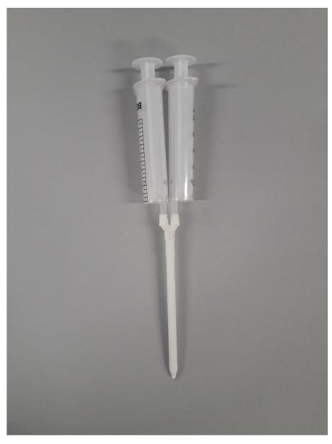
Figure 6 Syringes and static mixing nozzle assembly
