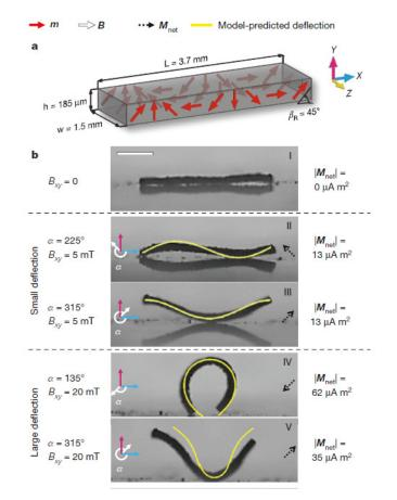
*Figure 2.2:* Magnetic soft material strip that is activated by different directions and strengths of a magnetic field and therefore it creates different shape changes (Hu, Lum, Mastrangeli, & Sitti, 2018)
