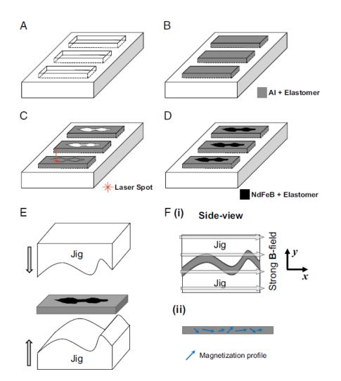
*Figure 2.12:* B: the magnetic soft material cures in a mould. E: the material is placed in a mould before magnetization. F (i): the material gets magnetized. (Lum et al., 2016)
