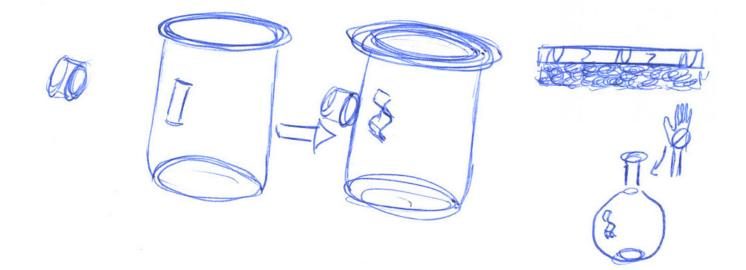
*Figure 4.23:* The cleaning tool for hard to enter spaces. Through the elastomer, the material can be rolled up and placed in spaces where the hand cannot come. By a permanent magnet, the wiping can be controlled on the outside and by moving the magnet closer and further away the magnetic soft material can contract and relax to create a scrubbing motion.
