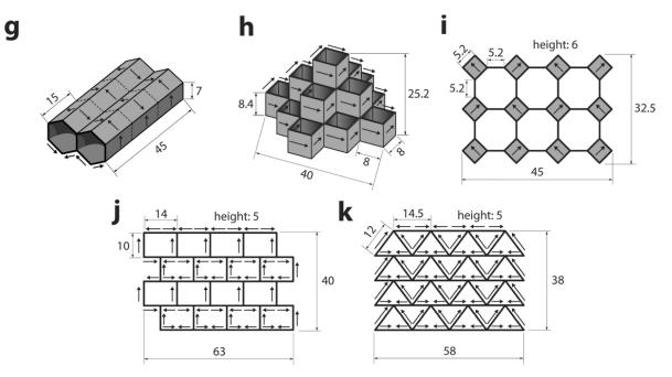
Figure 3 Dimensions printed 3D structures from the MIT paper (Kim et al., 2018)
