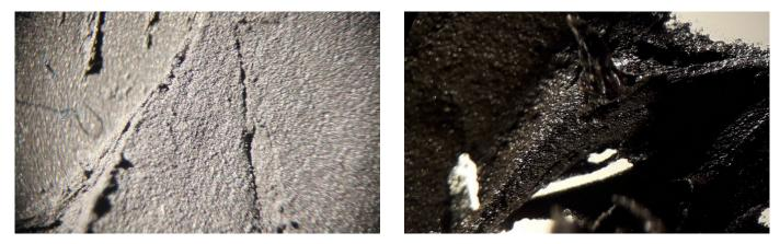
*Figure 3.6:* (left) Evenly distributed magnetic particles in Ecoflex. Mixed by hand. Non-magnetized ink. (right) Magnetized mixed ink. The picture is darker because another camera was used that was not compatible with the microscope.
