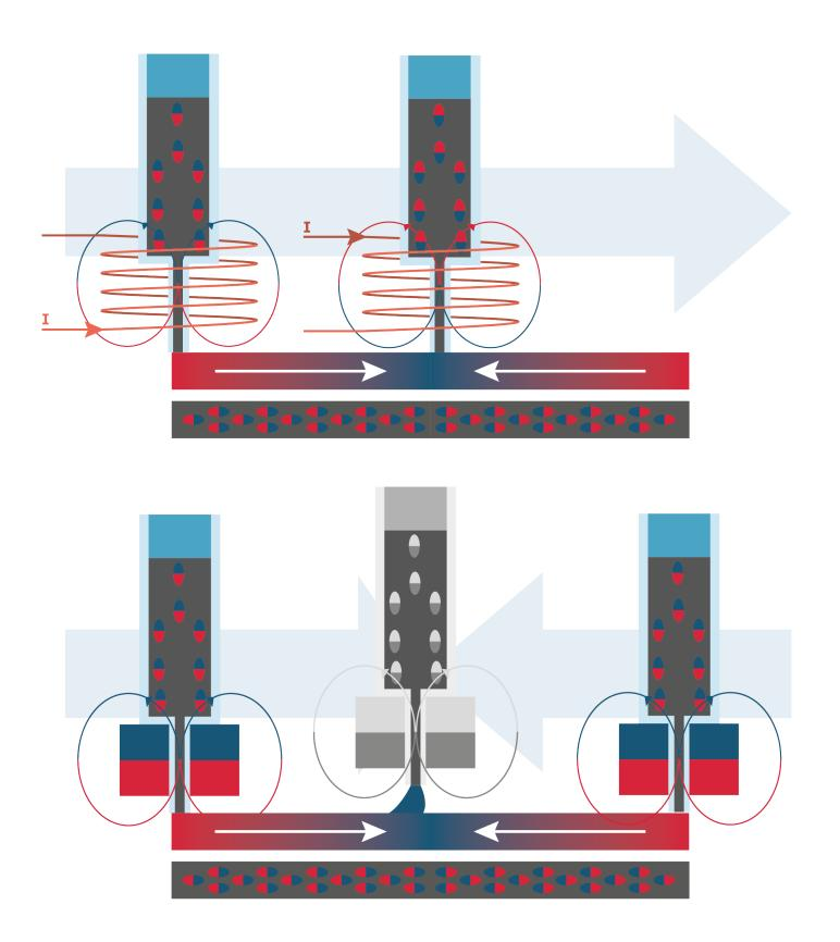
*Figure 3.41:* The difference in printing one line with opposite magnetic field directions by an electromagnet (top) or a permanent magnet (bottom)
