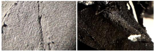
The first picture is a microscope picture of unmagnetized ink and the second of the magnetized ink of this test. From the comparison of these two pictures, we cannot conclude if the particles do agglomerate or not. What was noticed throughout the experiment was that the particles still stayed distributed throughout the material.
