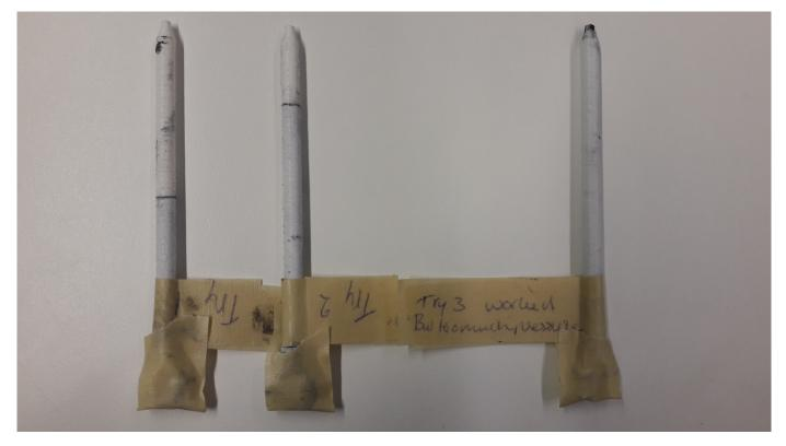
*Figure 3.22:* The three static mixing nozzles from static mixing nozzle test 1 (Appendix B.b.1). The first two inks had a too high viscosity and the ink did not come completely through the static mixing nozzle. The stipes indicate to where in the nozzle the ink came. The third static mixing nozzle was used with a less viscous ink and it came through.
