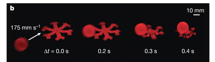
Figure 2.9: A gripper catches a ball when activated by a magnetic field (Y. Kim et al., 2018)
