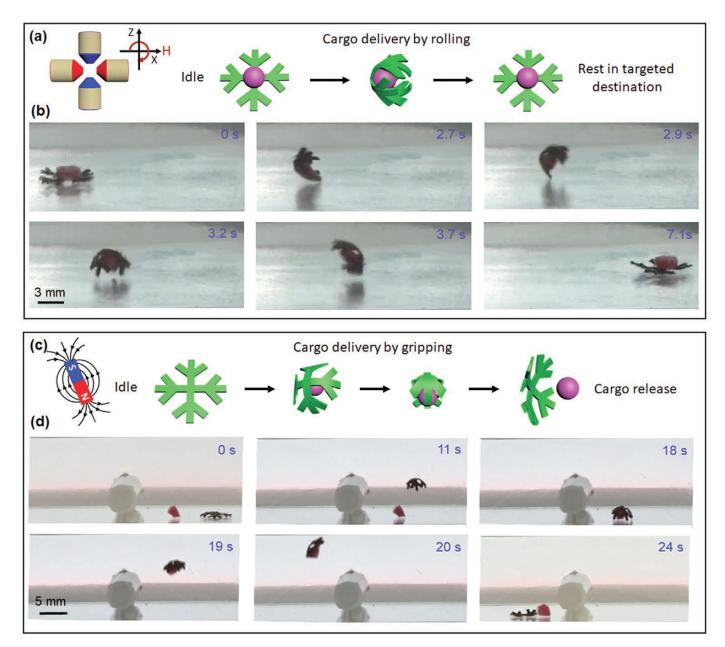
*Figure 2.10:* In picture (a)(b) the cargo is transported by a rolling jellyfish inspired swimmer. In picture (c)(d) the cargo is gripped moved and later released. (Goudu et al., 2020)
