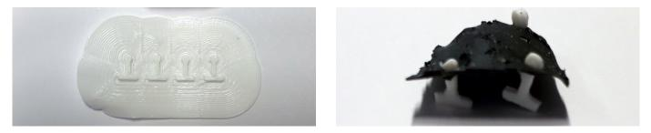
*Figure 4.29:* Prototype of the designed connectors. The best size had a thickness of 0.8 mm for the straight parts and a diameter of 1.6 mm for the circle on top.
