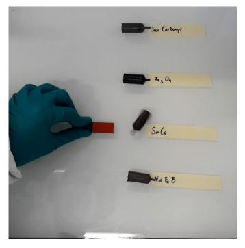
*Figure 3.17:* Repelling the SmCo samples, makes them turn around so that two opposite poles can attract each other
