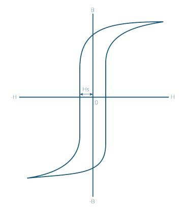
*Figure 3.19: Hysteresis curve of a magnet. The gap Hs shows the coercivity of the magnet.*
