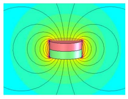
Figure 13 Magnetic field of a disc magnet (K&J Magnetics, n.d.)
