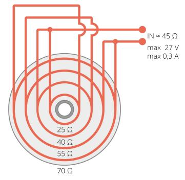
*Figure H.2:* The connections of the four spun coils of the electromagnet
