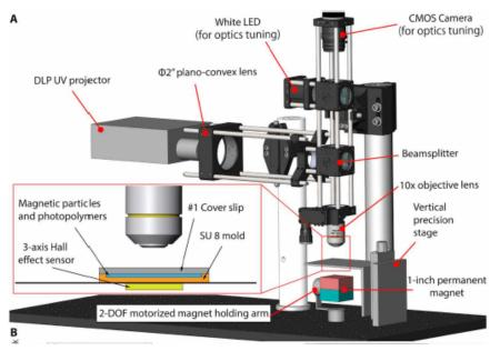
*Figure 2.13:* The manufacturing method from the study by Xu et al. (2019) where selective parts of the material are cured. The process is based on ultraviolet stereolithography. The 1-inch permanent magnet is the external magnetic field used to orient the magnetic particles. The lenses are used to cure specific regions of the material.
