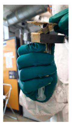
**Figure 3.44:** Syringe with mixed ink and a ring magnet at the nozzle. The larger ferrite magnet is further up the syringe to prevent the magnetic field from pulling the extruded ink of the glass plate.
