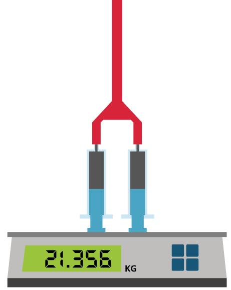
*Figure 3.3:* The setup to measure the force needed to extrude the ink through the static mixing nozzle
