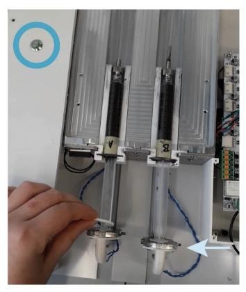
*Figure F.3:* The button in the circle moves the plates up and down and shows the light on the status of the plates. One of the plates is pointed to with an arrow
