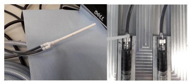
The new tubes worked and were stiff enough. In the picture above the connection of the tubes to the syringes can be seen when the entire tubes are filled with ink, and they have not swollen through the extrusion. The maximum measured diameter was 6,1 mm.
