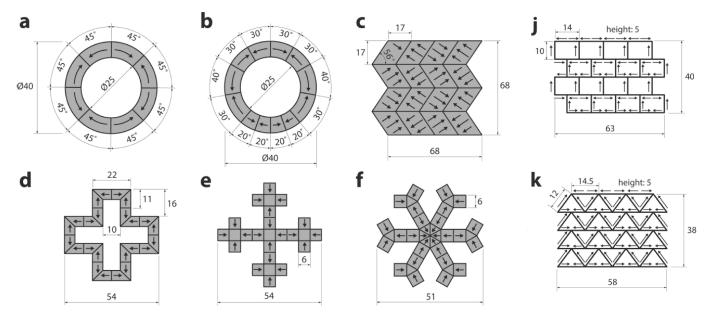
Figure 4.17: A-F: Printed 2D shapes MIT. J and K: Printed 3D shapes MIT (Y. Kim et al., 2018)
