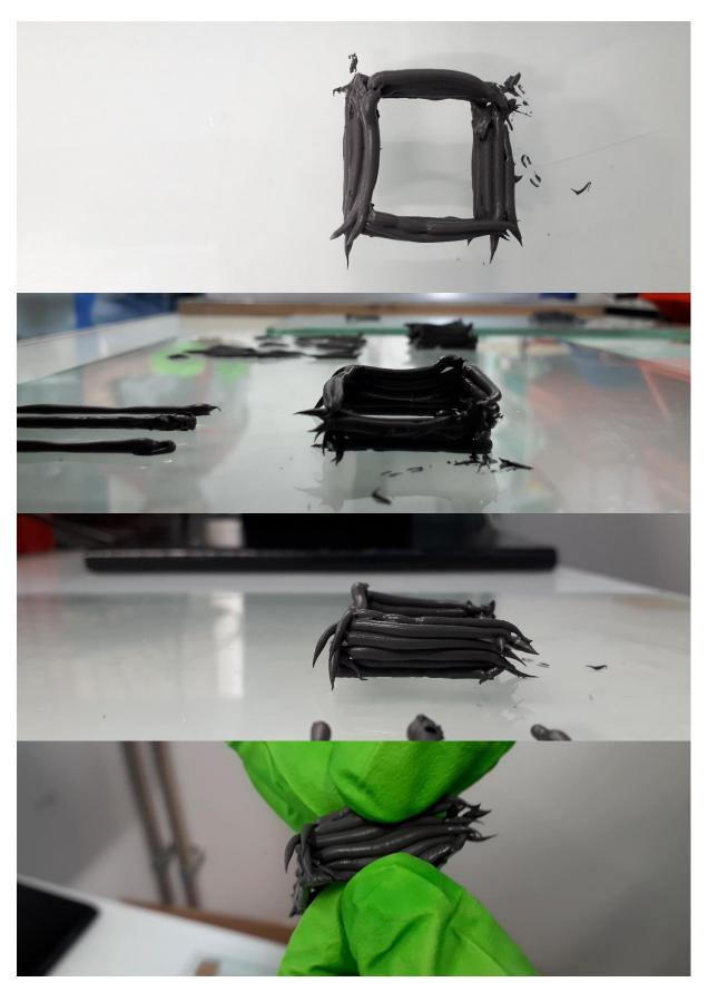
Figure 11 Experiment 4 after curing in the oven
