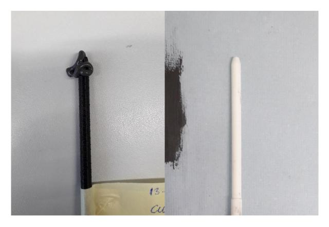
Ink curing after extrusion through the static mixing nozzle (static mixing nozzle test) The T7E1 was cured after it was extruded and mixed in the static mixing nozzle extrusion force measurement test.
