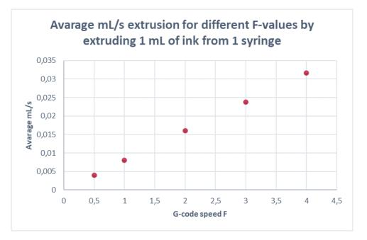
*Figure 3.38:* The value of F in the G-code and the corresponding extrusion speed. This was measured with the extrusion of 1 mL of ink; A89 or B89 in the G-code.
