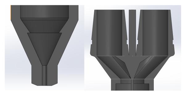
Figure 2 extrusion part of the static mixing nozzle Figure 3 part to insert the two ink compounds
