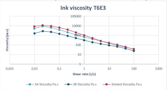
This ink also shows the shear-thinning properties and has the lowest measured viscosity of all the tree inks that were tested in this experiment.
