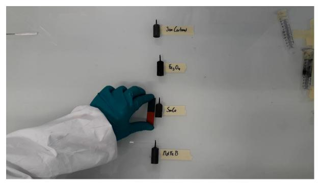
Figure 4 The SmCo sample is not pushed away as was the case in magnetizer experiment 1 with this orientation of the magnet
