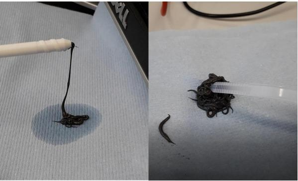
The ink got extruded through the static mixing nozzle with the printer setup and the ink did cure. This means that both ink components, A and B, can be extruded through the static mixing nozzle together in the 3D printer system and got mixed. The lines on the pile of ink are still individual which means that the ink has a bit of print stability which. Due to the not swollen tubes and the extruded ink, it was also tried to print the first line with it on the 3D printer.
