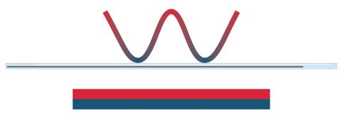
*Figure 4.25:* The South poles of the magnetic soft material are attracted to the North pole of the magnet that is facing the material. Making the material contract into an M-shape.
