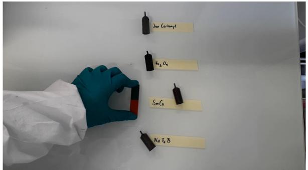
Figure 10 Repelling the samples, makes them role away. The NdFeB particles have a big field strength and turn to the magnet.
