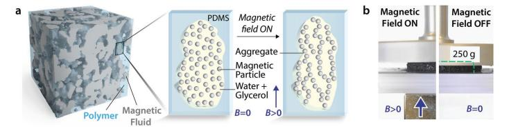
*Figure 2.11:* (a) The magnetic particles align when the material is placed in a magnetic field. (b) On the left side, the material is placed in a magnetic field and lifts the weight put upon it, on the right the material with the same weight without the magnetic field. (Testa et al., 2019)
