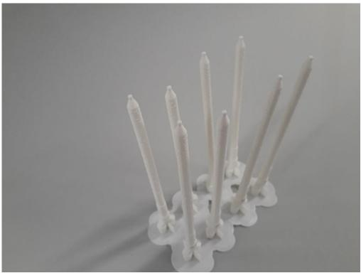
Figure 4 Printed static mixing nozzles first attempt, closed nozzles
