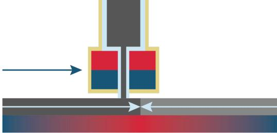
Figure 3 Extrusion of two different lines of ink that join in the middle to create a magnetization pattern
