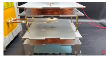
*Figure 4.15:* The magnetic field for activation is created by the two electromagnet coils (TV, 2020)
