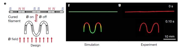
*Figure 2.1:* Magnetic soft material with different magnetization patterns (e). When the strip is placed in a magnetic field the strip transforms to an "M" shape. (Y. Kim et al., 2018)
