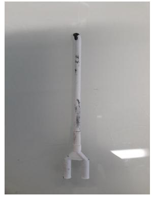
The T6E3 NdFeB ink was cured after it was extruded and mixed through the static mixing nozzle.
