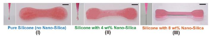
*Figure 3.23:* Silicones with different amounts of Nano-Silica. The more Nano-Silica is added the better the silicone keeps its printed shape (III). In (I) the print stability is very low and the defined edges have deformed over time. (Zhou et al., 2019)
