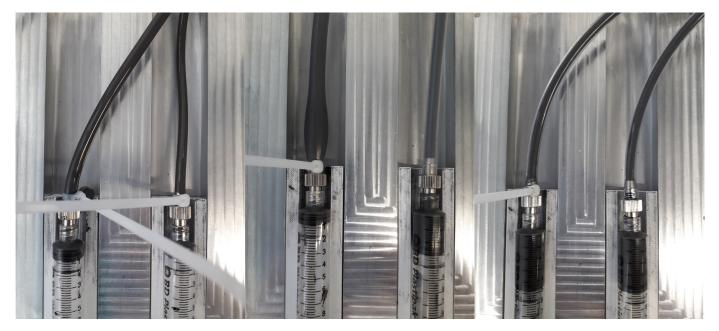
*Figure 3.37:* The three types of tubes tested during this project, the one on the right has the stiffest tubes and worked the best because they did not swell up
