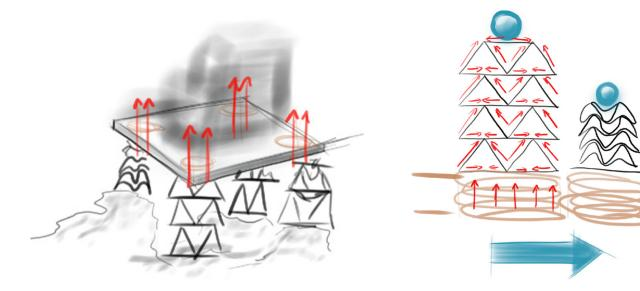
*Figure 4.20: Surface levelling mechanism. Every 3D mechanism is individually controlled by its electromagnet.*
