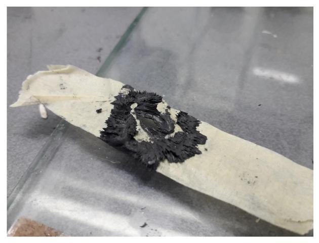
Figure 11 Ink that got attracted by the magnet that was attached to the syringe. The spikes in the ink show the magnetic field of the ring magnet
