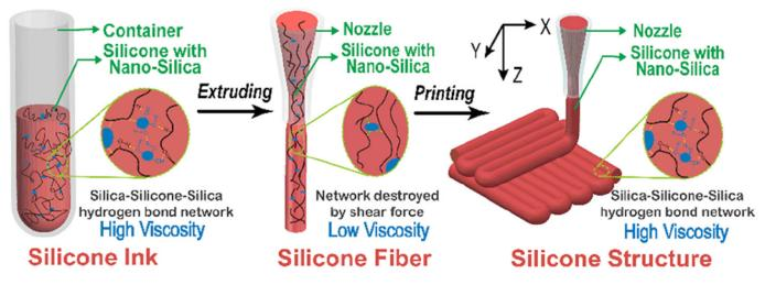
*Figure 2.18:* The viscosity of the silicone changes throughout the printing process through the addition of fumed silica particles (Zhou et al., 2019)
