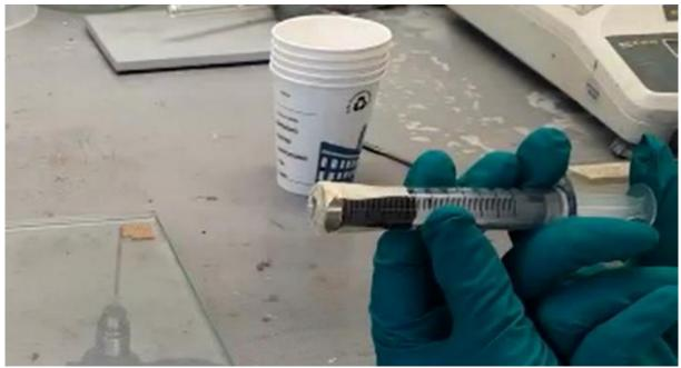
Figure 4 Syringe with mixed ink and a ring magnet at the nozzle
