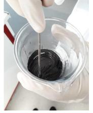
Figure 3 Ecoflex part B mixed with iron powder
