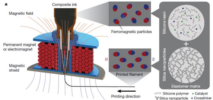
*Figure 2.16:* The 3D printing process of magnetic soft material developed by Y. Kim et al. (2018). The magnetic particles orient with the magnetic field that is applied through the electromagnet at the nozzle while printing. The shield is attached between the electromagnet and the printed material so that the printed magnetization patterns will not be distorted during the printing process.
