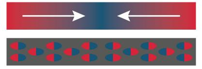
*Figure 4.27:* How the particles are oriented in the ink in comparison with the schematic North and South poles of the magnetic soft material
