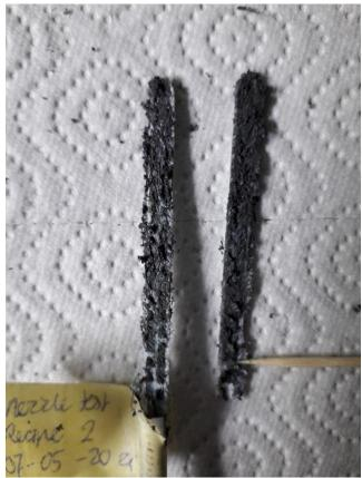
Figure 2 Sawn open static mixing nozzle v1 with T6E4 ink
