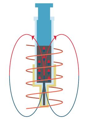
**Figure 3.14:** The syringe is placed inside a coil in the magnetizer. The magnetic field of the coil magnetizes the magnetic particles and their poles become the same as that of the magnetic field.
