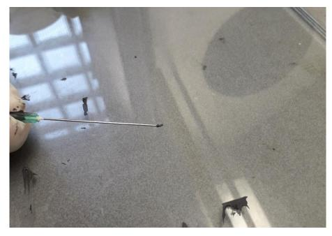
Figure 9 Test if the first material could be extruded through a needle with a 0.4mm diameter
