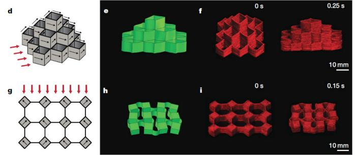
Figure 2.17: More complex shapes made from magnetic soft materials, made with 3D printing (Y. Kim et al., 2018)
