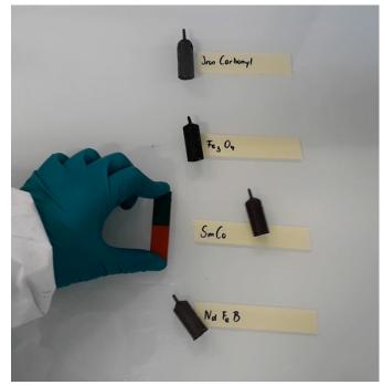
*Figure 3.18:* Repelling SmCo the samples, makes them role away. The NdFeB particles have a big field strength and turn to the magnet.
