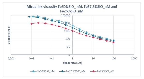
*Figure 3.12:* The viscosity of inks Fe50%SiO\_nM, Fe37,5%SiO\_nM and Fe25%SiO\_nM made in static mixing nozzle test 4 with different amounts of fumed silica relative to the MIT recipe. The viscosity of the ink increases if more fumed silica is added.
