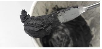
*Figure 3.8:* The smoother, less viscous ink with the 1:1 ratio from experiment 2
