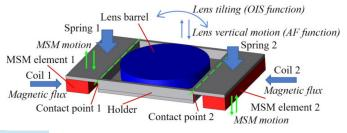
*Figure 2.4:* The combined autofocus and optical image stabilization system for a camera. The red boxes are the magnetic shape memory alloy parts. (Gabdullin et al., 2020)
