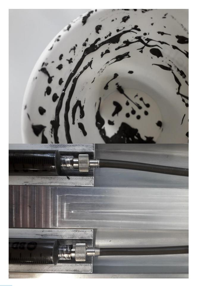
After the extrusion of the syringes stopped, the ink kept coming out of the static mixing nozzle. This is probably due to build up pressure in the system. The hoses connecting the syringes with the static mixing nozzle are very flexible and have expanded as can be seen in the figure above. The upper syringe is filled with ink component A (the more viscous one) and this can explain why that tube has expanded more than the one coming from ink component B.
