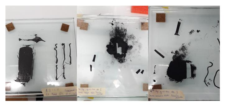
*Figure 3.25:* On the left is the Fe50%SiO\_nM ink with iron carbonyl particles on which the other two inks are based. In the middle is the Fe50%SiO\_nM ink of which the iron carbonyl particles are converted to Fe3O4 particles by wt%. On the right is the Fe50%SiO\_nM ink of which the iron carbonyl particles are converted to Fe3O4 particles by vol%.
