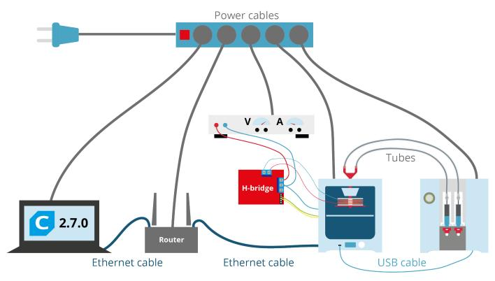
Figure F.9: The 3D printer set up with all the cable and tube connections including the electromagnet
