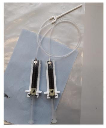
*Figure F.2:* The ink guiding system: conversion pieces, 10 mL syringes, Luer lock connections, tubes, static mixing nozzle
