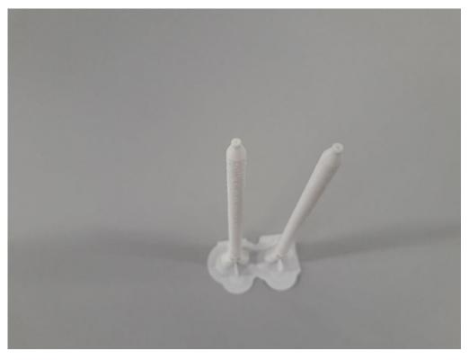
Figure 5 Printed static mixing nozzles third attempt open nozzles with a diameter of 0.4 mm
