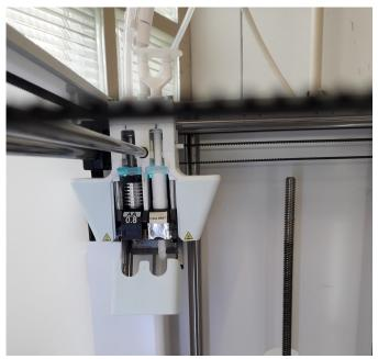
*Figure F.6: Printer core inside the printer head, with stabilizer and static mixing nozzle*
