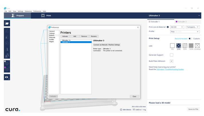
*Figure F.8:* The main screen of Cura 2.7.0 with the popup screen of "manage printers" to connect to the 3D printer
