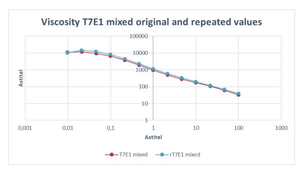
The viscosity of Ecoflex components A, B and mixed was also measured in this test:
