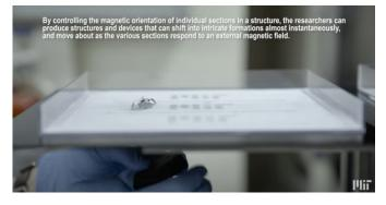
*Figure 4.14:* The magnetic soft material is activated by a permanent magnet that is moved and rotated under the glass plate by a researcher ((MIT), 2018)
