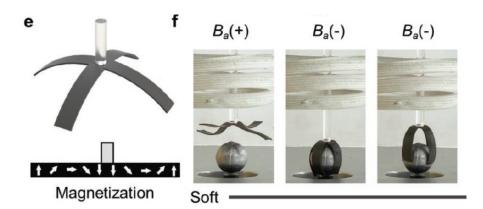
*Figure 2.8:* The gripper in its soft state (when it acts like magnetic soft material) is not able to lift the ball (Ze et al., 2020)
