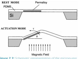
*Figure 2.3:* Schematic representation of the micropump and its activation by an external magnetic field (Khoo & Liu, 2001)
