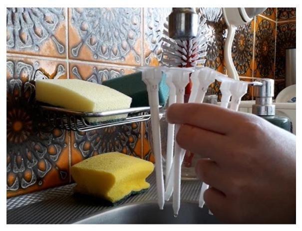
Figure 7 Test if the static mixing nozzles are hollow by running water through them
