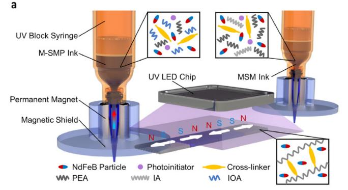
*Figure 2.15:* The 3D printing of magnetic soft materials in the study Ma et al. (2020) is part of a multimaterial printing system together with magnetic shape memory polymers. The magnetic fields of the magnetic particles are aligned with the field of the permanent magnet placed at the nozzle. A magnetic shield is placed between the permanent magnets and the printed material so that the printed magnetization patterns will not be distorted.
