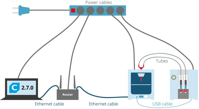
*Figure F.1:* The 3D printer set up with all the cable and tube connections **264**
