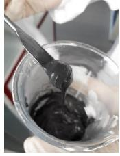
Figure 2 Ecoflex part B mixed with iron powder and Ecoflex part A
