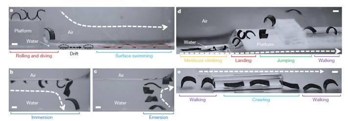
*Figure 2.7:* The strip of figure 2.2 can have different ways of locomotion due to different orientations of the external magnetic field and the frequency in which it moves(Hu et al., 2018)
