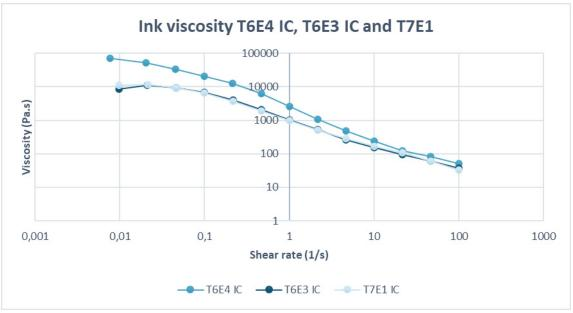
These two graphs show the relation of the mixed T7E1 ink with the other mixed ink viscosity values. As said in the introduction, there was aimed at a viscosity in between the T6E3 and the T6E4. This has not succeeded. The viscosity values of the T7E1 are more comparable with the T6E3, and therefore probably has a too low viscosity for a good print stability.
