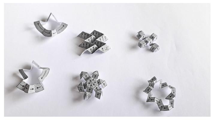
*Figure 4.18:* Prototypes from the MIT 2D shapes. The arrow represent the magnetic field direction, so all the arrows have to point in the same direction.
