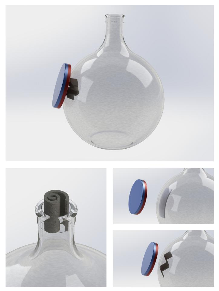
*Figure 4.24:* The cleaning tool is rolled up and put inside a vase. Depending on the distance of the magnet to the material, the strength of the shape transformation differs according to the magnetic field strength. The position of the magnet relative to the vase moves the tool over the inner surface of the vase.
