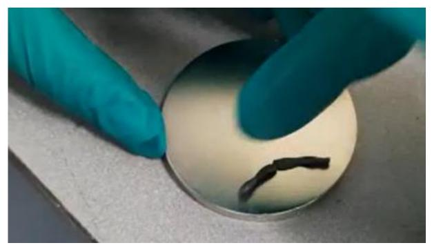
Figure 12 The ends of the extruded strip curl up in the magnetic field of the Neodymium magnet
