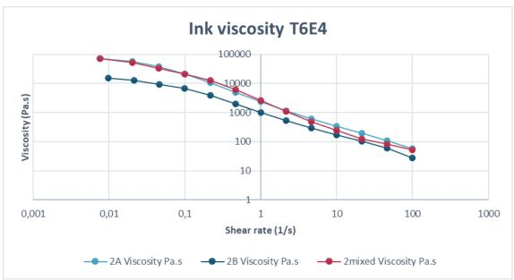
The graphs of the T6E4 ink show the same shear thinning behaviour as the T3E1 ink. The viscosity is a bit lower than that of T3E1 which can be seen in the Mixed ink viscosity graph.
