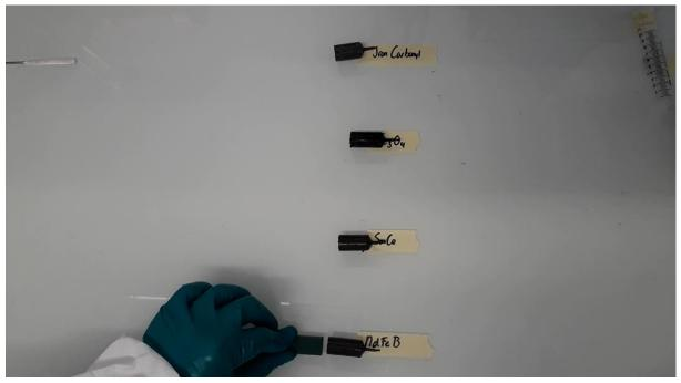
Figure 1 NdFeB particles are not attracted by the magnetic field, which was the case for this orientation of the magnet in experiment 1
