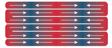
*Figure 4.26:* The schematic representation of the print process of the M-shape. The path is the path that the printer head travels, the red and blue colours the magnetization pattern and the arrows the direction of the magnetic field of the electromagnet attached to the nozzle during the print process.
