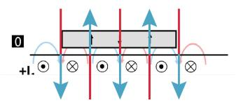
*Figure 4.16:* The current of the neighbouring wires run in opposite directions. The place where the magnetic fields of two wires meet, both turn up or down, creating small local magnetic fields. (Hsu et al., 2020)
