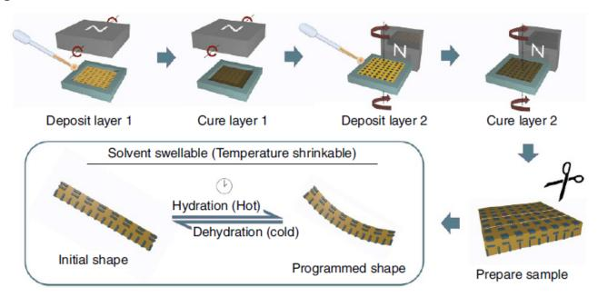
*Figure 2.14:* The production process in the study by Erb et al. (2013). First, the first layer is placed in the mould and cured. After that the second layer is placed on top of the external magnetic field is turned and the second layer is cured.
