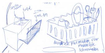
**Figure 4.4:** (left) A box with multiple functions. Here a table and chair pop out of the shape. (right) A drying rack for dishes that can be folded in to be easier to clean
