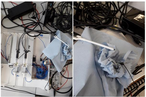
The ink got extruded through both the tubes and the static mixing nozzle, without the motors skipping steps. They ran smoothly the entire time.
