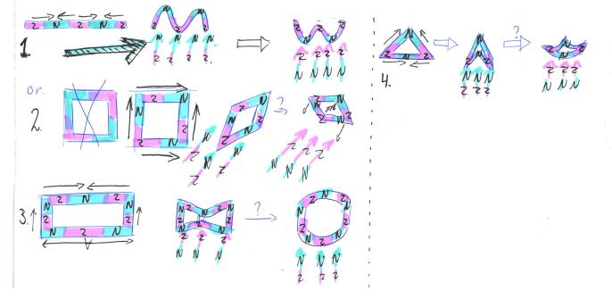
*Figure 4.19:* 3D MIT shape transformation analysis. The arrows from MIT were translated into North and South poles. While keeping the shape in the same orientation, two magnetic field directions were thought out.
