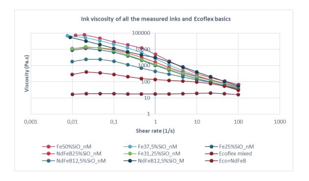
*Figure 3.43:* The viscosity measurements of the inks that were measured throughout the project and two reference measurements of plain mixed Ecoflex and Ecoflex with only NdFeB particles which also shows shear-thinning properties
