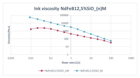
Figure 3.27: The viscosity increase due to the magnetization of the mixed NdFeB12,5%SiO ink
