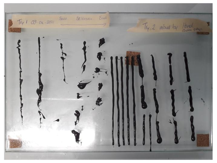
*Figure 3.5:* (left) cured ink that is mixed by the static mixing nozzle. (right) cured ink that is mixed by hand according to the first mixing order presented in this chapter.
