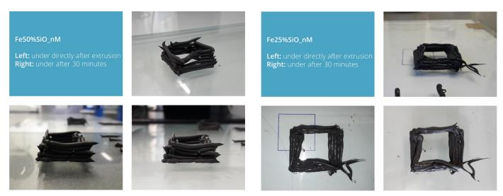
**Figure 3.24:** Fe50%SiO\_nM has a higher viscosity than Fe25%SiO\_nM and is better at holding its shape. The holes present just after the ink was extruded were still present after more than 30 minutes of waiting. The Fe25%SiO\_nM collapsed during the extrusion by hand (which could be a human error), and the extruded lines blended more into each other than the Fe50%SiO\_nM.
