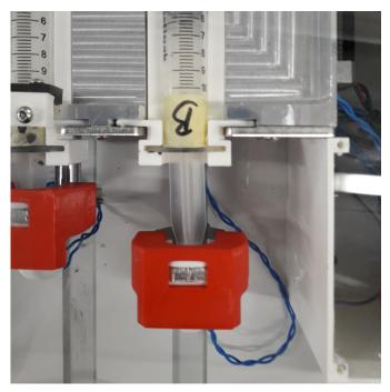
*Figure F.4:* The end of the piston with the plate against it, the white enlargement piece on top of it and the red cap over it
