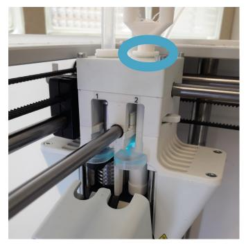
*Figure F.5:* The ring that should be pressed down when the static mixing nozzle is removed
