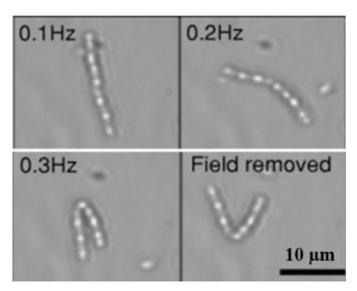
*Figure 2.5:* A strip made out of a few magnetic particles that can change its shape by an external magnetic field (Biswal & Gast, 2004; Erb, Martin, Soheilian, Pan, & Barber, 2016)
