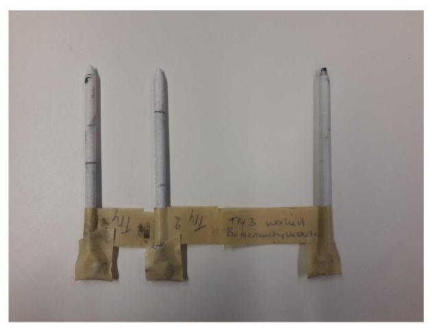
Figure 8 Nozzles used during the test. The black lines show how far the ink came inside the static mixing nozzle. In try3 the ink came out of the nozzle and therefore has no black line.
