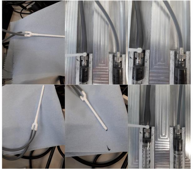
In the end, the ink of part A was retracted into the syringe to relieve the tube from the ink. Here can also be seen that there was at least 2 mL of ink in the swelling of the tube. Still, the tube of part A is expanded when compared to the part B tube.
