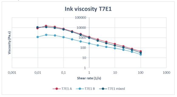
The viscosity graphs of the T7E1 follow the normal order and shape of the previously measured ink viscosities. With the mixed viscosity and part A on top and part B below. What Is different, is that part A seems to have a higher viscosity than the mixed ink, which was never the case before. Also, the starting viscosities of A and B lay farther apart than previously measured ink viscosities.
