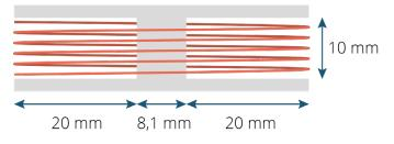
Figure H.1: The dimensions of the electromagnet coil
