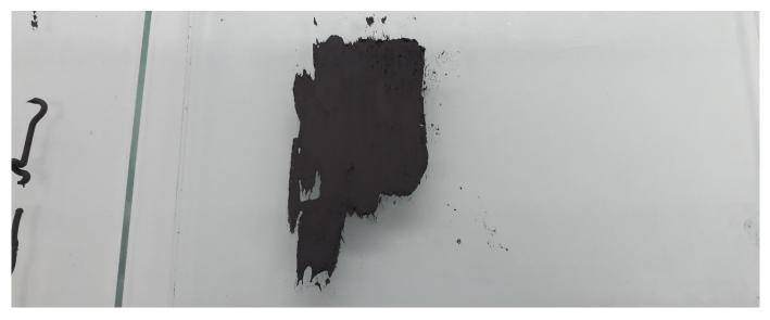
Figure 3.9: The ink with the 2A:1B ratio from experiment 3 which was too viscous to extrude through a 10 ml syringe
