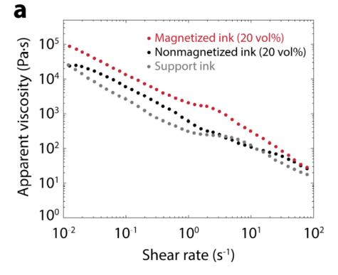
Figure 3.26: The viscosity increase of the ink from the MIT paper (Y. Kim et al., 2018)
