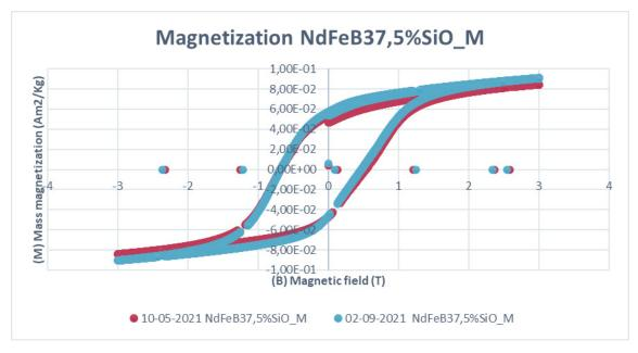
*Figure 3.21:* Magnetization curve of NdFeB37,5%SiO\_M. One sample was made during magnetizer test 1 and magnetized on 10-05-2021, the other sample was made during magnetizer test 1B and was magnetized on 02-09-2021. These measurements were both taken on 02-09-2021
