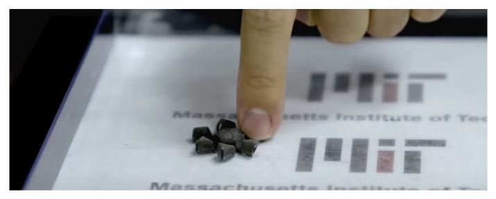
*Figure 4.1:* The magnetic soft material that is transformed under a magnetic field, is easily pressed flat by the force of a finger
