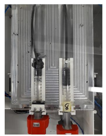
*Figure 3.35:* The 60 mL syringe to 10 mL syringe conversion pieces, the white parts in which the syringes are clicked as well as the white part near the red clips
