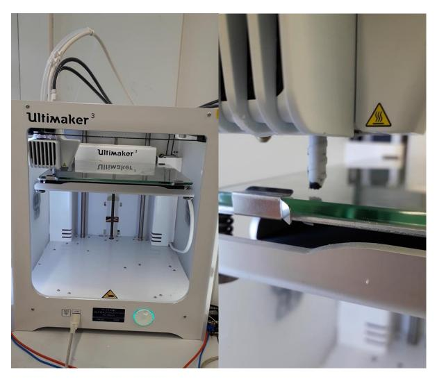
However, when it was tried to extrude ink from the syringes and draw a line of the ink on the glass plate of the 3D printer (pictures above), no ink came out of the static mixing nozzle. It was tried several times with no effect. This part of the g-code was tried again: F2 A45 (0,5 mL) B45 (0,5 mL) to get ink out of the static mixing nozzle, but still, nothing happened.
