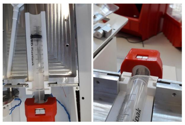
Figure 1 White 3D printed insertion pieces to convert the 60 mL syringe place to a 10 mL syringe
