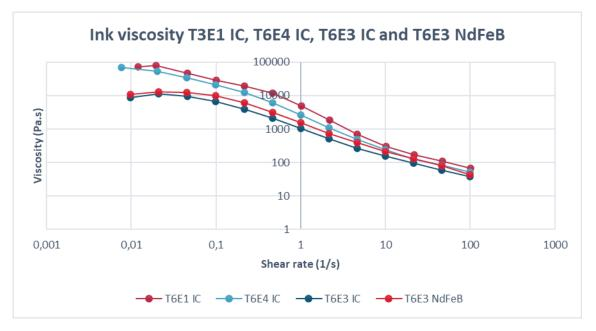
When the NdFeB based T6E3 is placed in the graph next to the viscosities of the other mixed inks measured in Static mixing nozzle test number 4, there can be seen that it does fall in the same order of magnitude of the T6E3 iron carbonyl based.
