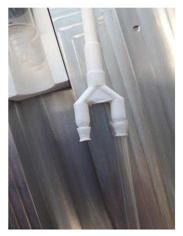
*Figure 3.36:* The new connections at the static mixing nozzle to secure the tubes
