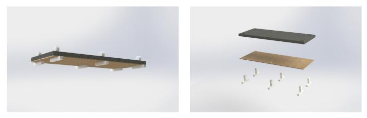
Figure 4.28: Magnetic soft material (grey) with fabric (brown) that is connected with the designed connectors (white)
