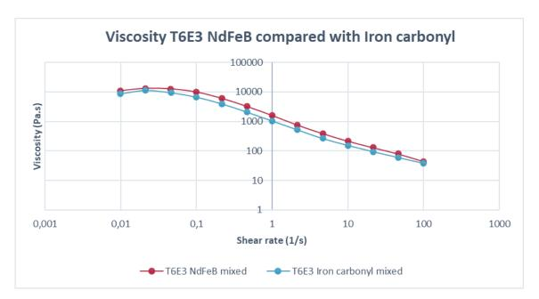
In this graph the ink viscosity of the original T6E3 with iron carbonyl particles with compared with the altered T6E3 with NdFeB particles. What can be seen is that the viscosity of the NdFeB based T6E3 is a bit higher. This can be because of the particles, but also because of conversion of the vol% of the particles, because these have been calculated with values found on the internet, instead of being specific to the particles that were used in this experiment.
