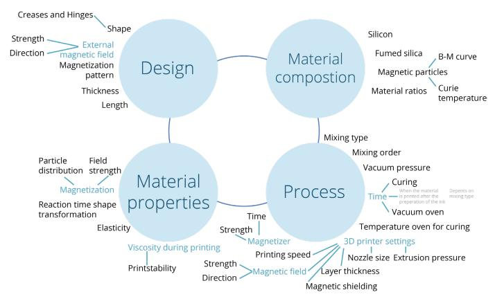
*Figure 3.2:* The magnetic soft material designers taxonomy. Magnetic soft material factors that (can) influence the performance of the magnetic soft material.
