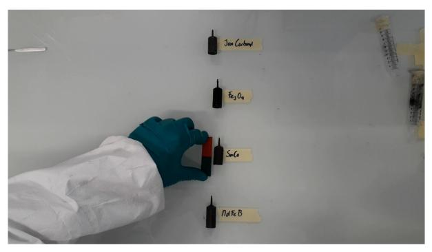
Figure 3 SmCo particles are not attracted by the magnetic field, which was the case for this orientation of the magnet in experiment 1
