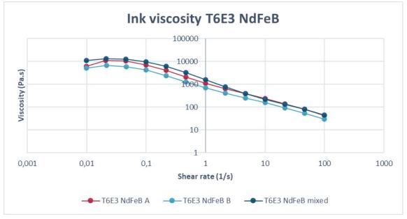
The individual and mixed ink components of the T6E3 NdFeB ink follow the same order for their viscosity in comparison with the earlier measured inks in Static mixing nozzle test 4. Where the mixed viscosity is the highest, and ink component A viscosity is above the viscosity of ink component B.
