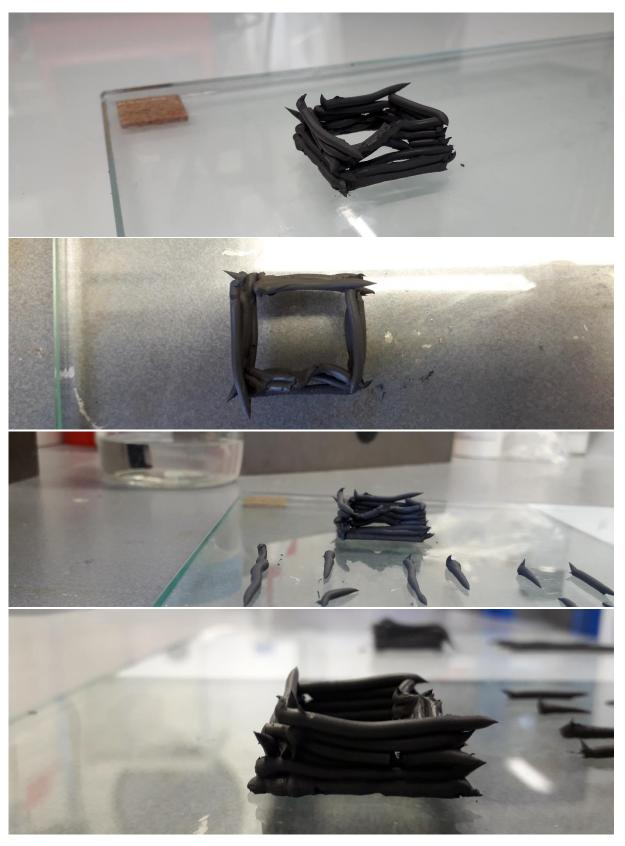
Figure 5 Experiment 1 after extruding
