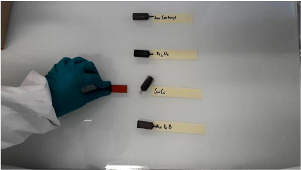
Figure 8 Repelling the samples, makes them turn around so that two opposite poles can attract each other
