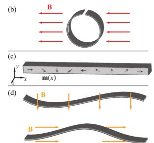
*Figure 2.6:* A strip made of magnetic soft material with a sinusoidal magnetization pattern (c). b and d show different shapes caused by the different directions of the magnetic field. (Diller et al., 2014)
