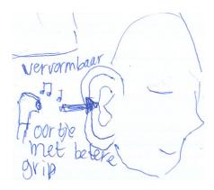
*Figure 4.6:* The magnetic field activates the magnetic soft material in the embodiment of earphones, to make the embodiment adjust to the shape of the ear of the user
