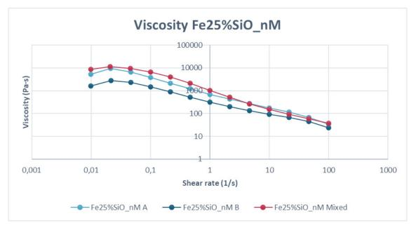
*Figure 3.10:* The viscosity of the Fe25%SiO\_nm ink from the sixth try of making ink recipes. There can be seen that the viscosity of component A is higher than that of component B. In this recipe, mixing order 2 is used.
