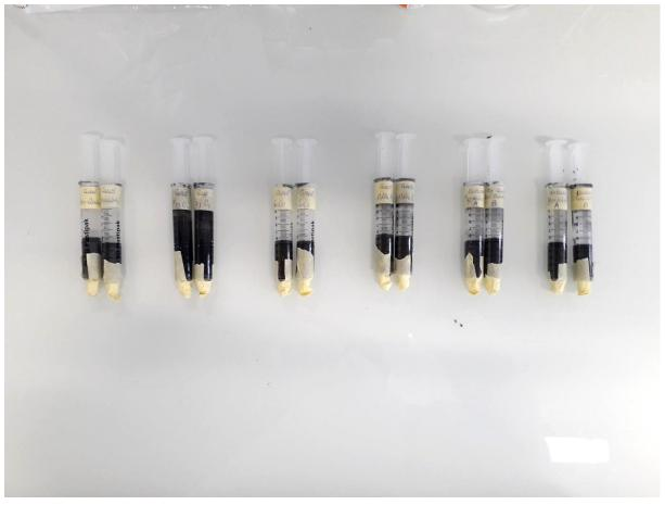
Figure 6 Magnetized ink samples in the syringes with the cut of tabs
