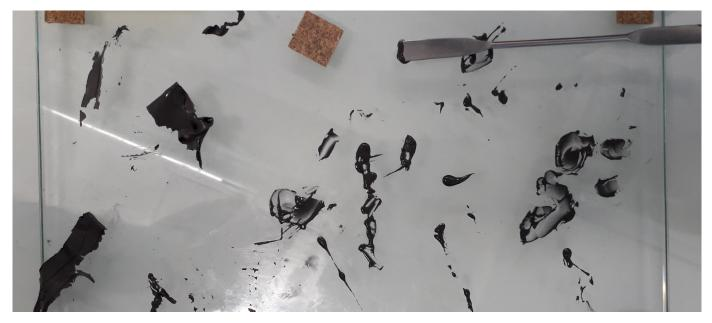
Figure 3.33: Ink out of the static mixing nozzle that after the curing time had not cured
