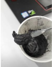
Figure 4 The smooth texture of the experiment with the 1:1 ratio between Ecoflex part A and B
