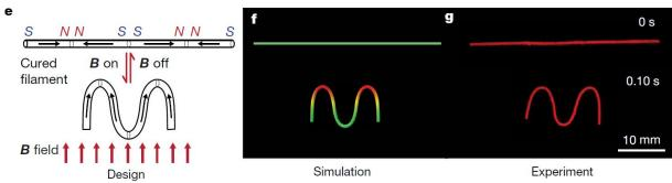
Figure 2 Magnetization pattern in one extruded rod
