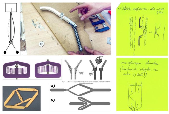
*Figure 4.12:* Collage of bistable mechanisms (Alqasimi, Lusk, & Chimento, 2016; Lichter, 1999; Technology, 2015; Wintergatan, 2018; Zirbel, Tolman, Brian P, & Howell, 2016)
