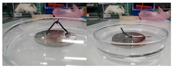
*Figure 3.45:* Working magnetic soft material. The disk magnet is turned around in the other picture, therefore once the middle is repelled and stands up in the left picture and in the picture on the right an end of the strips stands up.
